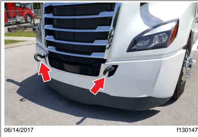
Fig. 13.3, Tow Hooks Installed, Facing Down
