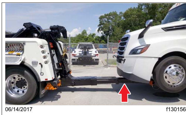
Fig. 13.12, Retracting the Recovery Boom
