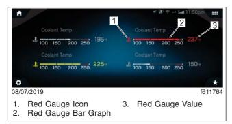
Fig. 3.57, Gauge Caution & Warning Indicator Display - ICC5
