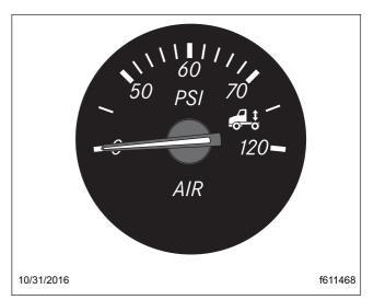
Fig. 3.44, Suspension Air Pressure Gauge
