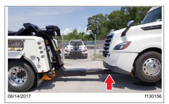
Fig. 26.13, Retracting the Recovery Boom
