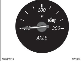
Fig. 3.38, Drive Axle Oil Temperature Gauge (rear drive axle gauge shown)
