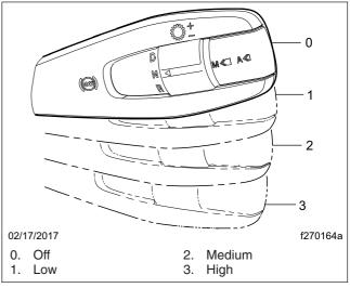
Fig. 4.14, Engine Brake Positions
