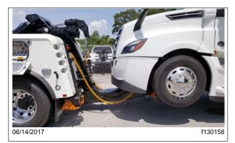
Fig. 26.15, Safety Chains Connected on the Towed Vehicle
