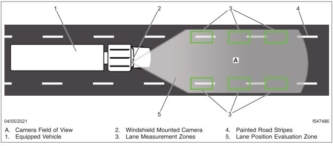
Fig. 7.27, Camera Field of View
