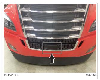
Fig. 5.1, Forward Radar Location
