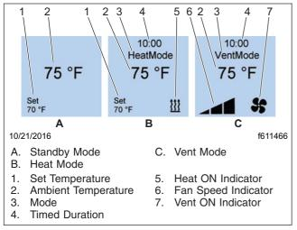
Fig. 8.10, Webasto Temperature Control Display Screens
