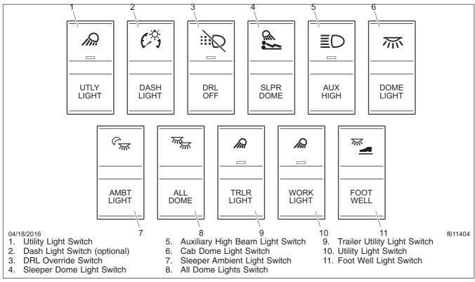
Fig. 4.3, Dash-Mounted and Sleeper-Control Light Switches
