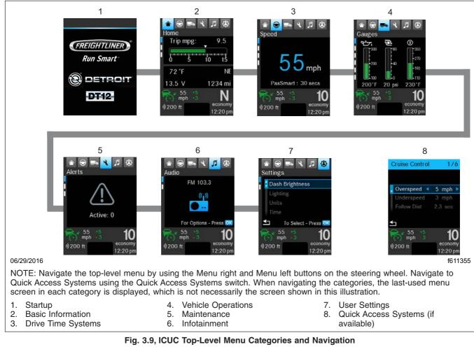
The Speed screen shows the current vehicle speed as well as temperature, odometer and PasSmart information. See **Fig. 3.9**
