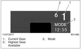
Fig. 17.11, Allison Gear Display in Automatic Mode
