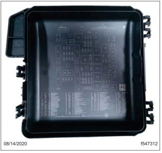
Fig. 11.7, VPDM Inside Cover Map of Fuses and Relays
