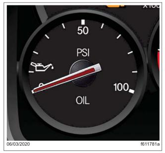
Fig. 3.39, Analog Engine Oil Pressure Gauge - ICUC
