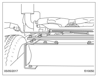
Fig. 20.12, Releasing the Sliding Fifth Wheel, (Fontaine)
