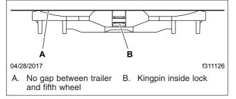
Fig. 20.5, Coupling Inspection
