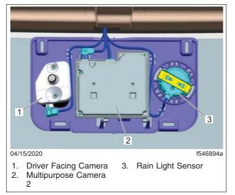
Fig. 6.1, Multipurpose Camera 2 Components
