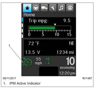
Fig. 7.20, IPM Active on the Driver Display - ICUC
