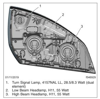
Fig. 22.5, Halogen Headlamp Assembly
