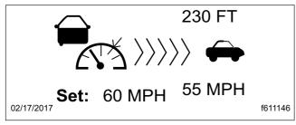
Fig. 7.33, ACC Lead Vehicle Detected (green)
