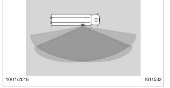
Fig. 6.11, Sensor Monitoring Area
