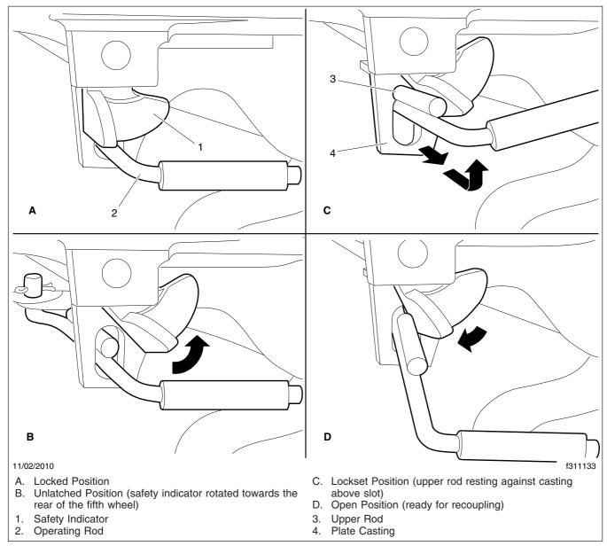
Fig. 20.8, Holland Kingpin Locking Mechanism
