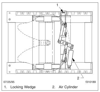
Fig. 20.15, Air-Operated Sliding Fifth Wheel (Fontaine shown)
