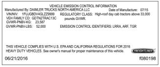
Fig. 1.13, Vehicle Emission Control Information Label
