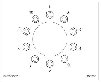
Fig. 25.4, Tightening Pattern, 10-Hole Wheels
