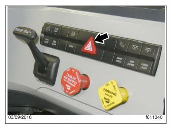
Fig. 26.1, Hazard Warning Switch
