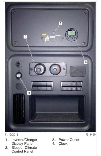
Fig. 10.6, Sleeper Control Panel
