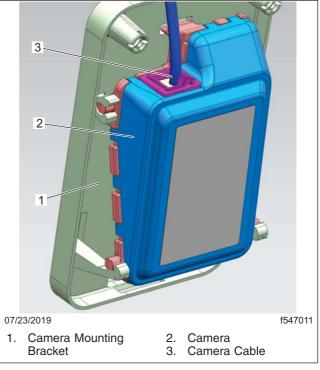
Fig. 5.2, Multipurpose Camera 1 Components
