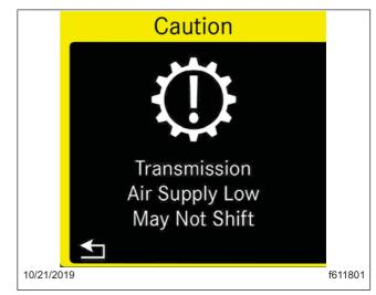
Fig. 17.8, Low Transmission Air Pressure Pop-up
