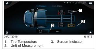
Fig. 3.63, TPMS: Tire Temperature- ICC5
