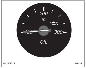
Fig. 3.40, Engine Oil Temperature Gauge
