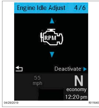
Fig. 3.21, Quick Access Screen: Engine Idle Adjust
