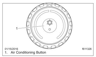
Fig. 8.3, Temperature Control Knob
