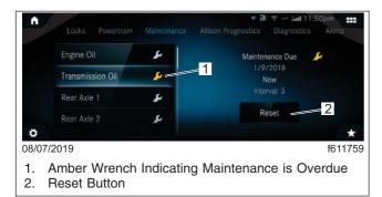
Fig. 3.65, Example ICC5 Maintenance Screen - ICC5
