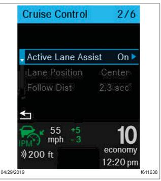
Fig. 3.19, Quick Access Screen: Cruise Control
