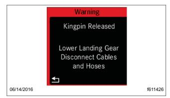
Fig. 20.10, Kingpin Release Alert Screen
