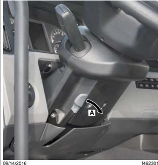
A. Pull the steering column locking lever out and away from the column.
