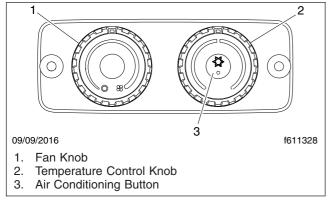
Fig. 8.5, Sleeper Climate Control Panel
