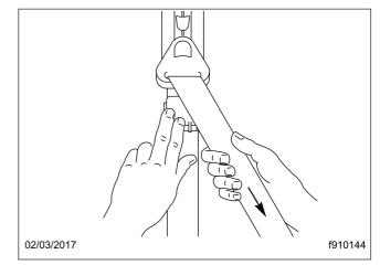
Fig. 9.11, Locking the Komfort Latch
