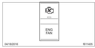
Fig. 4.15, Engine Fan Switch
