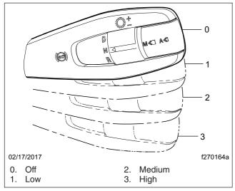
Fig. 17.2, Engine Brake Positions
