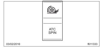
Fig. 15.3, ATC SPIN Switch
