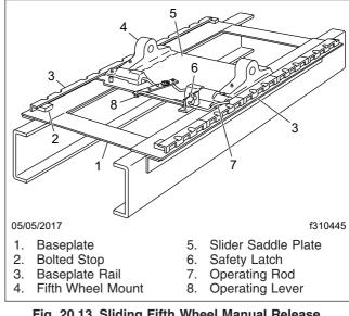
Fig. 20.13, Sliding Fifth Wheel Manual Release, (Holland Simplex)
