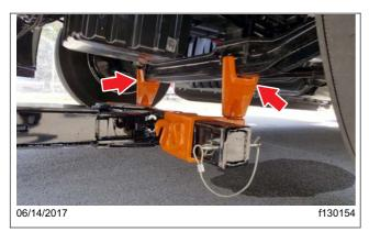
Fig. 26.11, Positioning the Stinger with Lift Adaptors Under the Axle
