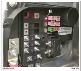
1. Cab Load Disconnect Switch Status LED
