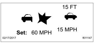
Fig. 7.34, ACC Collision Warning (red)
