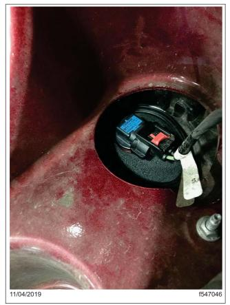
Fig. 22.9, Correct Halogen Headlamp Installation With Foam Grommet
