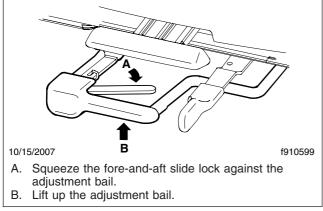
Fig. 9.5, Fore/Aft Slide Adjustment, Sears Atlas Seat
