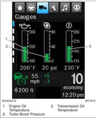
Fig. 3.23, Digital Oil and Pressure Gauges - ICUC
