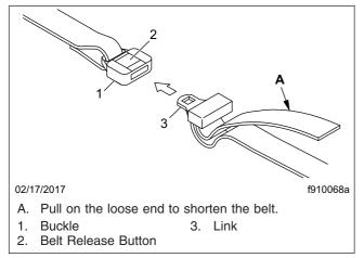
Fig. 9.12, Bunk Restraint Adjustment
