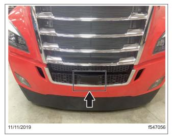
Fig. 6.2, Forward Radar Location
