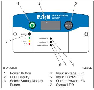
Fig. 11.13, Inverter/Charger Display Panel (Eaton)
