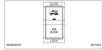
Fig. 4.29, Fifth Wheel Slide Control Switch
