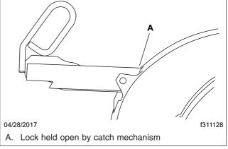
Fig. 20.6, Jost Release Handle Unlocked
