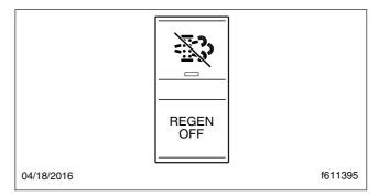
Fig. 4.12, Regen Inhibit Switch
