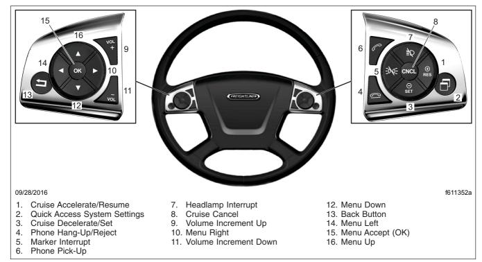
Fig. 5.4, Steering-Wheel-Mounted Switches
