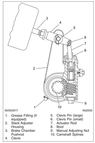
Fig. 25.3, Meritor Automatic Slack Adjuster
