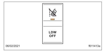
Fig. 7.25, AutoVue LDW OFF Switch
