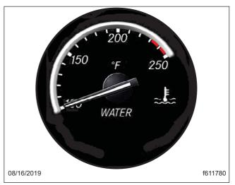
Fig. 3.37, Analog Coolant Temperature Gauge - ICUC
