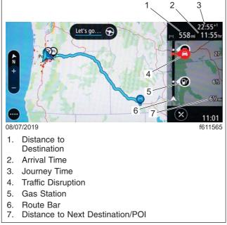
Fig. 7.13, Example of a Wide Route Bar - ICC5
