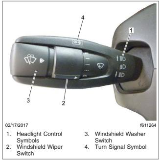
Fig. 4.5, Steering Column-Mounted Turn Signal Lever
