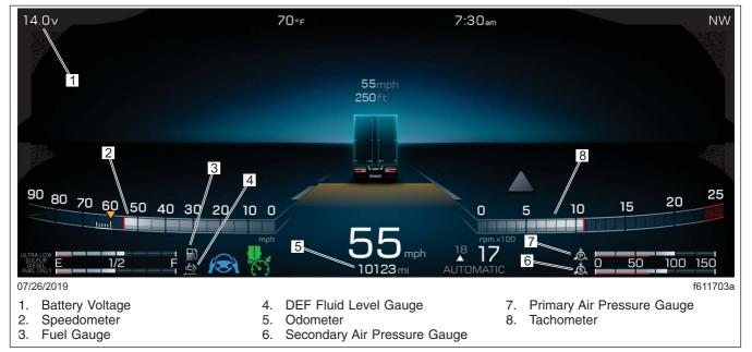
Fig. 3.58, Driver Display in Pilot Screen Mode - ICC5
