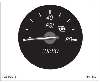
Fig. 3.47, Turbocharger Boost Pressure Gauge
