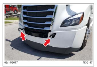
Fig. 26.5, Tow Hooks Installed, Facing Down
