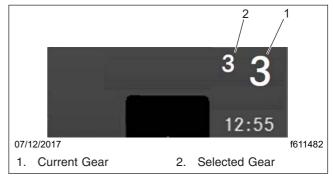
Fig. 17.12, Allison Gear Display in Manual Mode
