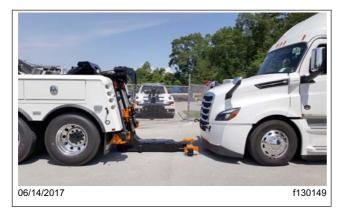
Fig. 26.6, Positioning the Stinger Assembly
