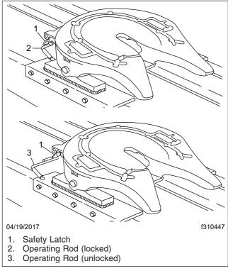
Fig. 20.2, Holland Simplex SE Locking Mechanism
