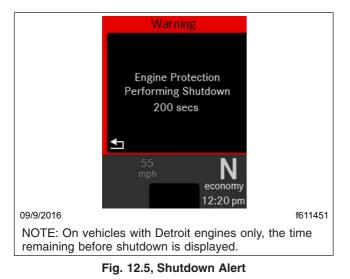
Do not operate the vehicle further until the problem causing the shutdown has been corrected.
