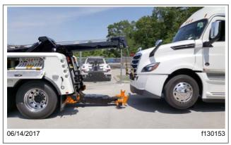
Fig. 26.10, Backing the Tow Truck with Lift Adaptors on the Crossbar
