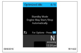
Fig. 13.4, Optimized Idle State Screen
