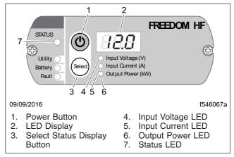
Fig. 11.12, Inverter/Charger Display Panel (Xantrex Freedom)
