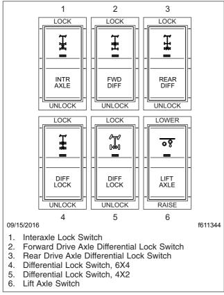
Fig. 4.13, Axle Switches
