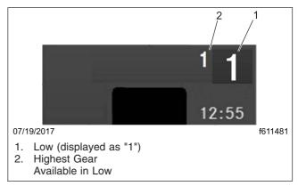
Fig. 17.13, Allison Gear Display in Low Gear
