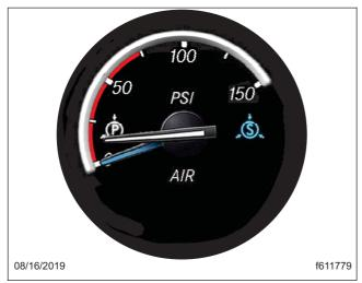
Fig. 3.42, Analog Combined Application Air Pressure Gauge - ICUC
