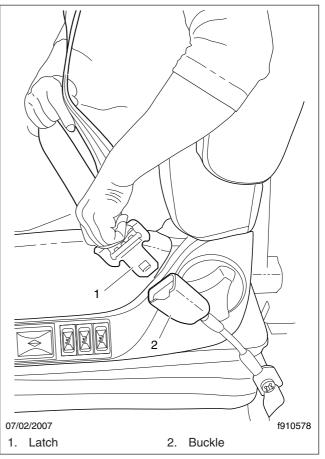
Fig. 9.8, Three-Point Seat Belt Operation
