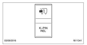
Fig. 20.9, Kingpin Release Switch
