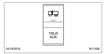
Fig. 4.30, Trailer Auxiliary Switch
