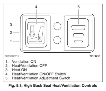
IMPORTANT: Turn off seat heating/ventilation when the seat is unoccupied.
