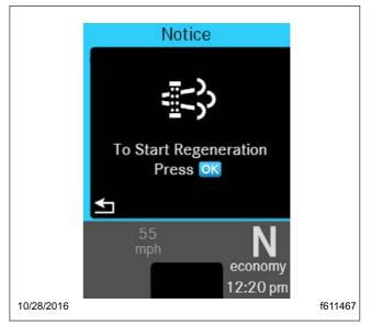
Fig. 4.11, Regen Start Digital Switch - ICUC
