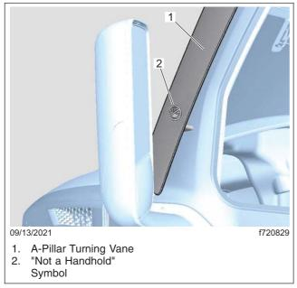
Fig. 2.9, A-Pillar Turning Vane
