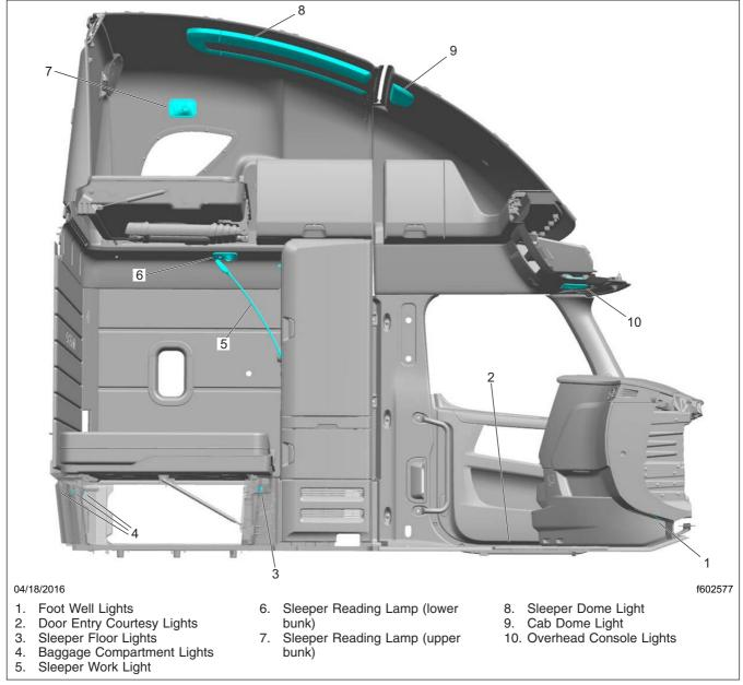
Fig. 4.9, Cab and Sleeper Interior Lighting
