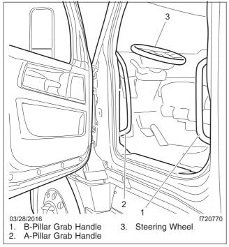
Fig. 2.4, Driver-Side Cab Access
