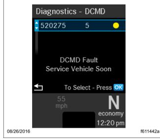
Fig. 11.3, Information Screen for an Active Fault Code
