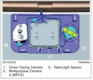
Fig. 4.23, MPC2 Cameras and Rain/Light Sensor
