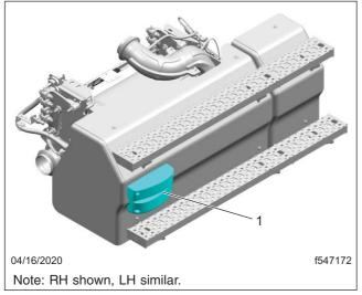
Fig. 6.10, Radar Sensors with Covers
