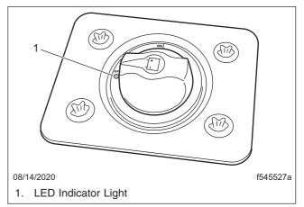
Fig. 11.9, Cab Load Disconnect Switch
