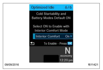
Fig. 13.3, Optimized Idle Mode Selection Screen
