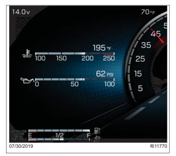
Fig. 3.60, Coolant Temperature & Engine Oil Pressure on Driver Display - ICC5
