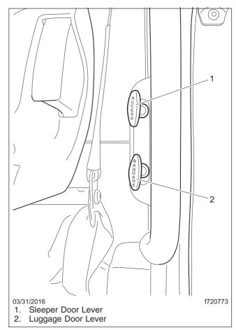
Fig. 2.7, Sleeper Door Levers
