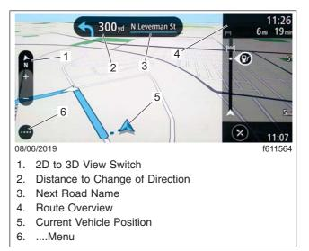
Fig. 7.12, Overview of 3D Display- ICC5
