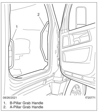
Fig. 2.5, Passenger-Side Cab Access
