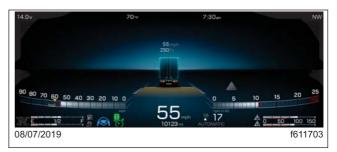
Fig. 3.50, Driver Display Pilot Screen - ICC5
