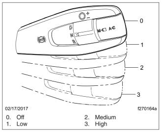
Fig. 15.5, Engine Brake Positions, Right-Hand Steering Column Lever
