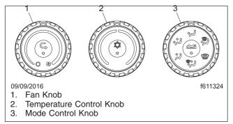
Fig. 8.1, Cab Climate Controls
