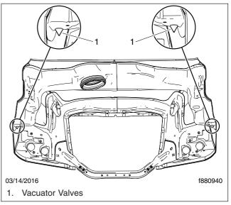
Fig. 25.11, Hood Vacuator Valves (hood interior shown)
