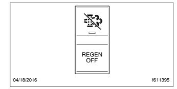
Fig. 14.3, Regen Inhibit Switch
