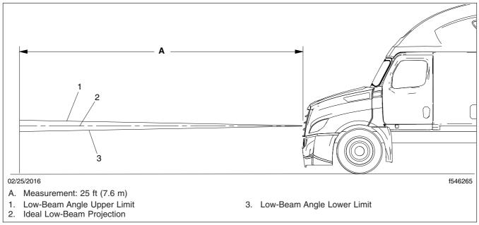
Fig. 22.3, Vertical Low-Beam Headlight Variation Limits
