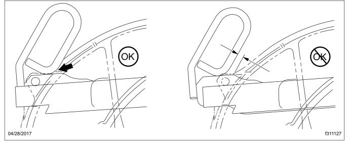
Fig. 20.7, Jost Release Handle Locked
