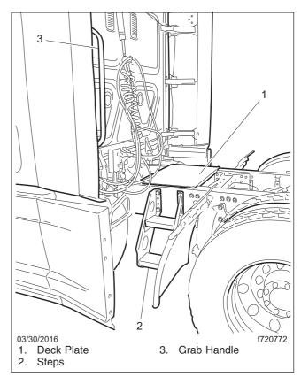
Fig. 2.8, Back-of-Cab Access
