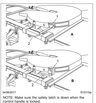
A. UnlockedB. Locked1. Safety Latch2. Lock Control Handle
