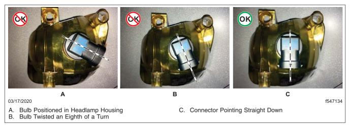
Fig. 22.8, Improper and Proper Bulb Installation, Back View
