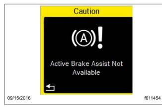
Fig. 6.7, Active Brake Assist (ABA) Alert - ICUC
