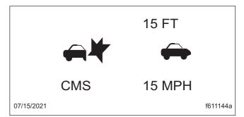
Fig. 7.31, CMS Collision Warning (red)
