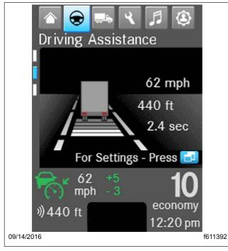
Fig. 5.3, Adaptive Cruise Control Screen
