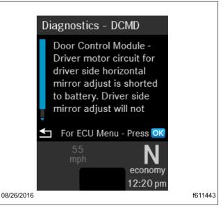
Fig. 11.4, Additional Information for the Fault
