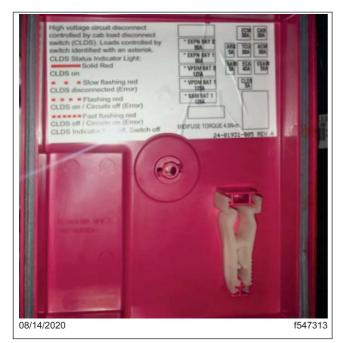
Fig. 11.6, Example Fuse Labeling on BCA Cover
