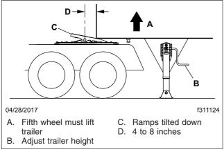
Fig. 20.3, Trailer Connection Point, Standard Fifth Wheel
