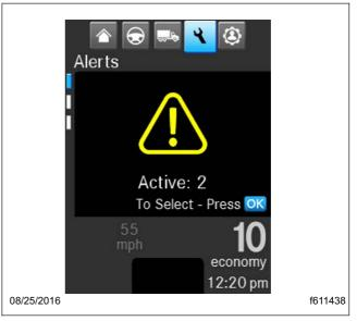
Fig. 11.1, ICUC Active Faults Alert Screen
