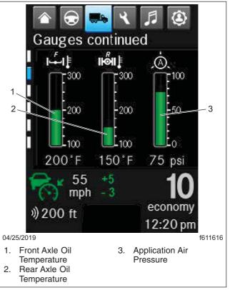
Fig. 3.24, Digital Oil and Pressure Gauges - ICUC
