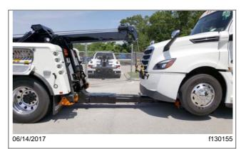
Fig. 26.12, Stinger with Lift Adaptors Under the Axle (tow truck shown)
