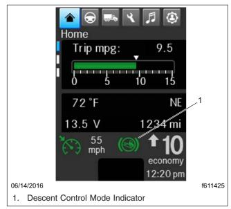
Fig. 7.22, Descent Control Mode on the Driver Display - ICUC
