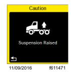
Fig. 3.29, Suspension Raised Alert - ICUC
