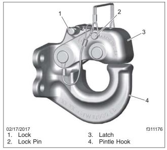
Fig. 21.2, Holland Trailer Coupling with Lock Pin
