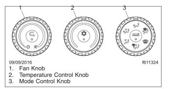
Fig. 4.33, Cab Climate Controls
