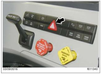
Fig. 4.4, Hazard Warning Switch
