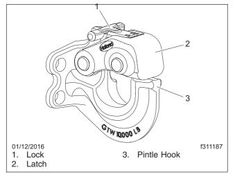
Fig. 21.1, Holland Trailer Coupling with FastLatch
