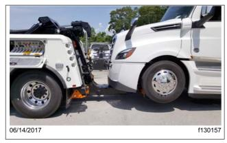
Fig. 26.14, Final Towing Position
