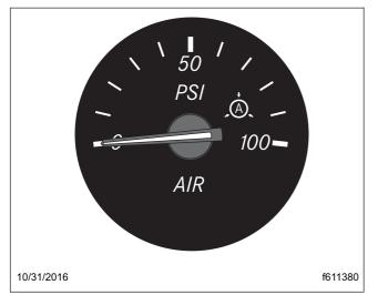
Fig. 3.36, Application Air Pressure Gauge
