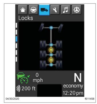
Fig. 19.1, Interaxle and Differential Locks Status Screen
