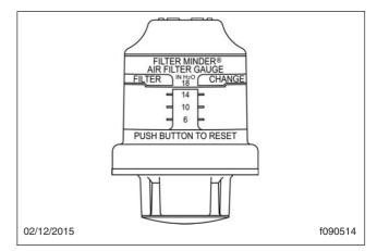
Fig. 3.35, Air Intake Restriction Indicator, Graduated
