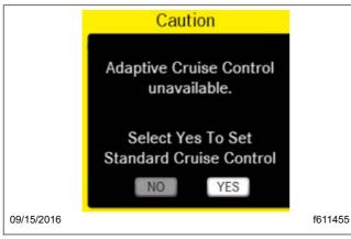
Fig. 6.5, Adaptive Cruise Control (ACC) Unavailable - ICUC
