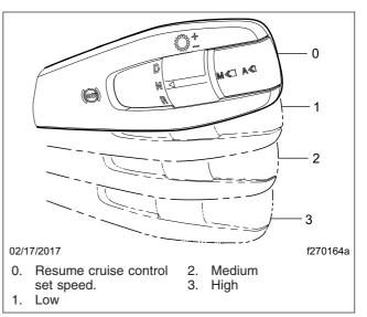
Fig. 7.23, Deceleration Mode Positions, Automated/ Automatic Transmission Multifunction Control
