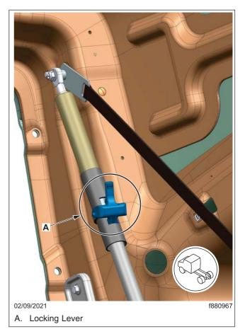
Fig. 2.10, Locking Right-Hand Hood Strut
