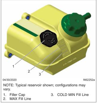
Fig. 25.5, Power Steering Fluid Reservoir
