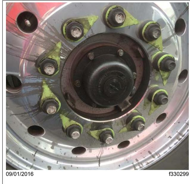
**Fig. 9, Excessive Leakage**
