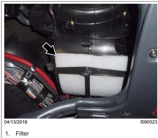
**Fig. 4, Cab Recirculation Air Filter**
