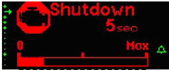
Engine Protection Shutdown Timer
