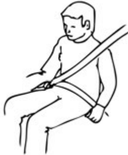
Incorrect (too high on hips)
