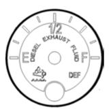
The diesel exhaust fluid gauge shows the approximate amount of DEF fluid in the DEF tank. Besides empty and full, the gauge also indicates 1/4, 1/2, and 3/4 of total capacity. DEF fluid is required to meet certain emission requirements. Maintain an adequate amount of diesel exhaust fluid at all times, as provided in the aftertreatment system operator manual. Please refer to the aftertreatment operator manual for more details about DEF fluid.
