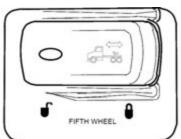
Vehicles having an air slide fifth wheel have a fifth wheel slider lock controlled by a switch on the instrument panel. By placing the switch in the unlock position, you can slide the fifth wheel to various positions to adjust weight distribution. There is a guard over this switch to protect you against accidentally activating or releasing the lock.
