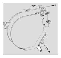
Using a 27 mm socket wrench (DIN3124), remove the filter cap that is screwed to the DEF Supply pump.
