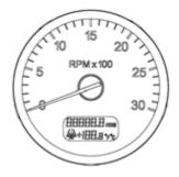
Watching your tachometer is important to driving efficiently. It will let you match driving speed and gear selection to the operating range of your engine. If your engine speed gets too high, you can select a higher gear to lower the RPM. If your engine speed drops
