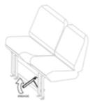
Apply the parking brake. Pull upward on the parking brake lever
