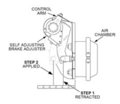
Brake Chamber Stroke
