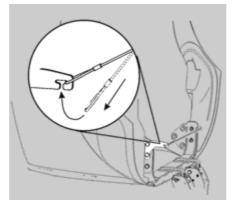
Safety cable in its attached position
