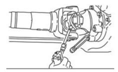
The slip joints and universal joints of the drive shaft should be lubricated according to Preventive Maintenance Schedule on page 5-12.
