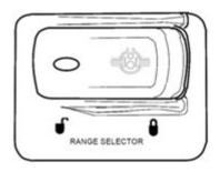
If your vehicle is equipped with a two-speed rear axle, you can select the axle range by the dash mounted switch shown above. The low range provides maximum torque for operating off-highway. The high range is a faster ratio for highway speeds.
