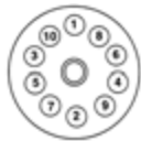
Nut Tightening Sequence for Hub Piloted Disc Wheels
