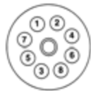
Nut Tightening Sequence for Hub Piloted Disc Wheels
