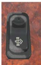
Figure 26 Regen Request Switch
