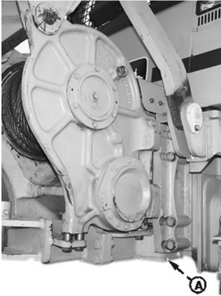
Winch Oil Filter Location
