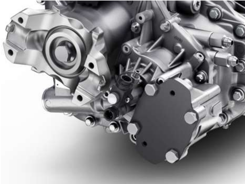
Figure 2: Rear DT12 PTO drive assembly (option 362-2HB) with cover plate.
