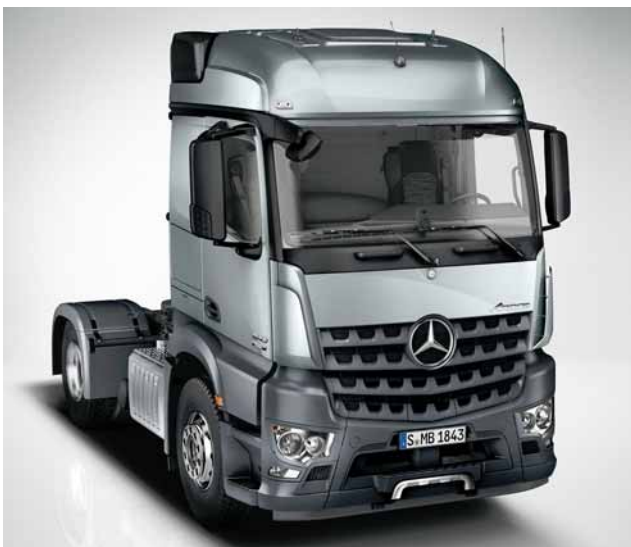
StreamSpace L cab, body floor height 600 mm
