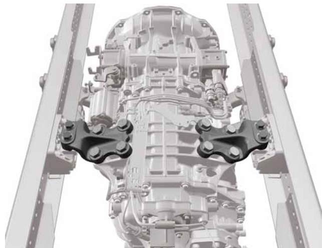
Transmission with bolted support arms
