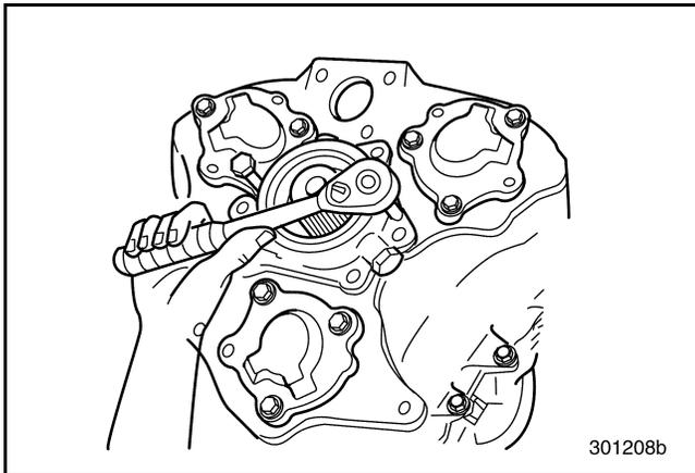
**Figure 83 — Removing Rear Mainshaft Bearing Cover Using Jackscrews**
