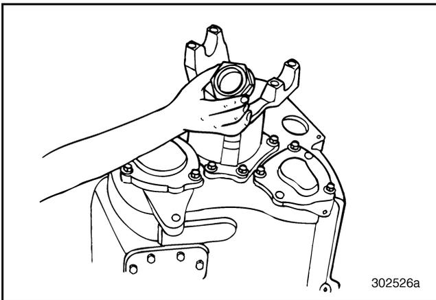
**Figure 566 — Installing Drive Yoke and Nut (T313L21/T318L21 Shown)**
