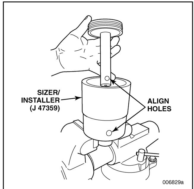
**Figure 457 — Aligning Shift Fork Locking Bolt Hole with Air Fitting Port in Cylinder Housing**
