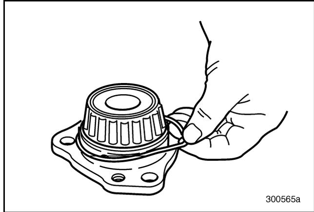
Figure 275 — Removing O-Ring from Shoulder of Front Countershaft Front Bearing Cover
