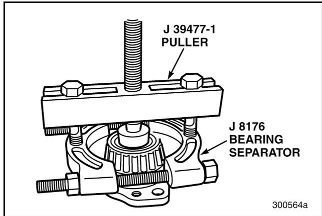
Figure 276 — Removing Bearing Cone from Front Countershaft Front Bearing Cover
