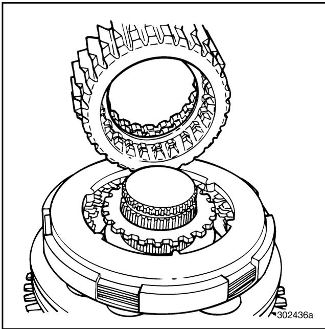
**Figure 392 — Installing Hi-Range/Hi-Split Gear (T313L21/T318L21 Shown)**
