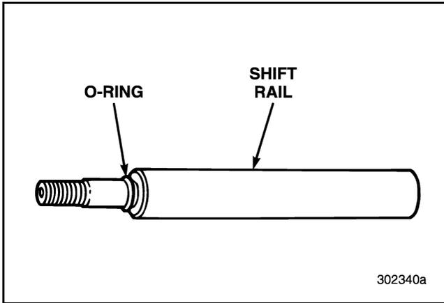
Figure 176 — Removing Shift Rail O-Ring
