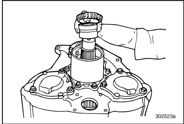
**Figure 563 — Installing Spacer and Outer Bearing Cone (T313L21/T318L21 Shown)**
