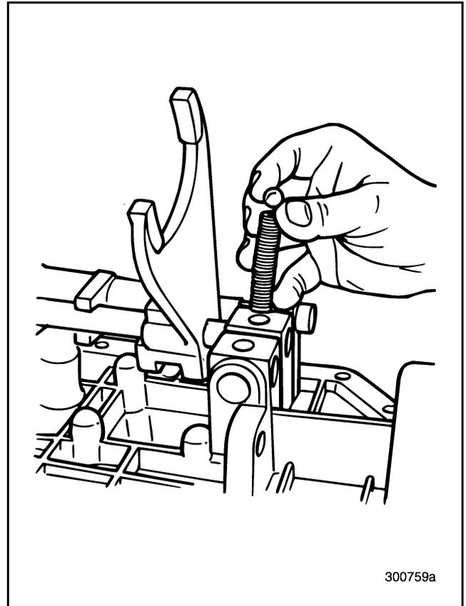
Figure 143 — Removing Poppet Ball and Spring
