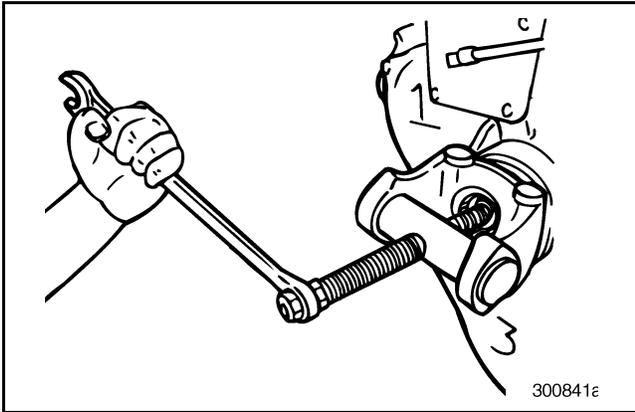
Figure 70 — Removing Drive Yoke (T313L/T318L Shown)
