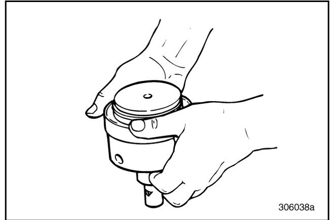
Figure 181 — Piston Assembly Partially Removed
