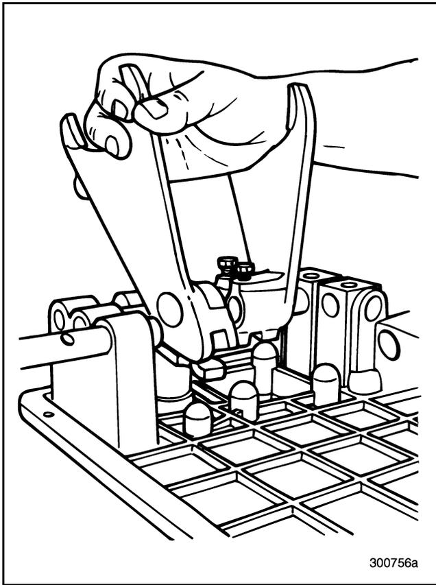
Figure 498 — Installing Third/Fourth Shift Fork
