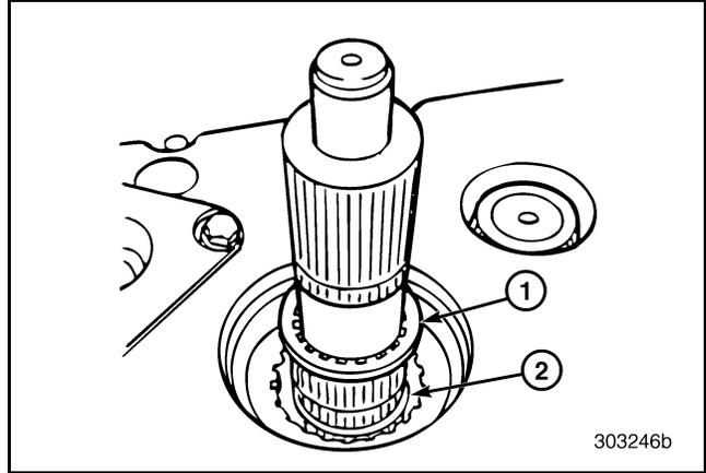
**Figure 108 — Removing Internal-Toothed Thrust Washer and Snap Ring (T313L/T318L Shown)**
