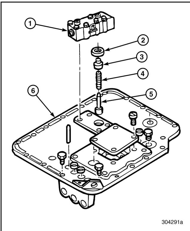
**Figure 63 — Removing Range Shift Valve**
