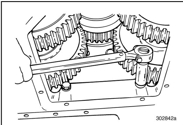
Figure 556 — Tightening Inner Case-to-Case Capscrews
