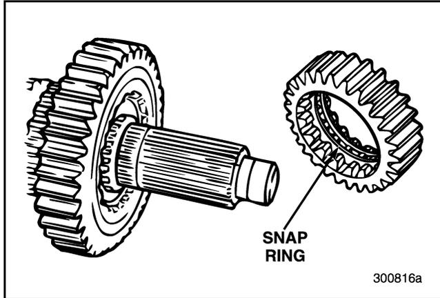
Figure 217 — Removing Fourth Speed Gear
