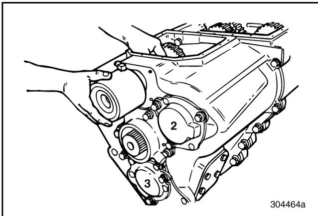
Figure 75 — Removing Range Shift Cylinder
