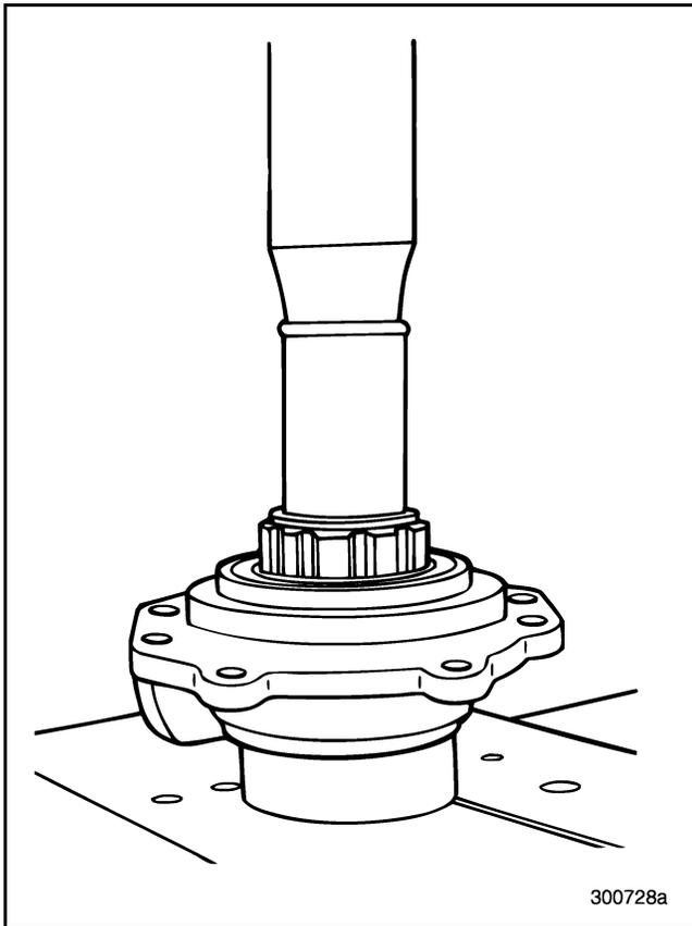
Figure 431 — Installing Main Drive Pinion Assembly into Drive Pinion Bearing Cover
