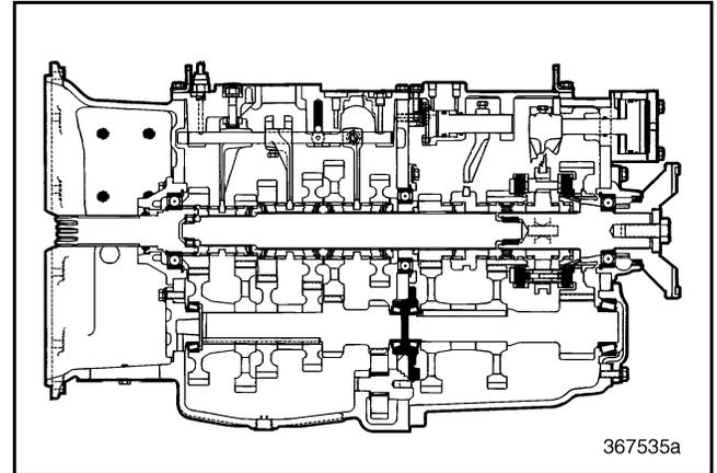
Figure 320 — Front Countershaft Rear Bearing Cover Component Locator (T313L/T318L Shown)
