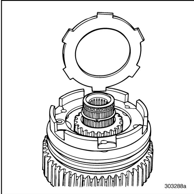
**Figure 379 — Installing Reaction Disc
