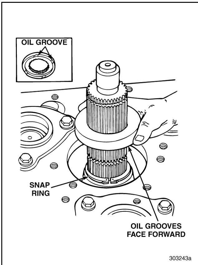
Figure 535 — Installing Bearing Spacer (T313LR/T318LR Shown)
