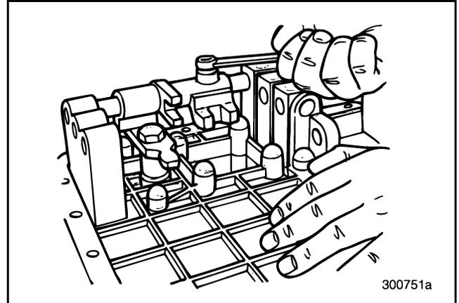
Figure 148 — Removing Setscrew from Third/Fourth Shifter
