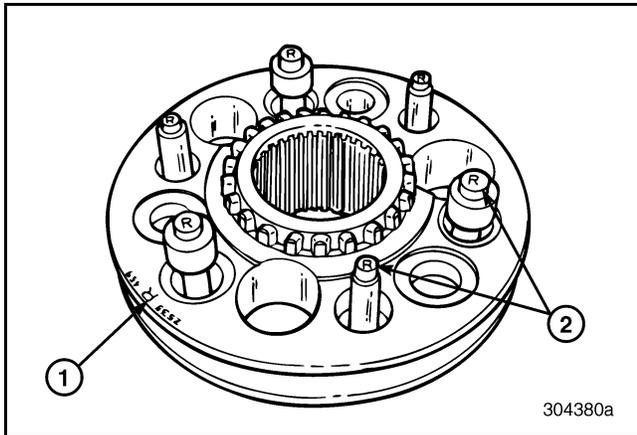
**Figure 263 — Letter “R” on Sliding Clutch and Synchronizer Pins**
