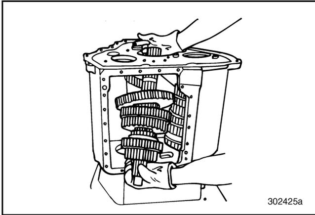
Figure 122 — Removing the Mainshaft
