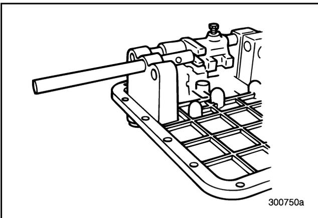
Figure 147 — Removing First/Second Shift Rail
