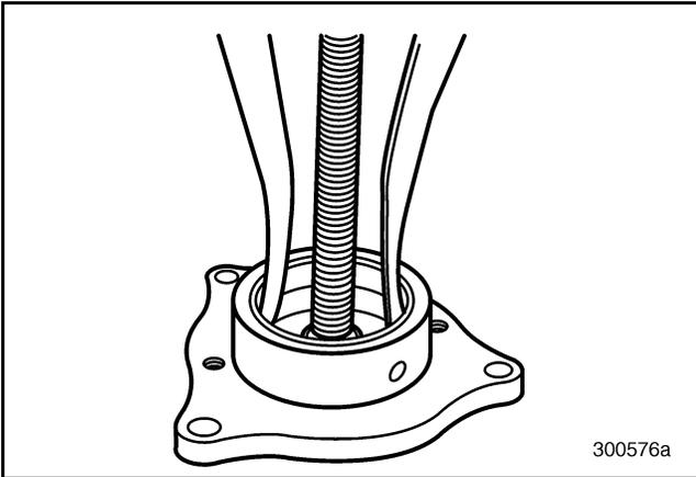
Figure 297 — Removing Bearing Cup from Cover
