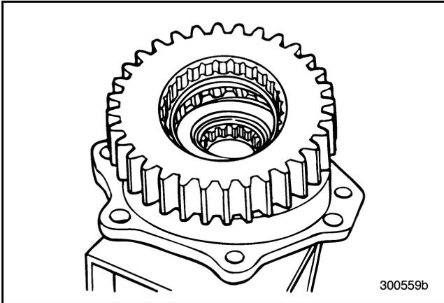
Figure 193 — Removing Main Drive Pinion Gear
