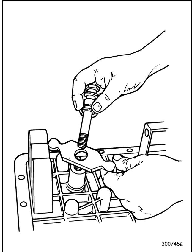
Figure 481 — Installing Third/Fourth Rocker Pin and
