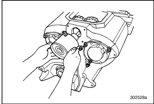
**Figure 570 — Installing Range Shift Cylinder**
