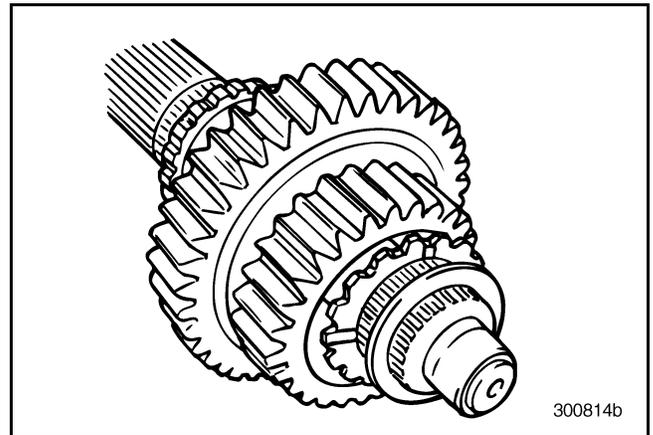
**Figure 216 — Removing Internal- and External-Toothed Thrust Washers at Fourth Speed Gear**
