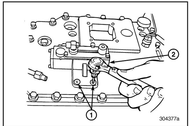
Figure 579 — Tightening Range Shift Interlock Valve Screws
