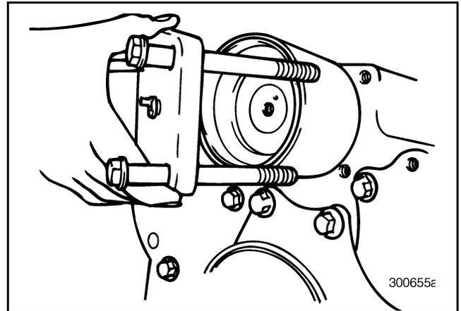
Figure 73 — Removing Range Shift Cylinder Cover
