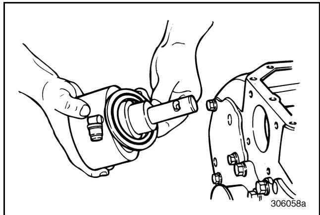
**Figure 571 — Installing Shift Cylinder Gasket**
