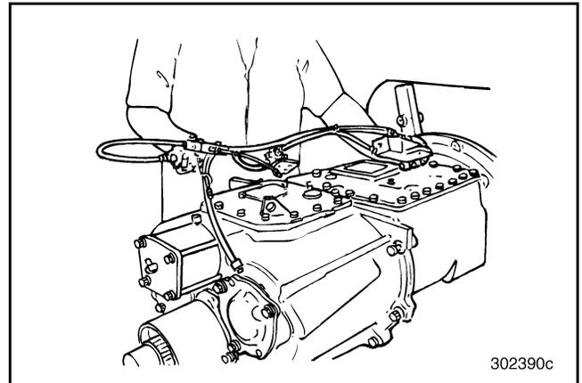
**Figure 64 — Removing Air Lines and Valves**
