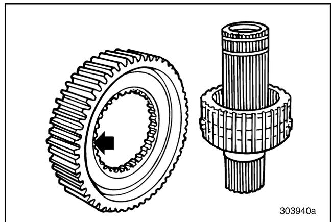
Figure 255 — Removing Lo-Range Gear from Hub (T313L/T318L Shown)
