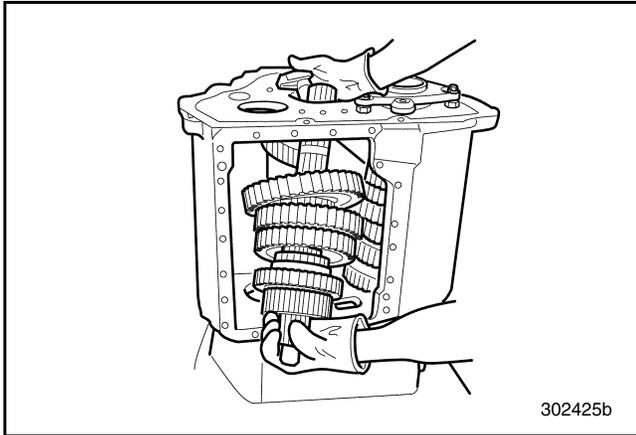
Figure 522 — Installing Mainshaft into Case
