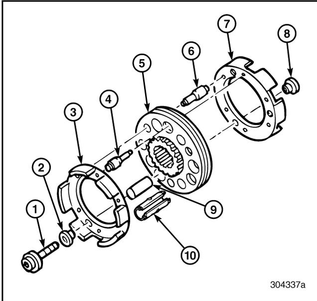
Figure 260 — Exploded View of Synchronizer
