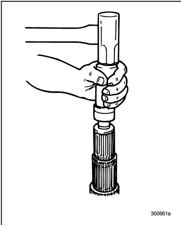
Figure 400 — Installing Spigot Bearing Inner Race
