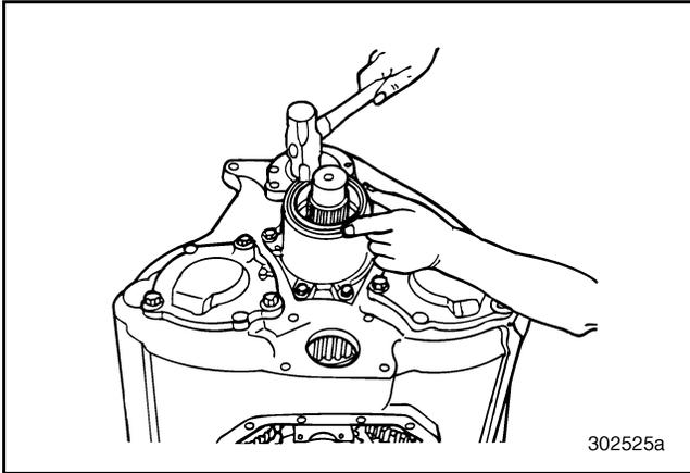
**Figure 565 — Installing Output Housing Oil Seal (T313L21/T318L21 Shown)**
