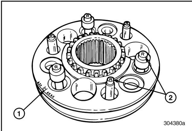
**Figure 359 — Synchronizer Pins and Sliding Clutch Temporarily Assembled to Show "R" Marks**
