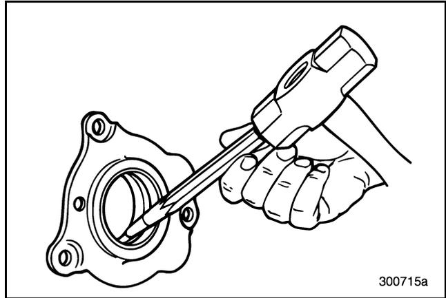
Figure 287 — Removing Front Bearing Cup
