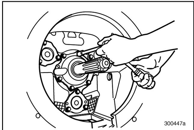
**Figure 109 — Removing Pinion Bearing Cover Capscrews**
