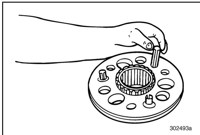
**Figure 362 — Installing Preload Springs into Sliding Clutch**
