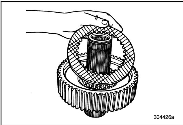
Figure 376 — Installing Friction Disc
