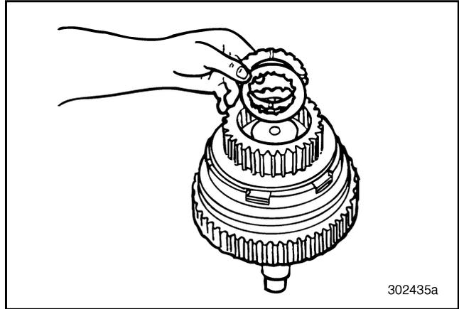
**Figure 393 — Installing Thrust Washers (T313L21/T318L21 Shown)**
