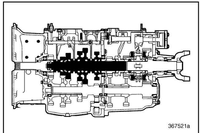
Figure 397 — Front Mainshaft Component Locator
