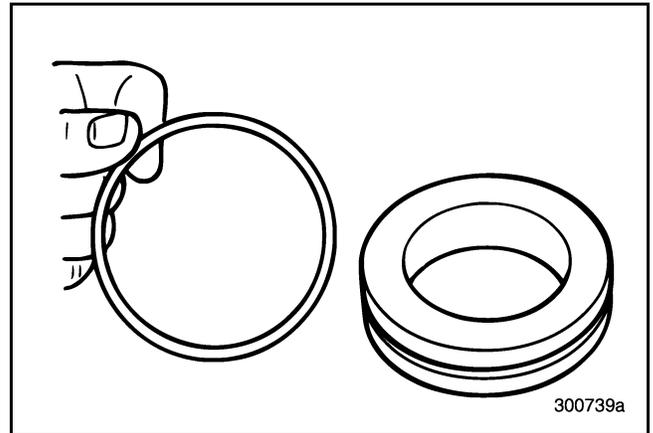
Figure 462 — Installing Piston Sleeve O-Ring
