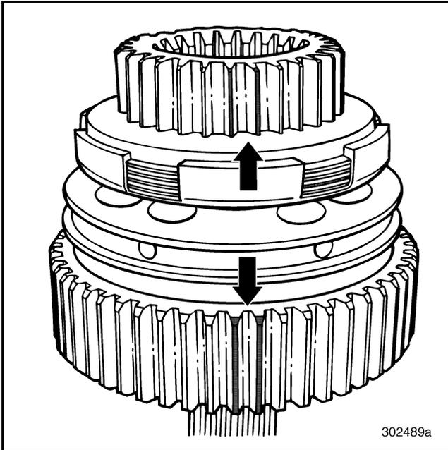
Figure 395 — Painting Timing Marks on Gears
