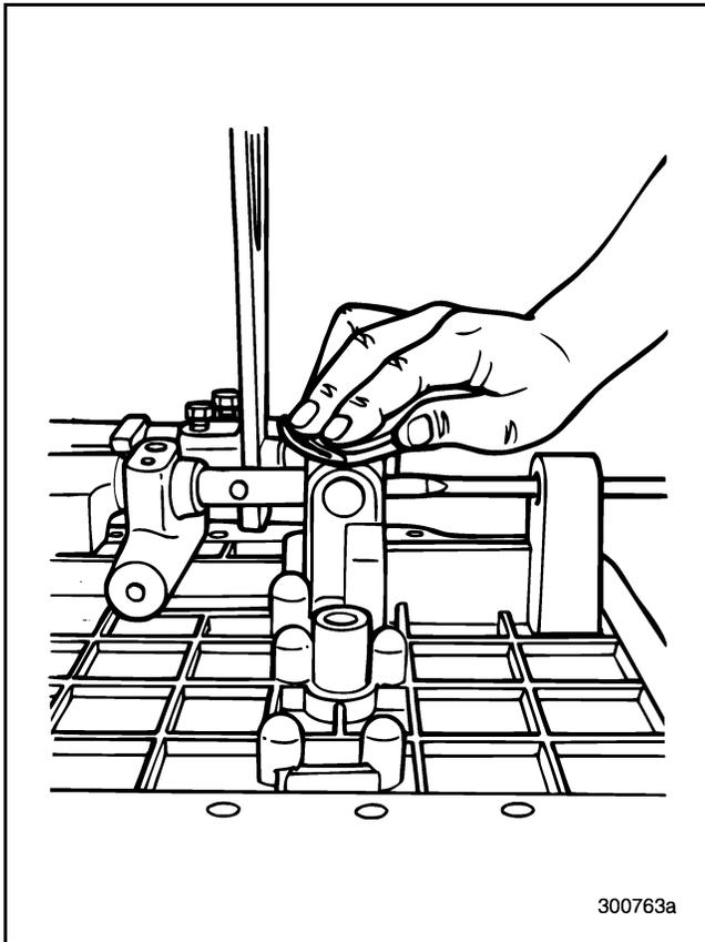
**Figure 136 — Pushing Lo/Reverse Shift Rail Forward**
