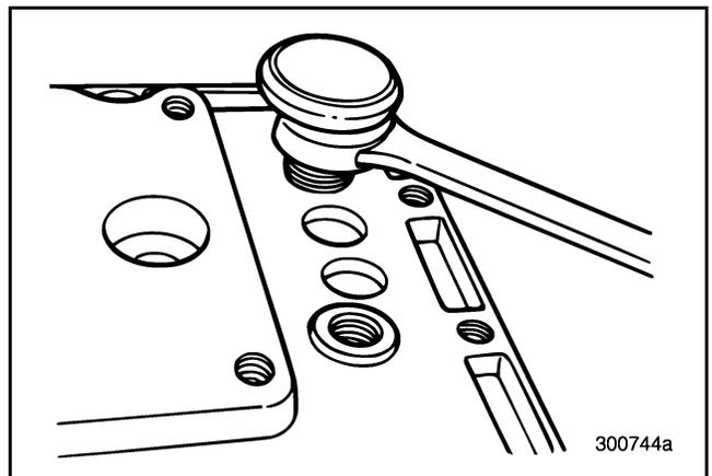
Figure 158 — Removing Breather Vent
