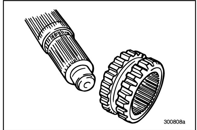
**Figure 223 — Removing First/Second Sliding Clutch**
