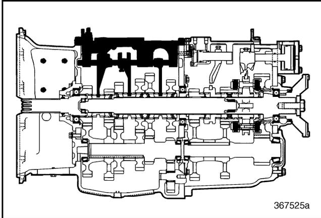
Figure 479 — Main Case Shift Cover Locator
