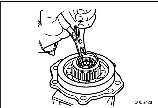
Figure 194 — Removing Spigot Bearing Snap Ring
