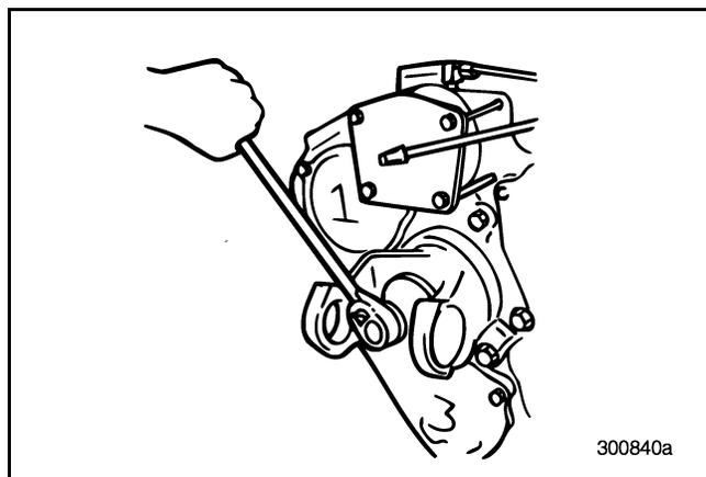
Figure 69 — Removing Clamp Plate and Capscrew (T313L/T318L Shown)
