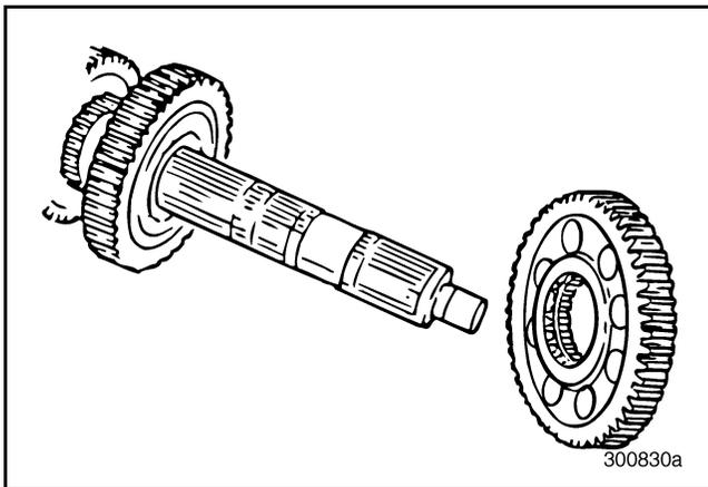
**Figure 418 — Installing Lo-Speed Gear (T313L/T318L Shown)**
