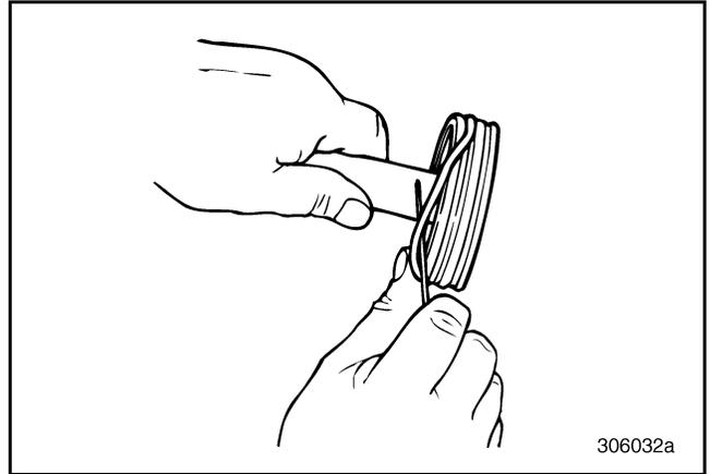
Figure 450 — Installing O-Ring in Second/Lower Groove on Piston
