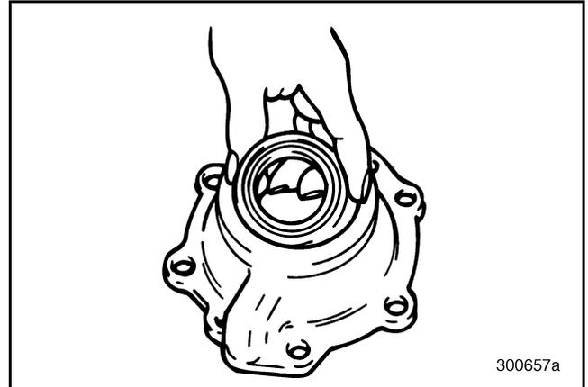
Figure 429 — Positioning Bearing Cover Oil Seal
