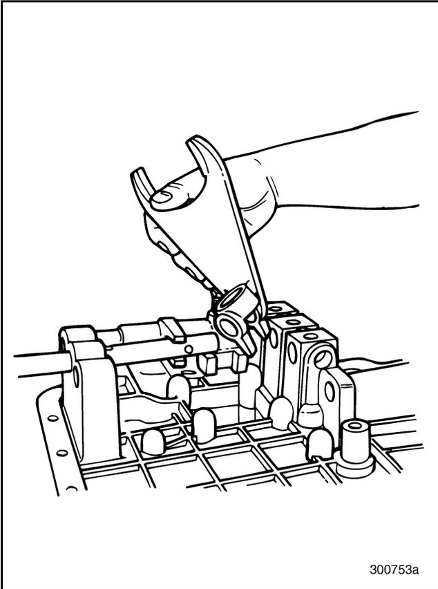
Figure 146 — Removing First/Second Shift Fork
