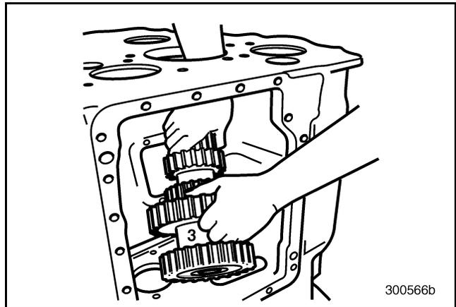
Figure 124 — Removing No. 3 Lower Countershaft
