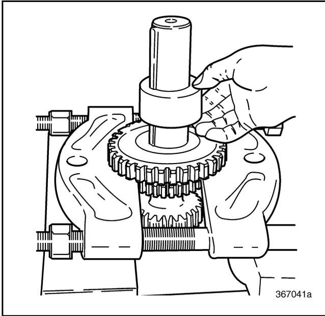
**Figure 280 — Removing First/Second Gear Spacer**
