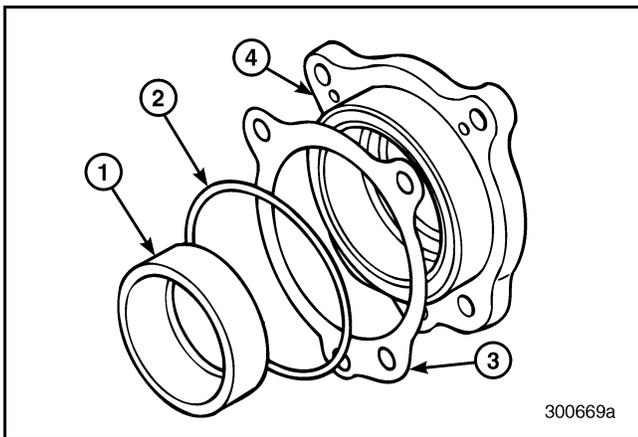
**Figure 607 — Exploded View of Rear Countershaft Bearing Cover**
