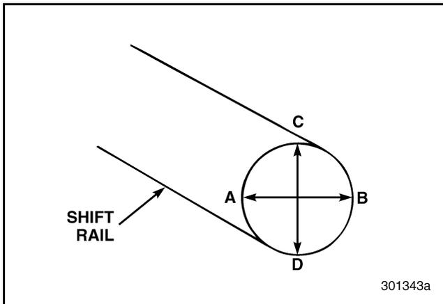
Figure 302 — Measuring Shift Rail
