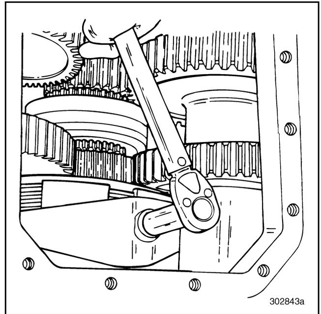
**Figure 573 — Tightening Shift Fork Setscrew**
