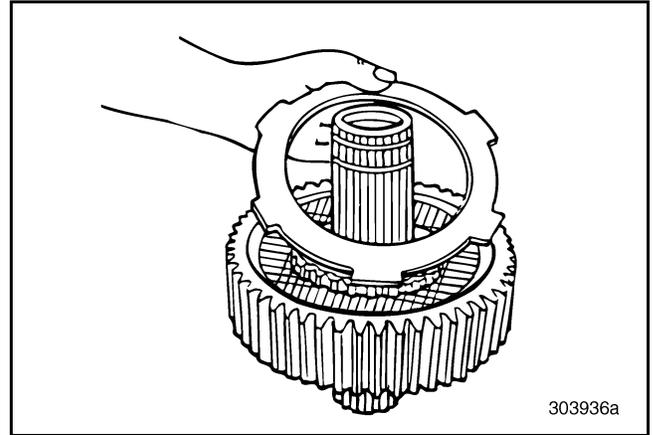
**Figure 250 — Removing Reaction Disc (T313L/T318L Shown)**
