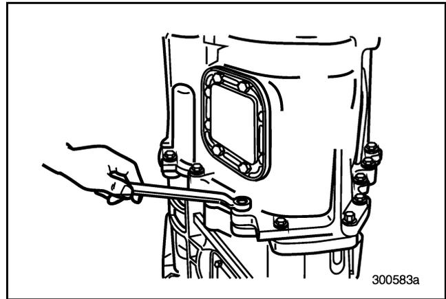
Figure 92 — Removing Inner Rear Case-to-Main Case Capscrews
