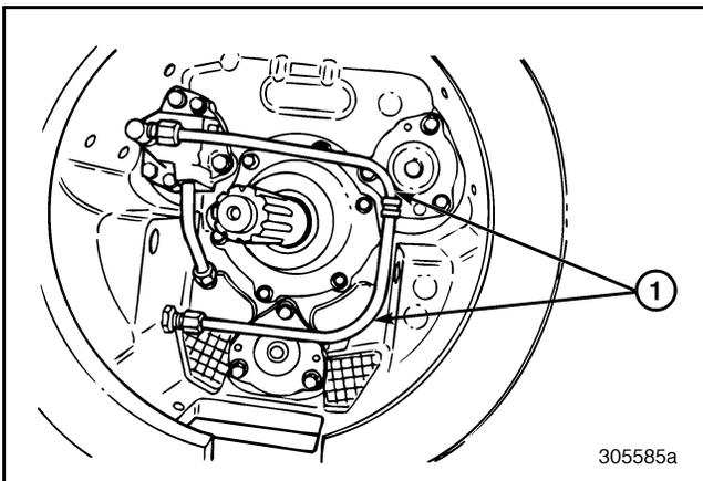
**Figure 111 — Oil Pump Discharge Line (if Equipped)**
