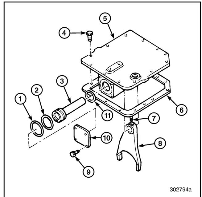
Figure 472 — Exploded View of Rear Case Shift Cover
