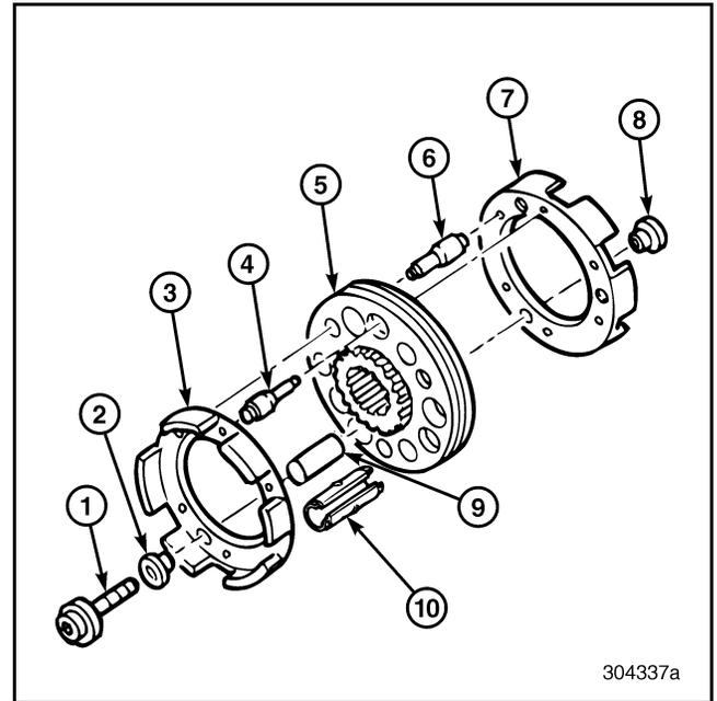
Figure 356 — Exploded View of Synchronizer
