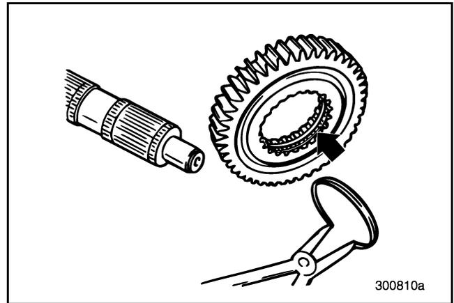
Figure 415 — Installing Snap Ring into First Speed Gear (T313L/T318L Shown)
