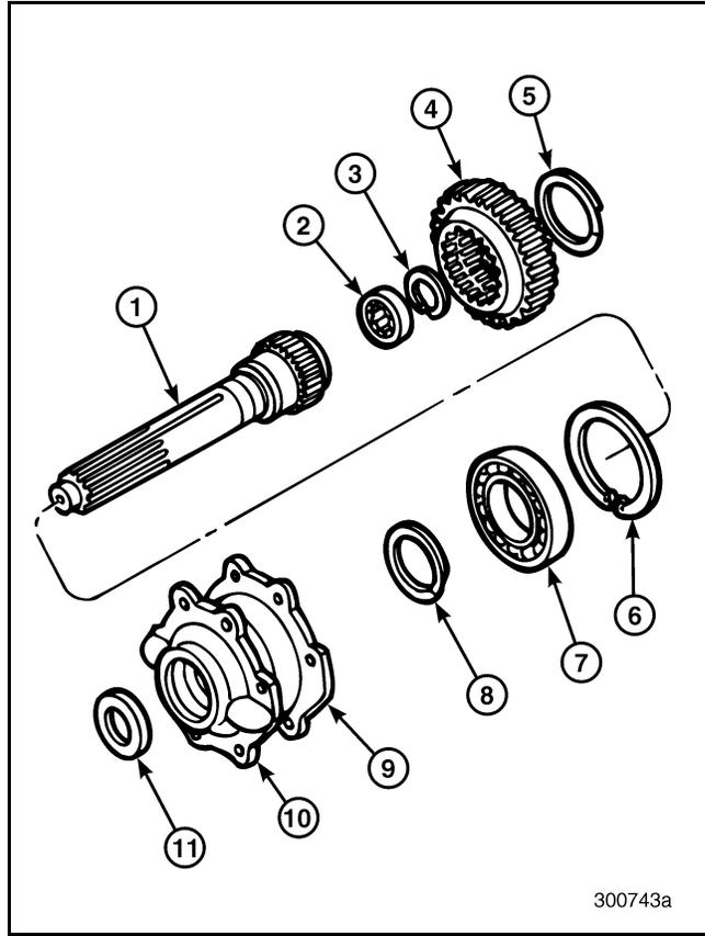
Figure 426 — Exploded View of Main Drive Pinion
