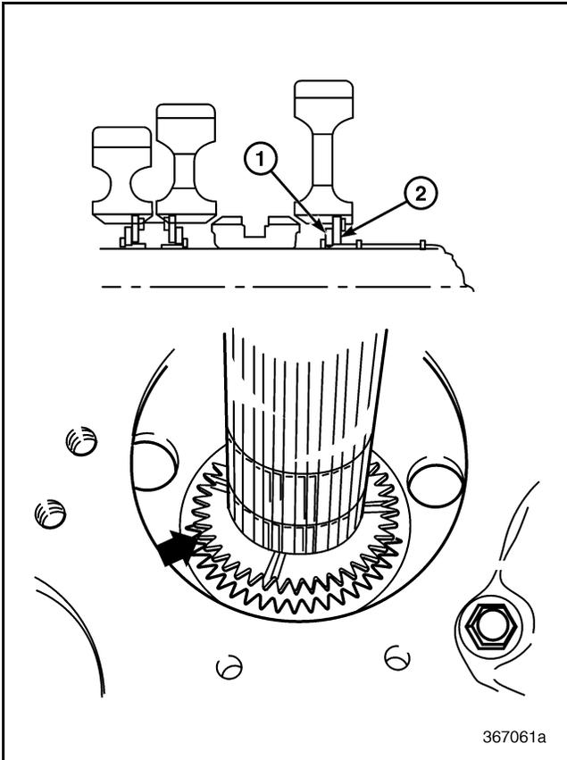
Figure 530 — Installing Internal-Toothed Thrust Washer
