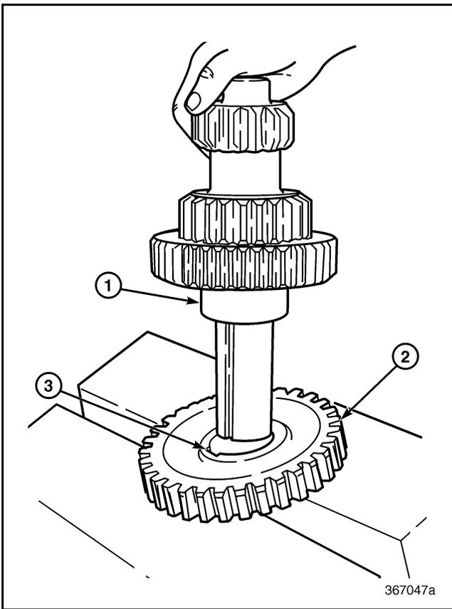
Figure 330 — Aligning Keyway with Second (Sixth) Gear
