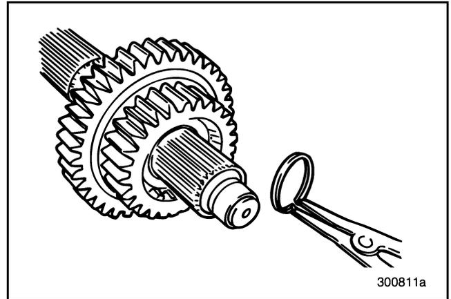
**Figure 215 — Removing Fourth Speed Gear Snap Ring**
