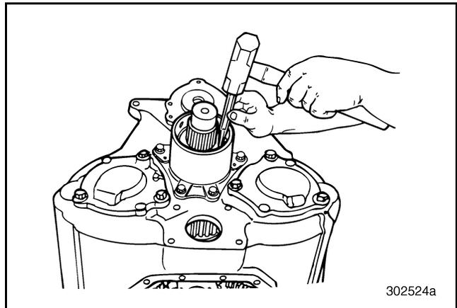
**Figure 564 — Seating the Bearing Cone and Spacer (T313L21/T318L21 Shown)**
