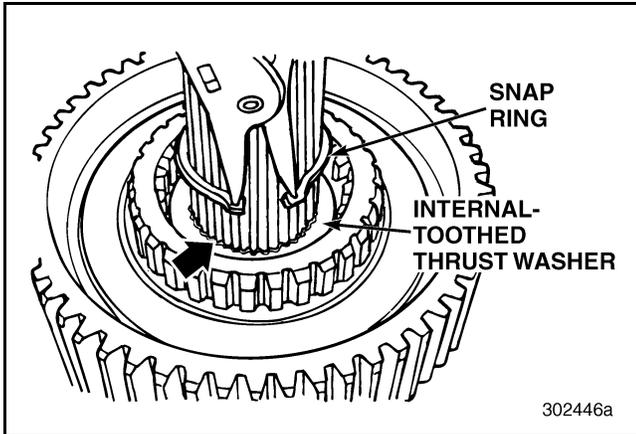
Figure 252 — Removing Shaft Snap Ring
