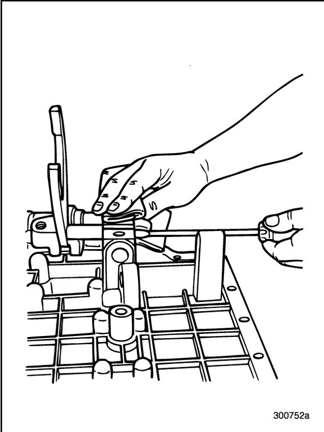
Figure 142 — Pushing First/Second Shift Rail Forward
