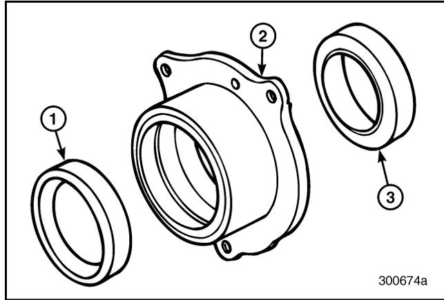
**Figure 608 — Exploded View of Front Countershaft Rear Bearing Cover**
