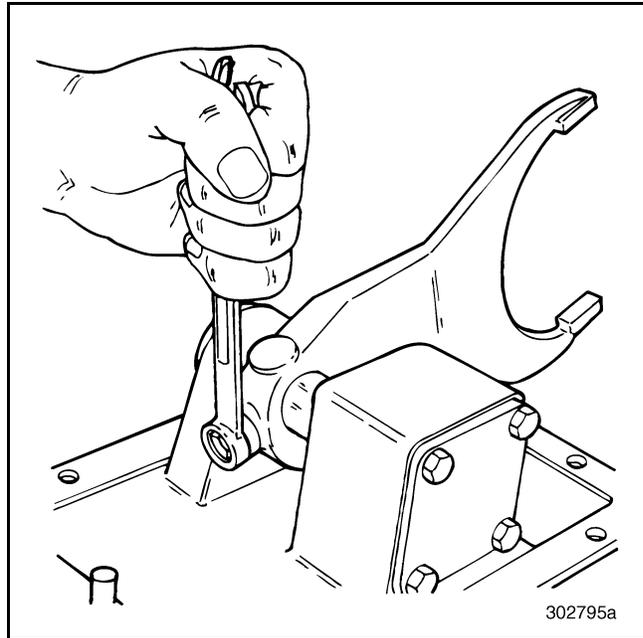
Figure 161 — Removing Setscrew
