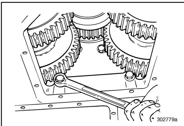
Figure 91 — Removing Outer Rear Case-to-Main Case Capscrews
