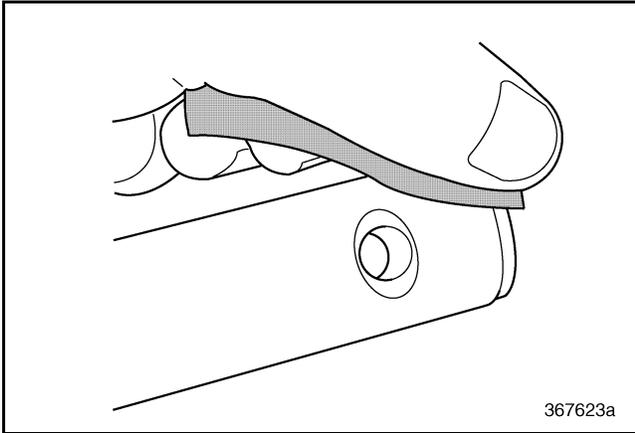
**Figure 455 — Polishing Shift Rail and Setscrew Hole with Crocus Cloth**
