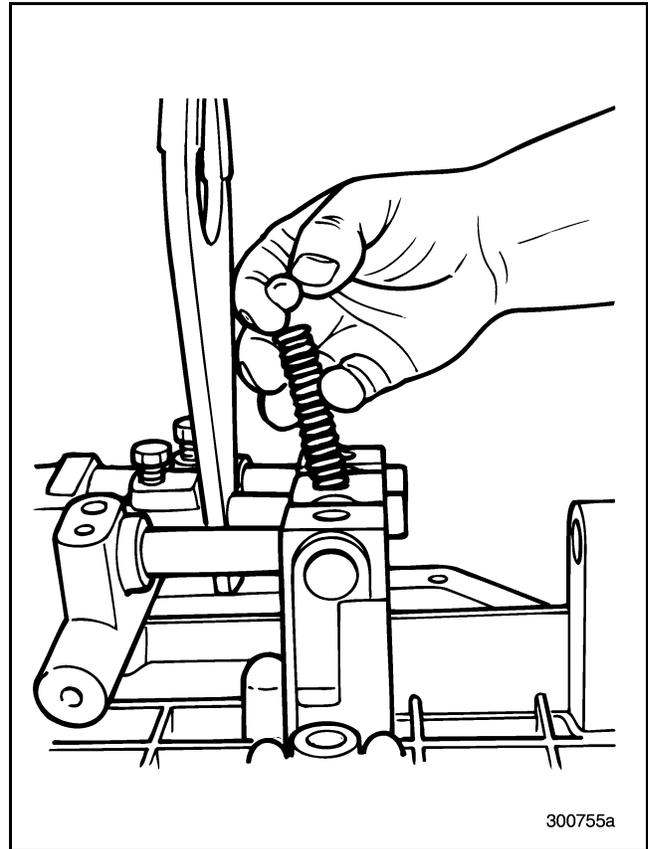
**Figure 137 — Removing Poppet Ball and Spring**
