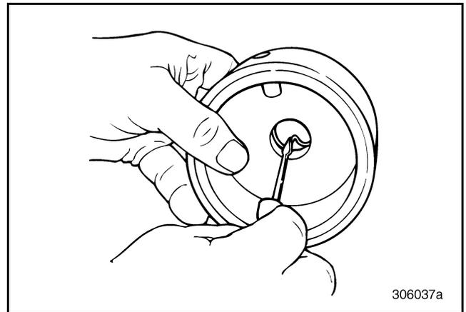
Figure 182 — Removing Teflon® Seal and O-Ring Expander
