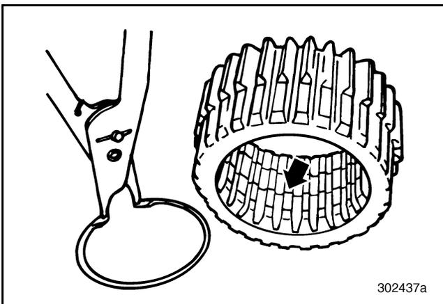
Figure 242 — Removing Snap Ring from Gear (T313L21/T318L21 Shown)
