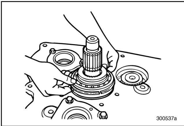
Figure 103 — Removing Front Mainshaft Rear Bearing
