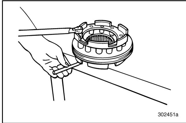
Figure 261 — Removing 12-Point Screws
