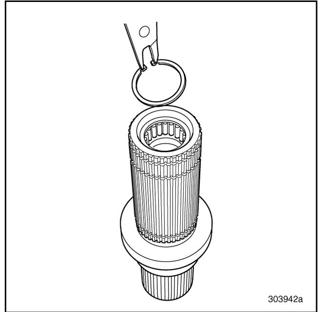
Figure 370 — Installing Spigot Bearing Snap Ring (T313L/T318L Shown)
