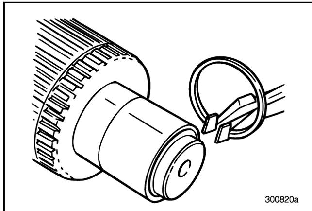
Figure 403 — Installing Inner Race Snap Ring (T313L/T318L Shown)
