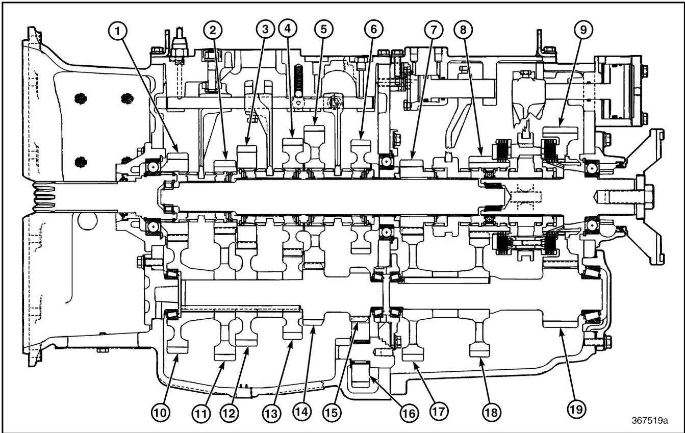
Figure 585 — Gear Identification (T313L/T318L Shown)
