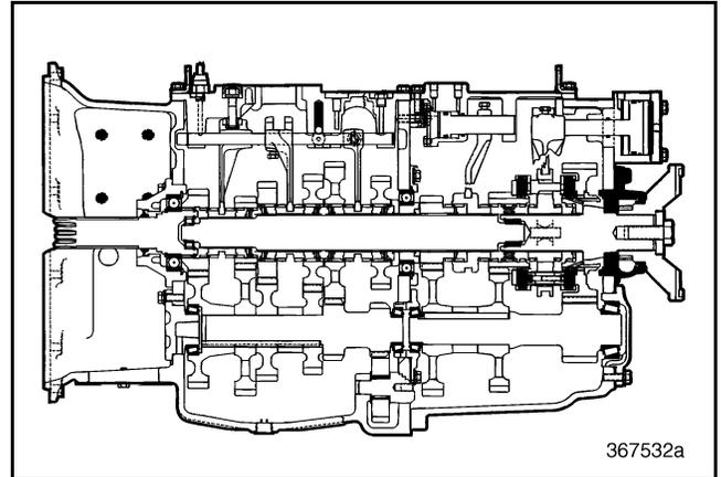
**Figure 265 — Rear Mainshaft Bearing Cover Component Locator (T313L/T318L Shown)**
