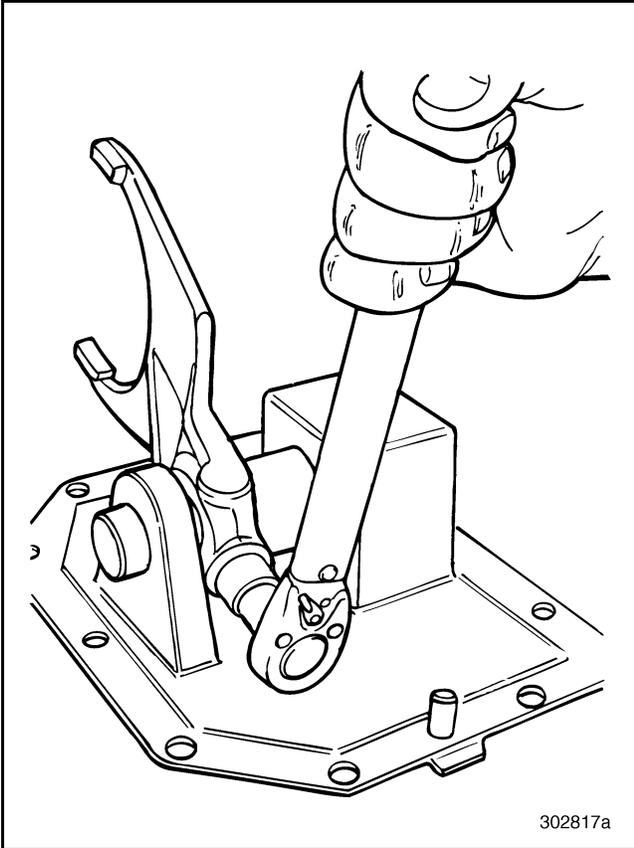
Figure 477 — Tightening Shift Fork Setscrew
