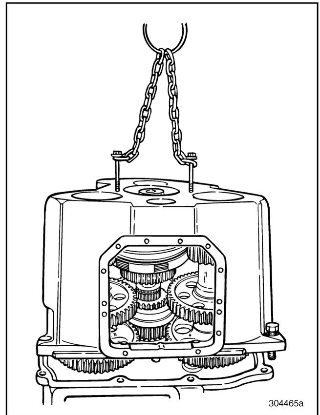
Figure 554 — Installing Rear Case
