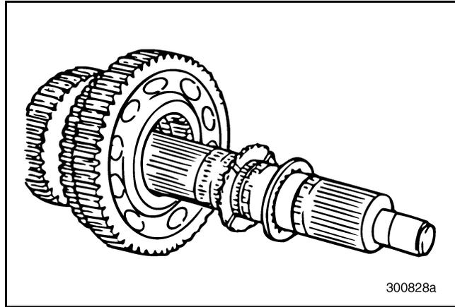
**Figure 419 — Installing Internal- and External-Toothed Thrust Washers (T313L/T318L Shown)**
