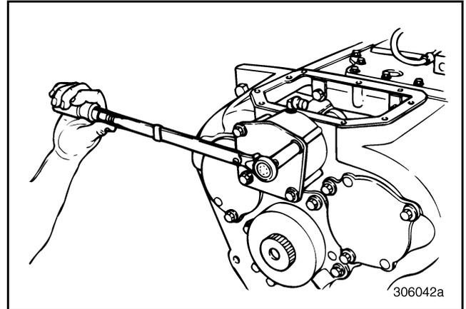
Figure 72 — Removing Range Shift Cylinder Capscrews
