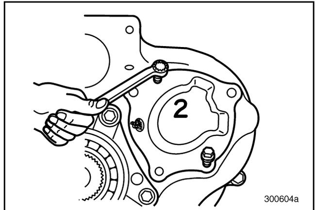
Figure 89 — Removing Bearing Cover
