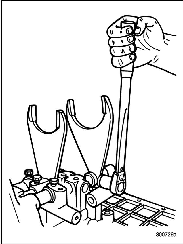
Figure 508 — Tightening Setscrew
