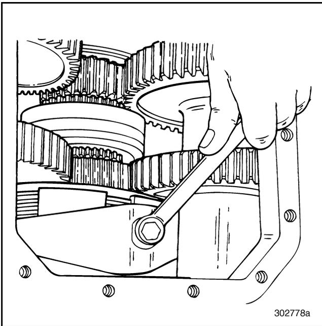
Figure 71 — Removing Range Shift Fork Setscrew
