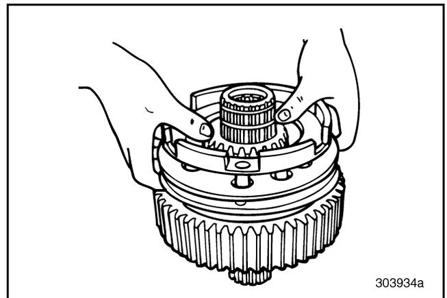
Figure 378 — Installing Synchronizer Assembly
