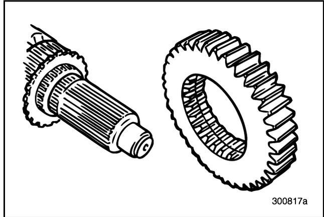
Figure 219 — Removing Second Speed Gear
