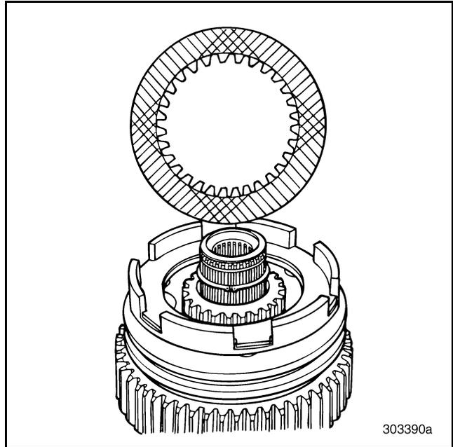
**Figure 380 — Installing Friction Disc
