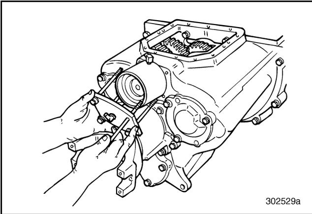
**Figure 572 — Installing Range Shift Cylinder, Capscrews, Cover and O-Ring**
