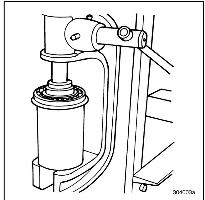
Figure 536 — Installing Front Mainshaft Rear Bearing
