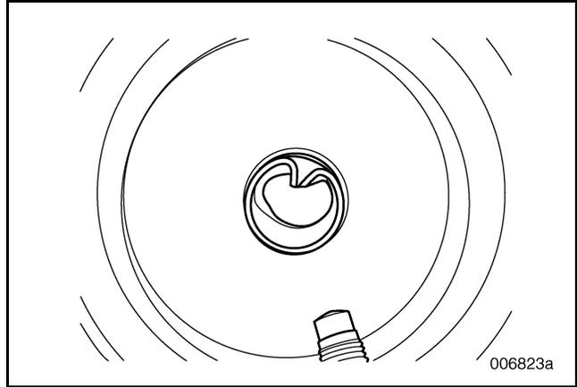
Figure 447 — Seal Properly Installed in Shift Rail Bore
