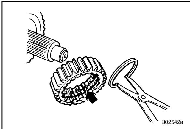
Figure 218 — Removing Snap Ring Inside Fourth Speed Gear
