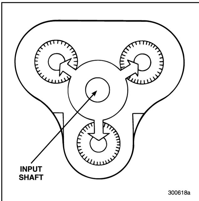
Figure 8 — Equal Torque Distribution
