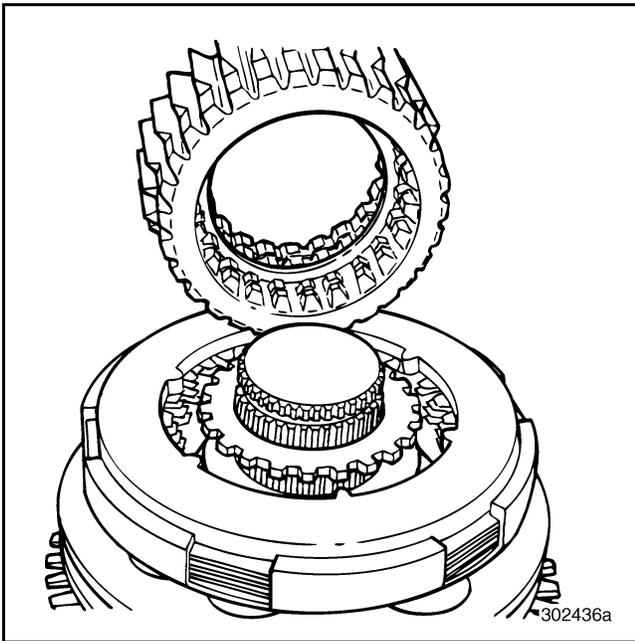
Figure 241 — Removing Hi-Range/Hi-Split Gear (T313L21/T318L21 Shown)
