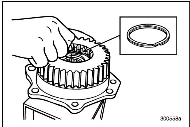
Figure 192 — Removing Snap Ring from Main Drive Pinion
