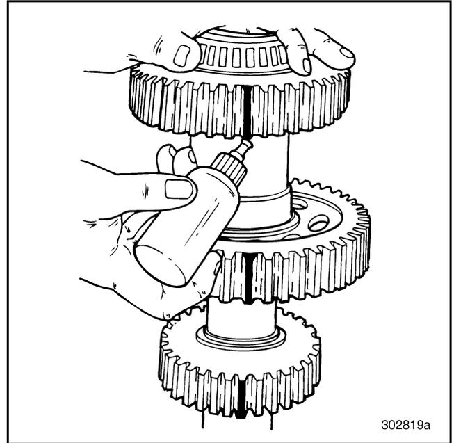
Figure 550 — Marking Rear Countershaft Gears
