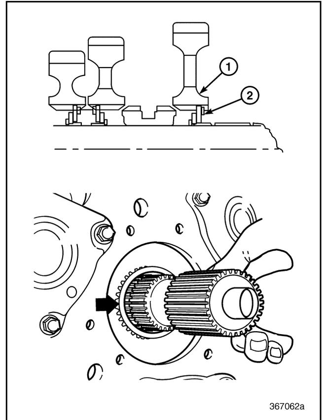
Figure 531 — Installing Reverse Gear Snap Ring (T313L/T318L Shown)
