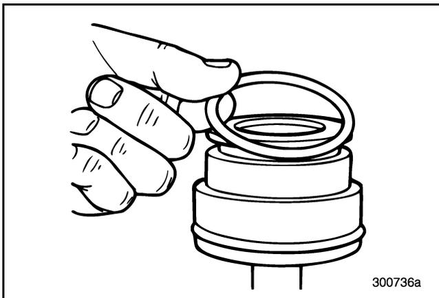
Figure 466 — Installing Shift Piston Rear O-Ring
