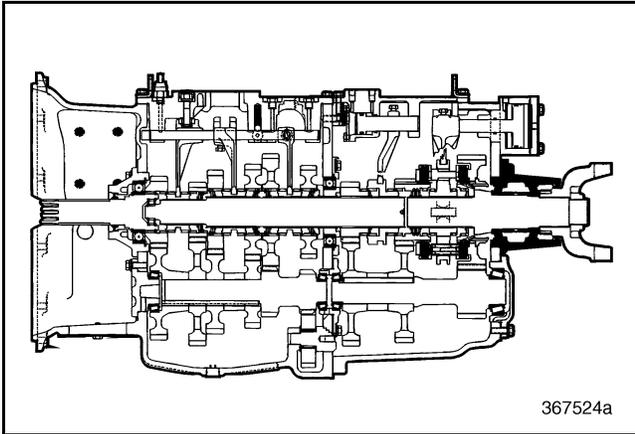
Figure 270 — Rear Output Housing Component Locator
