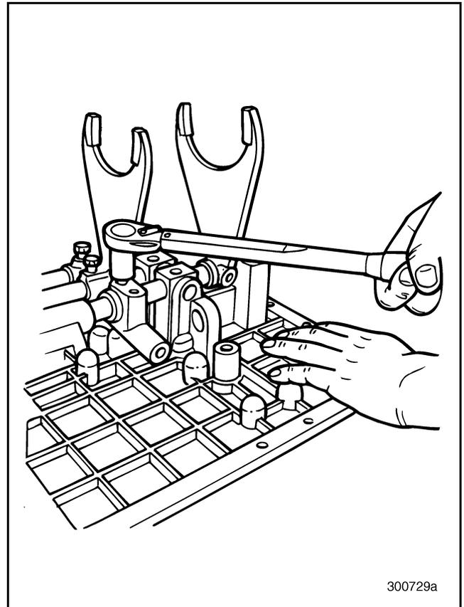
Figure 507 — Tightening Setscrew
