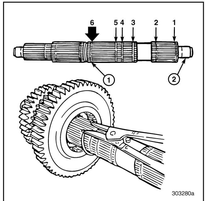
**Figure 208 — Removing Lo-Speed Gear Snap Ring (T313L/T318L Shown)**
