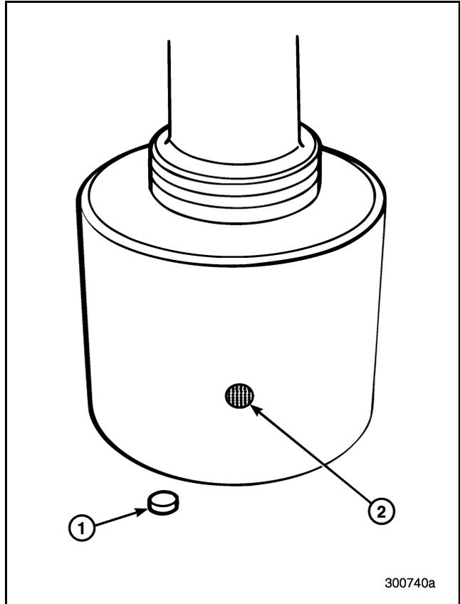
Figure 178 — Shift Cylinder Breather Vent Shown Removed (1) and Installed (2)
