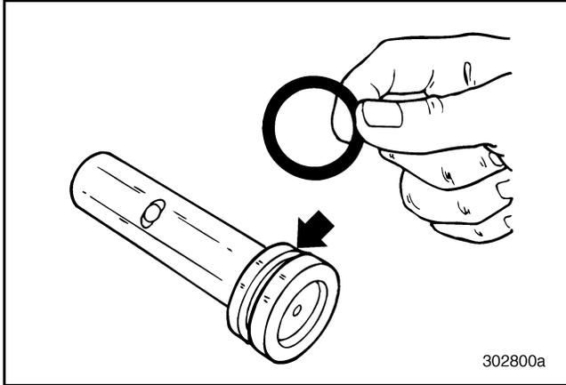
Figure 473 — Installing Shift Piston O-Ring
