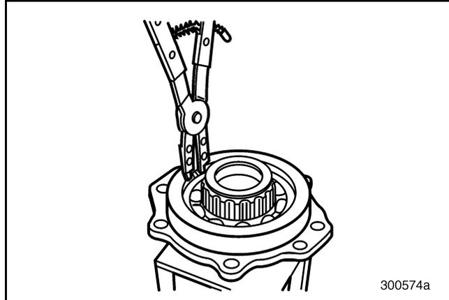
Figure 432 — Installing Snap Ring into Main Drive Pinion Bearing Cover
