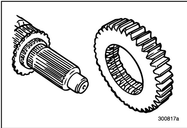
Figure 409 — Installing Second Speed Gear onto Mainshaft
