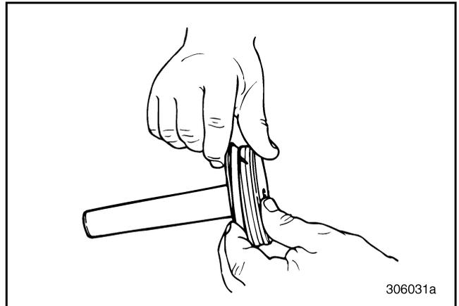
Figure 451 — Installing Teflon® Seal
