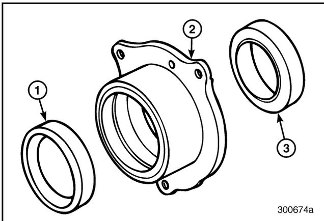
Figure 286 — Exploded View of Front Countershaft Rear Bearing Cover
