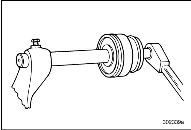
Figure 464 — Tightening Shift Piston Retaining Nut
