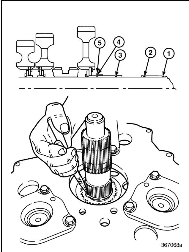
**Figure 532 — Installing Spacer Snap Ring onto Mainshaft (T313L/T318L Shown)**
