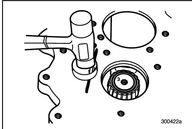
**Figure 519 — Tapping Reverse Idler Shaft into Place**
