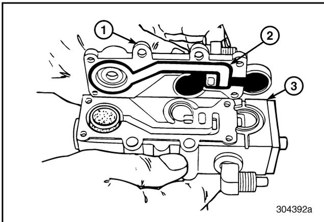
Figure 439 — Installing Top Cover Seal
