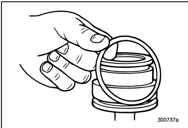
Figure 465 — Installing Shift Piston Front O-Ring
