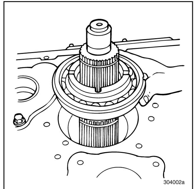
Figure 537 — Installing Front Mainshaft Rear Bearing (T313LR/T318LR Shown)
