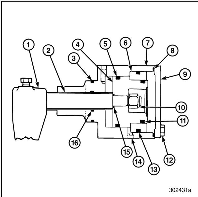
Figure 168 — Cutaway View of Range Shift Cylinder
