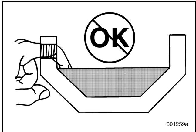
Figure 57 — Incorrect Oil Level
