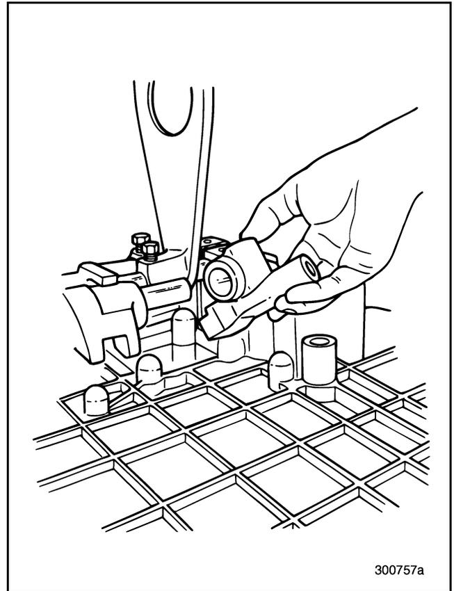
Figure 139 — Removing Lo/Reverse Shifter
