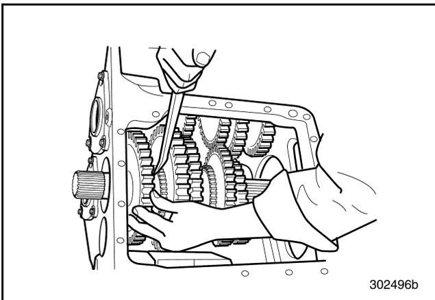
Figure 526 — Sliding Lo/Reverse Sliding Clutch and Reverse Speed Gear to Engage Gear Teeth (T313L21/T318L21 Shown)
