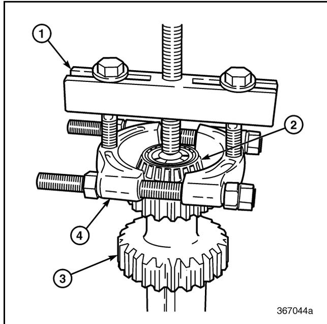
**Figure 282 — Removing Rear Bearing Cone**
