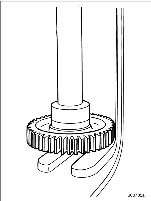
Figure 326 — Pressing Bearing Cup into Main Drive Gear
