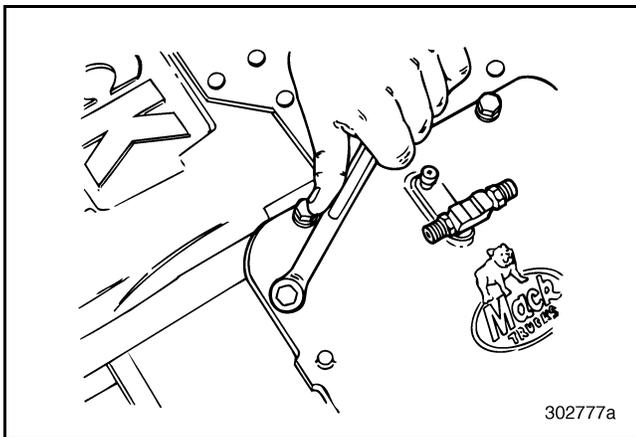
Figure 67 — Removing Rear Case Shift Cover Capscrews
