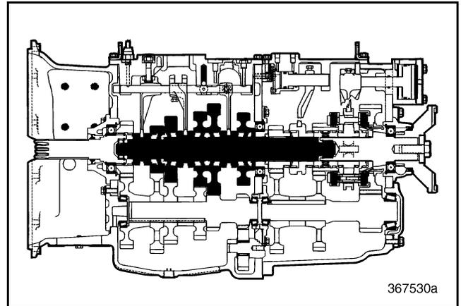
Figure 396 — Front Mainshaft Component Locator
