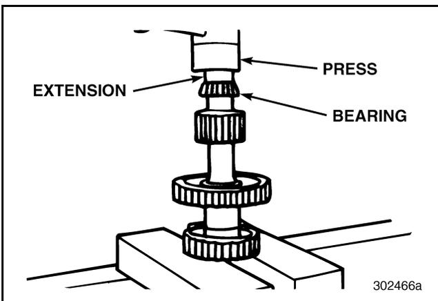
Figure 319 — Pressing on Rear Bearing Cone
