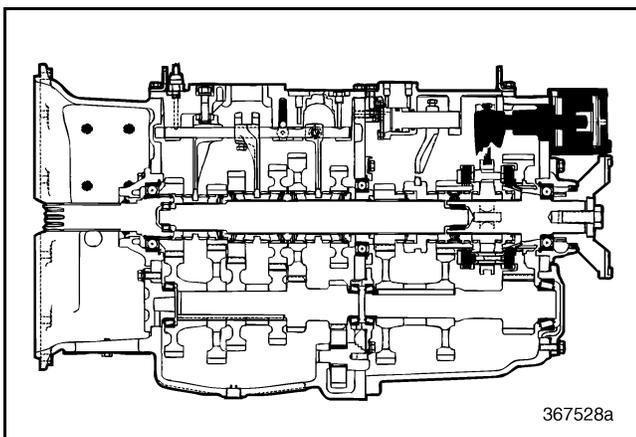
Figure 459 — Range Shift Cylinder Locator (T313L/T318L Shown)
