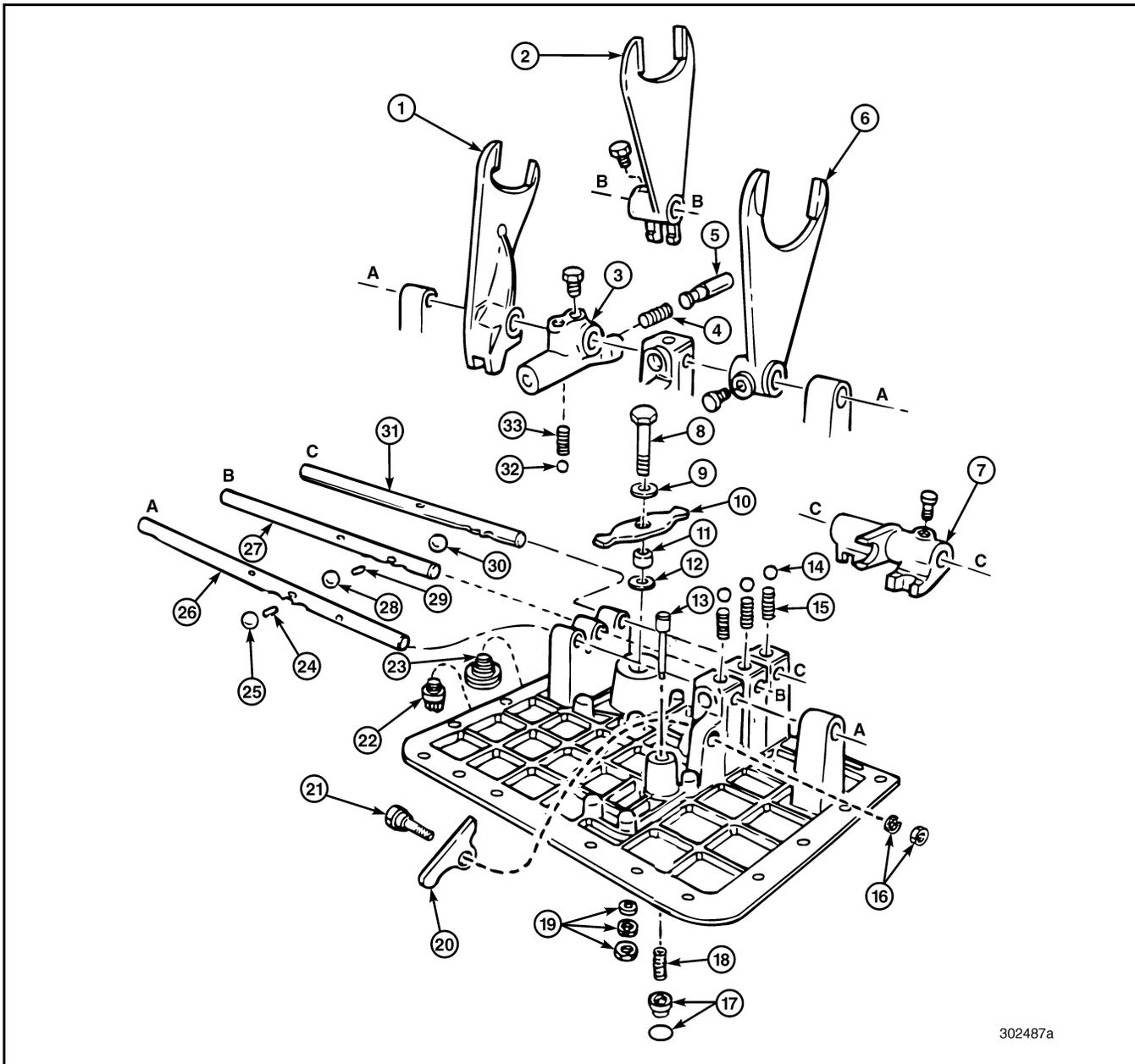
Figure 594 — Exploded View of Main Case Shift Cover
