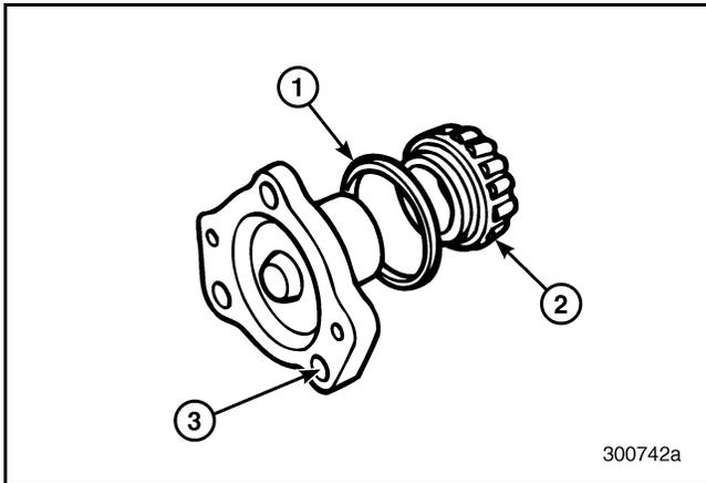
Figure 274 — Exploded View of Front Countershaft Front Bearing Cover
