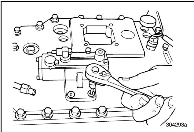
**Figure 62 — Removing Range Shift Valve Screws (Air Lines Removed for Clarity)**
