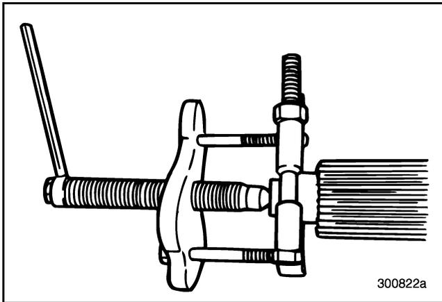
Figure 225 — Removing Front Spigot Bearing Inner Race
