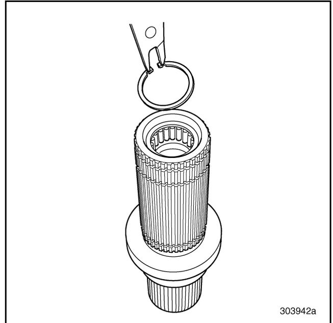
**Figure 258 — Removing Spigot Bearing Snap Ring (T313L/T318L Shown)**
