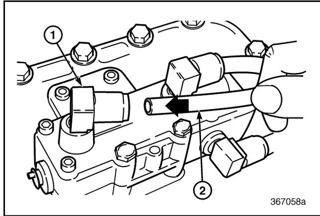
**Figure 581 — Installing Air Line**
