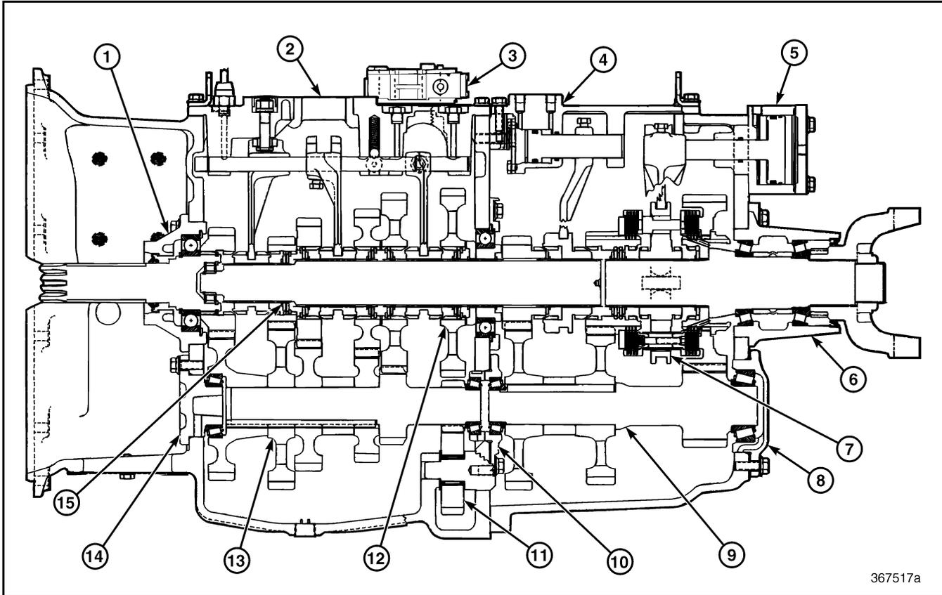
Figure 54 — Major Component Locations for T313LR21/T318LR21 Transmission
