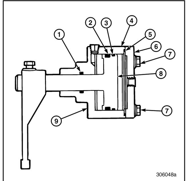
**Figure 605 — Cutaway View of Two-Position Range Shift Cylinder**
