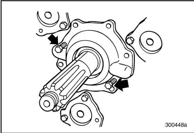
**Figure 110 — Use Jackscrews to Remove Main Drive Pinion Assembly**
