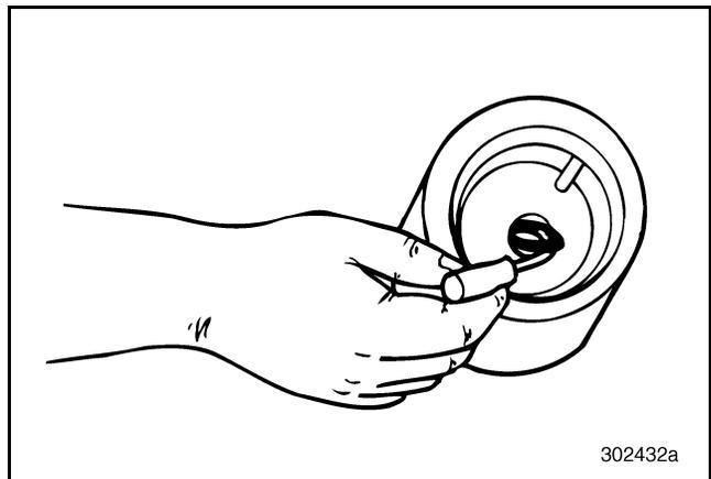
Figure 468 — Installing Shift Cylinder Inside O-Ring
