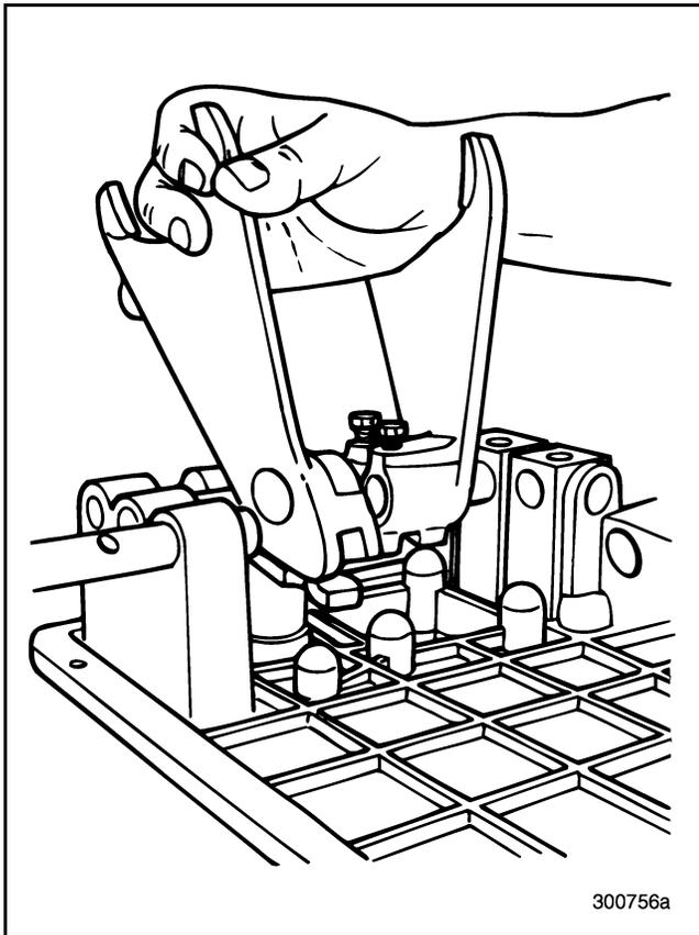
Figure 140 — Removing Third/Fourth Shift Fork
