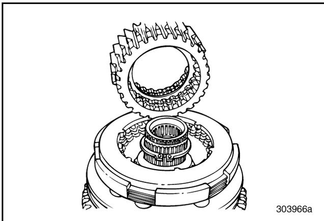
**Figure 384 — Installing Hi-Range/Hi-Split Gear into Synchronizer (T313L/T318L Shown)**
