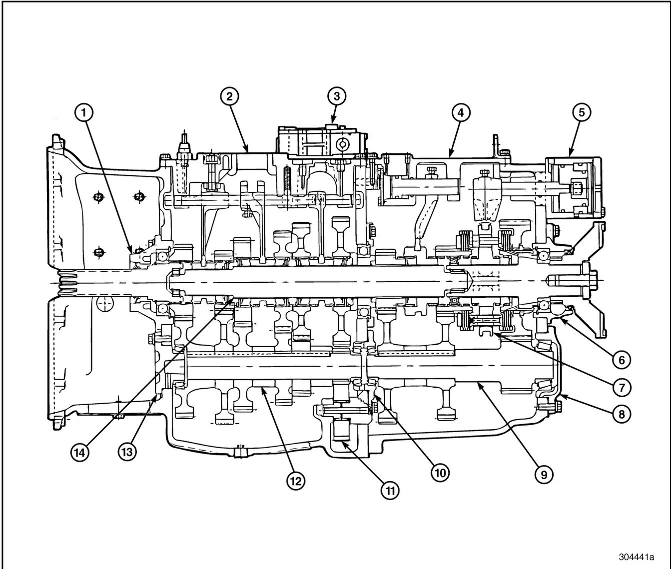
Figure 50 — Major Component Locations for T313/T318 Transmission
