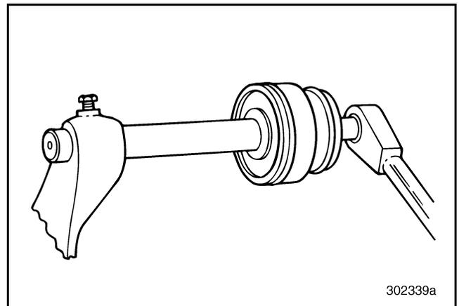
Figure 175 — Removing Shift Piston Retaining Nut
