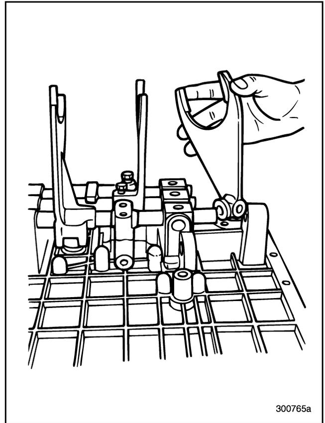
Figure 135 — Removing Lo/Reverse Shift Fork
