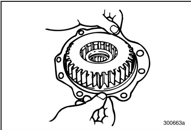
Figure 435 — Installing Main Drive Pinion Bearing Cover Gasket
