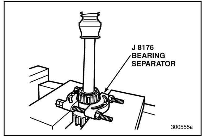
Figure 291 — Pressing off Rear Bearing Cone
