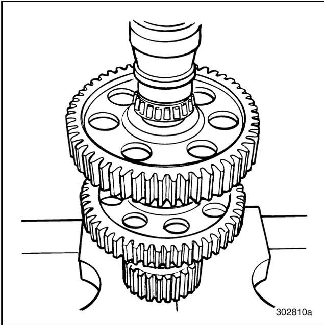
Figure 318 — Pressing on Front Bearing Cone
