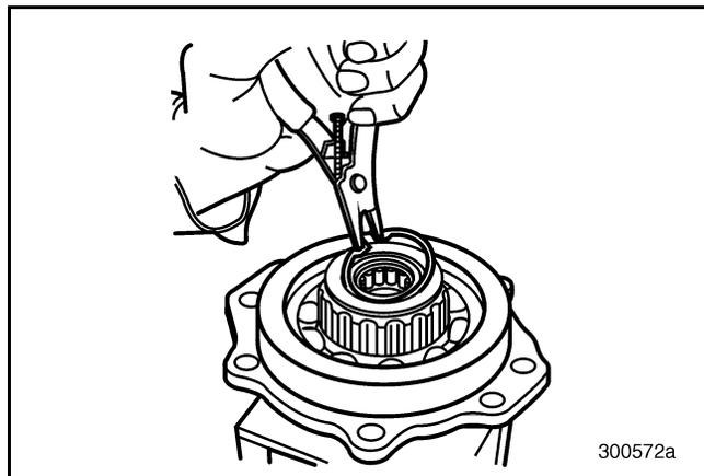
Figure 433 — Installing Spigot Bearing and Snap Ring
