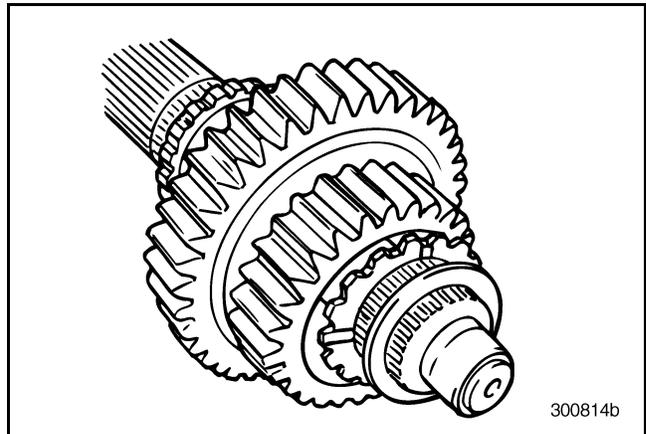
Figure 412 — Installing Internal- and External-Toothed Thrust Washers
