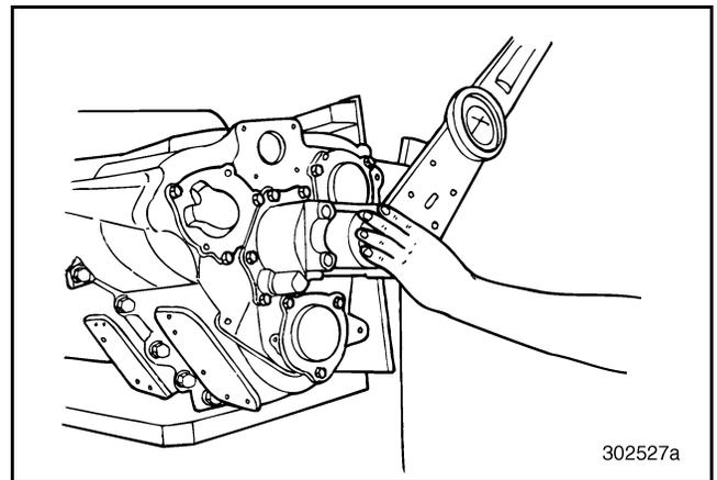
**Figure 567 — Torquing Drive Yoke Nut (T313L21/T318L21 Shown)**
