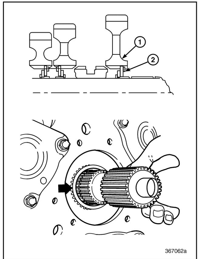
Figure 106 — Removing Snap Ring from Inside Reverse Speed Gear (T313L/T318L Shown)
