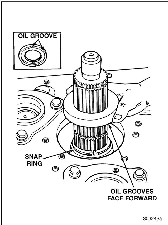
Figure 105 — Removing Front Mainshaft Spacer and Snap Ring (T313L/T318L Shown)
