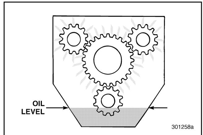
Figure 9 — Splash Lubrication
