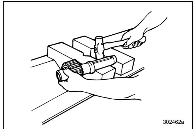
Figure 314 — Installing Key
