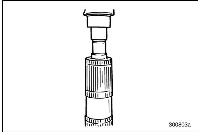
Figure 402 — Installing Spigot Bearing Inner Race (T313L/T318L Shown)
