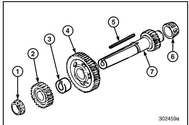
**Figure 598 — Exploded View of Rear Countershaft**
