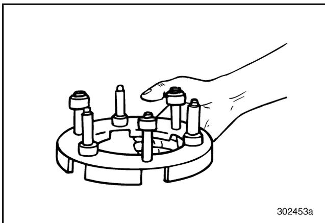
**Figure 264 — Removing Synchronizer Pins**
