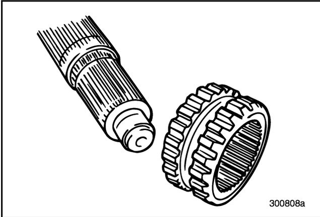
Figure 405 — Installing First/Second Sliding Clutch onto Mainshaft
