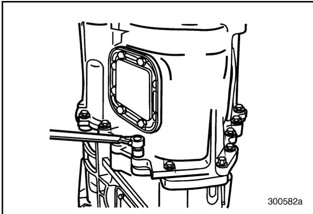
Figure 555 — Tightening Outer Case-to-Case Capscrews
