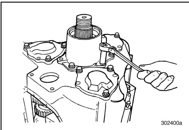
**Figure 79 — Removing Extended Output Housing Capscrews (T313L21/T318L21 Shown)**
