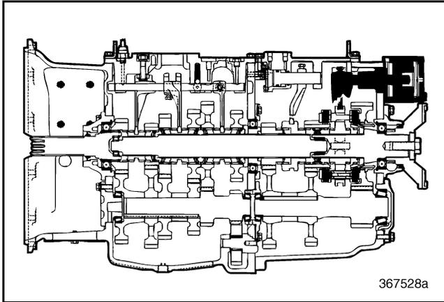
Figure 167 — Range Shift Cylinder Component Locator (T313L/T318L Shown)
