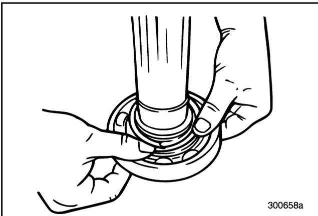
Figure 428 — Installing Spiral Snap Ring
