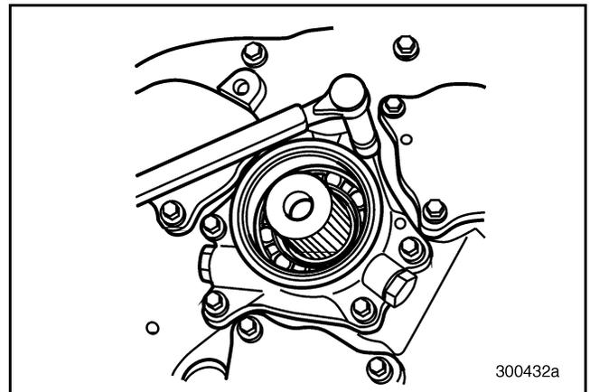
Figure 560 — Installing Rear Mainshaft Bearing Cover Assembly and Tightening Capscrews (T313LR/T318LR Shown)
