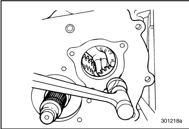
Figure 525 — Installing No. 2 Reverse Idler Shaft and Gear
