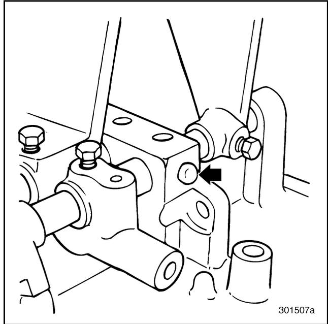
Figure 509 — Installing Interlock Ball into Cover
