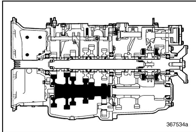
Figure 324 — Front Countershaft Component Locator (T313L/T318L Shown)
