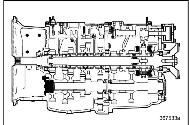
Figure 335 — Front Countershaft Front Bearing Cover Component Locator (T313L/T318L Shown)
