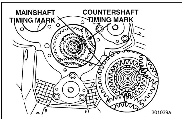
Figure 523 — Timing Gears with Mainshaft in Place
