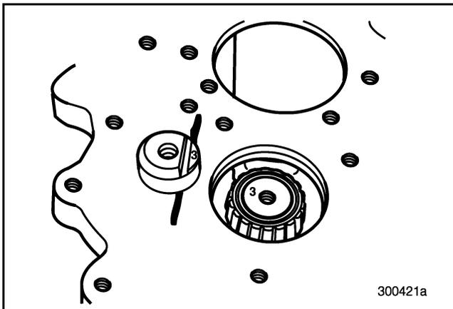
**Figure 518 — Aligning Reverse Idler Shaft with Marks**
