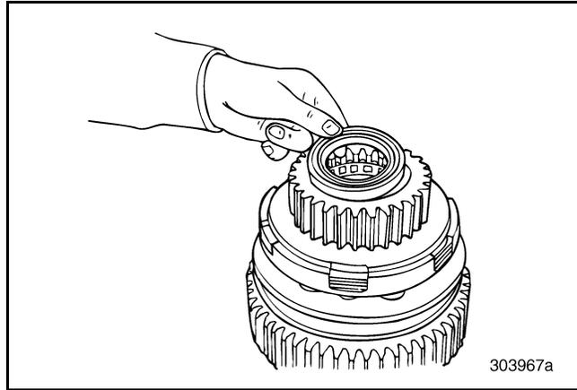
**Figure 385 — Inserting Ball Bearing
