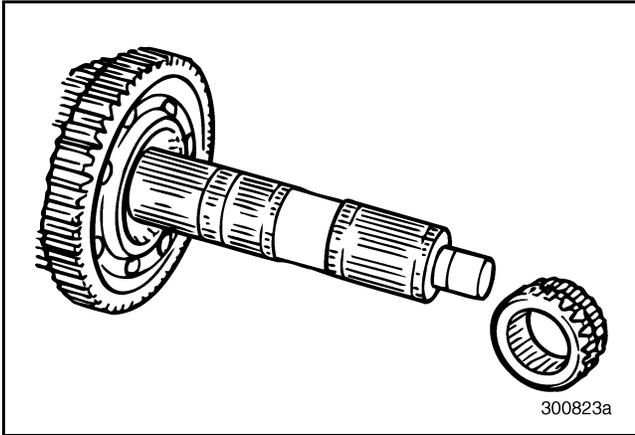
Figure 421 — Installing Lo/Reverse Sliding Clutch onto Mainshaft (T313L/T318L Shown)
