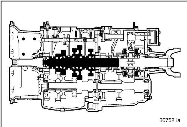
Figure 202 — Front Mainshaft Component Locator (T313L21/T318L21 Shown)
