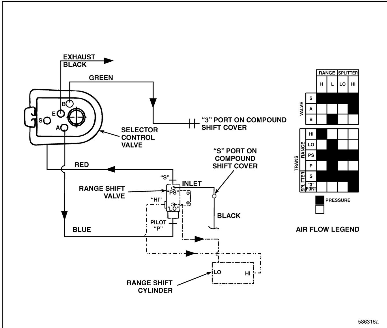
Figure 590 — Air Control Schematic
