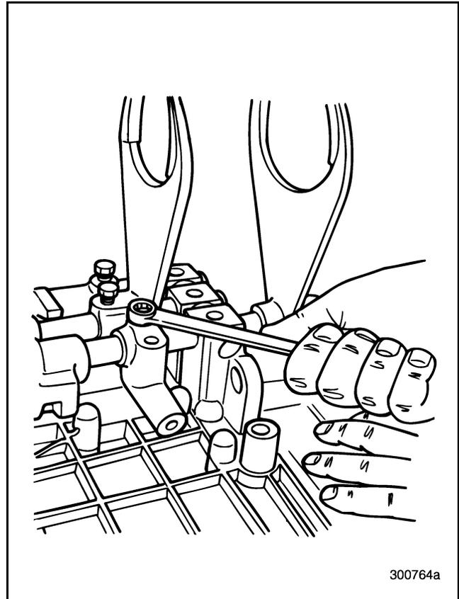
Figure 133 — Removing Setscrew from Lo/Reverse Shifter
