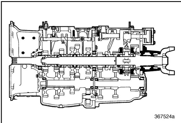
Figure 346 — Rear Output Housing Component Locator
