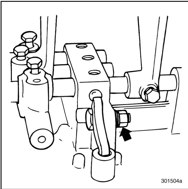
**Figure 511 — Installing Nut and Washers**
