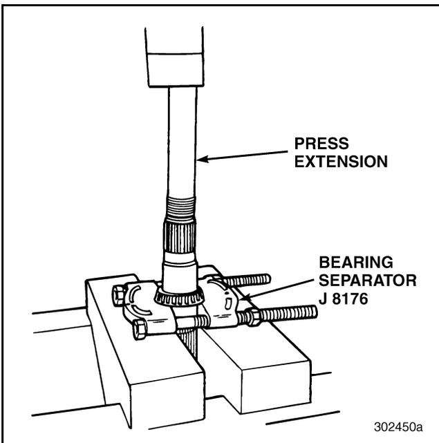
**Figure 257 — Separating Bearing Cone from Output Shaft (T313L21/T318L21 Shown)**
