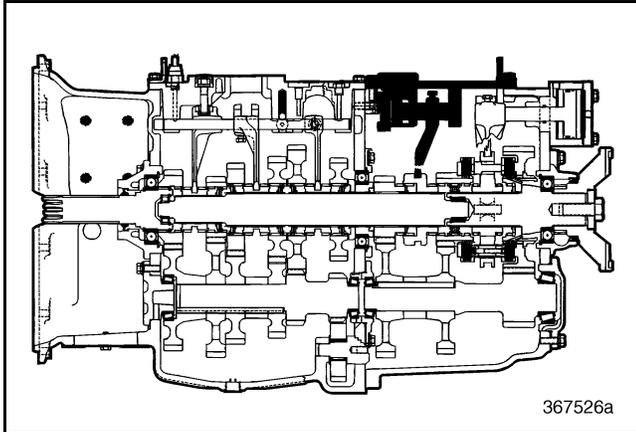
Figure 159 — Rear Case Shift Cover Component Locator (T313L/T318L Shown)
