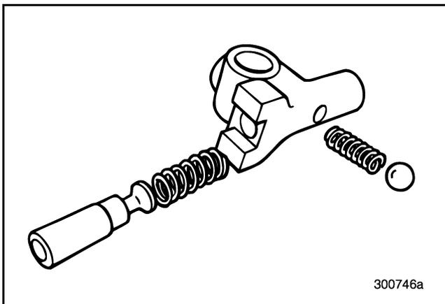
Figure 499 — Assembling Lo/Reverse Shifter
