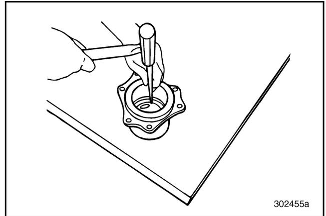
Figure 272 — Removing Bearing Cup from Housing
