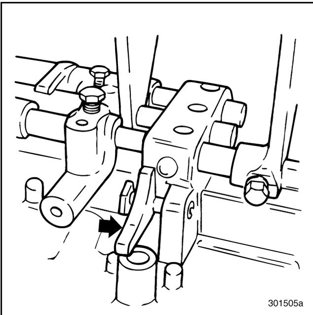
Figure 130 — Remove Interlock Rocker and Bolt
