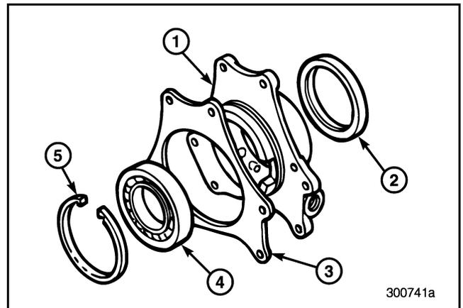
**Figure 266 — Exploded View of Rear Mainshaft Bearing Cover**
