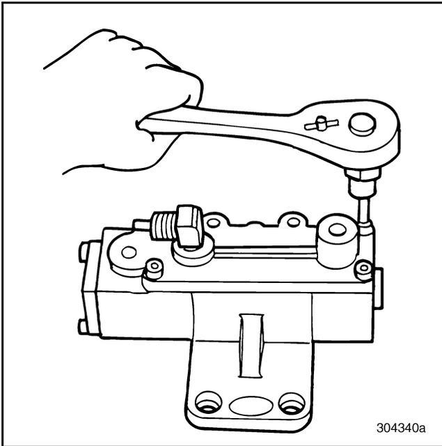
Figure 187 — Valve Top Cover Screws
