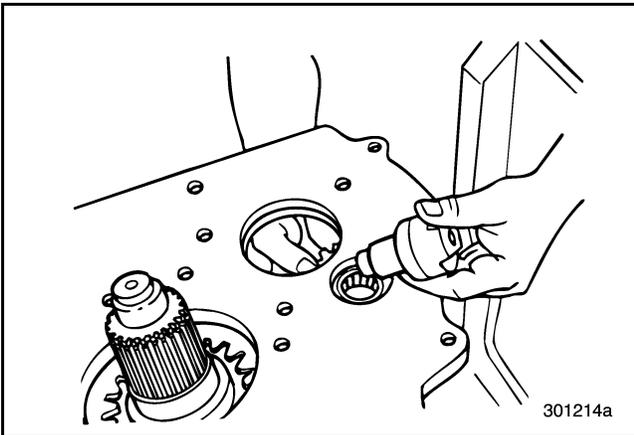
Figure 119 — Removing Reverse Idler Gear and Shaft
