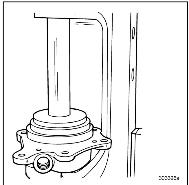
Figure 343 — Pressing Bearing into Cover
