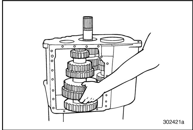
**Figure 533 — Installing No. 2 Countershaft (T313L21/T318L21 Shown)**
