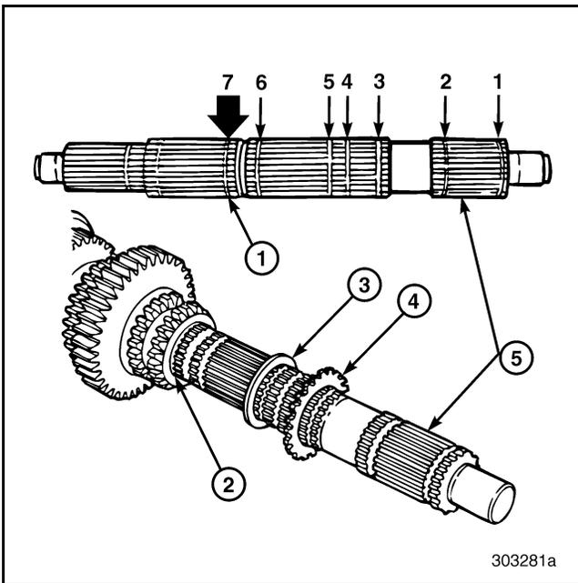
**Figure 214 — Removing Internal- and External-Toothed Thrust Washers and Snap Ring (T313L/T318L Shown)**
