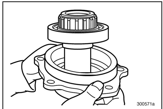
Figure 197 — Removing Main Drive Pinion Shaft and Bearing from Cover
