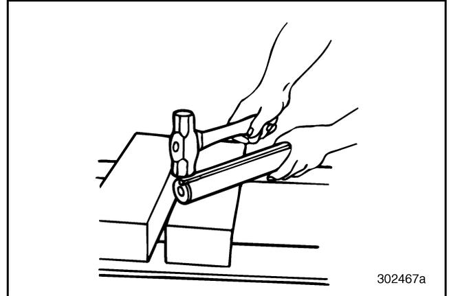
Figure 327 — Installing Key
