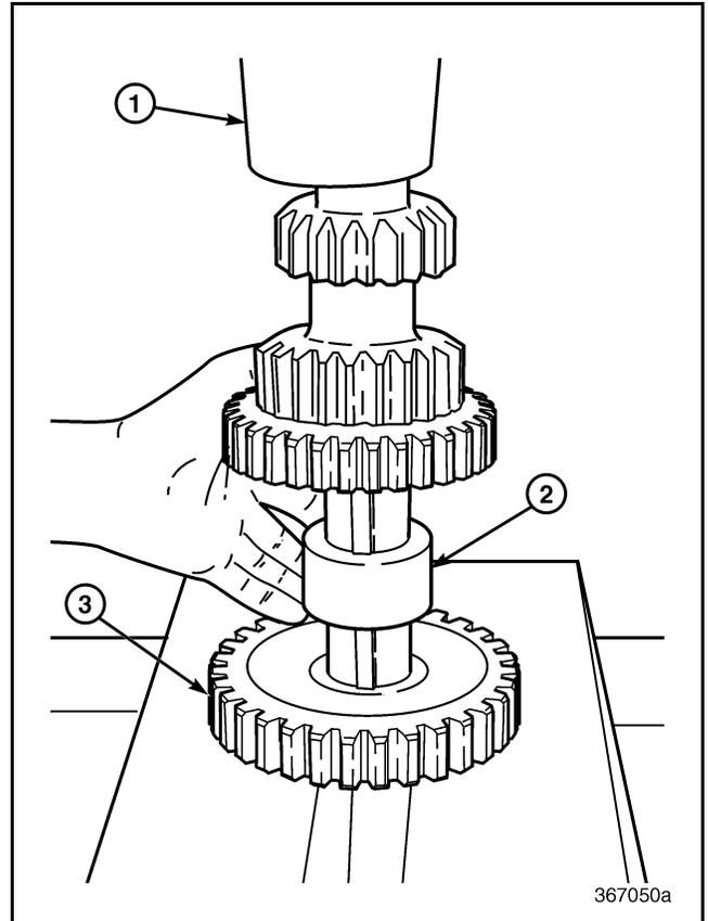
Figure 331 — Pressing Second Speed Gear onto Shaft
