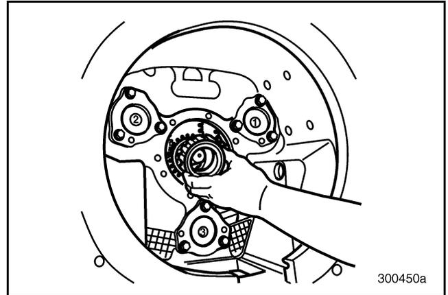
Figure 543 — Aligning Pinion Cover Oil Hole with Hole in Case
