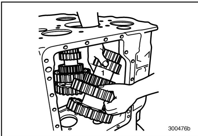
Figure 123 — Removing No. 1 Upper Left Countershaft
