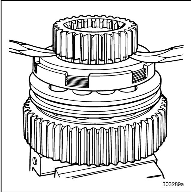
Figure 235 — Removing Hi-Range/Hi-Split Gear and Ball Bearing (T313L/T318L Shown)
