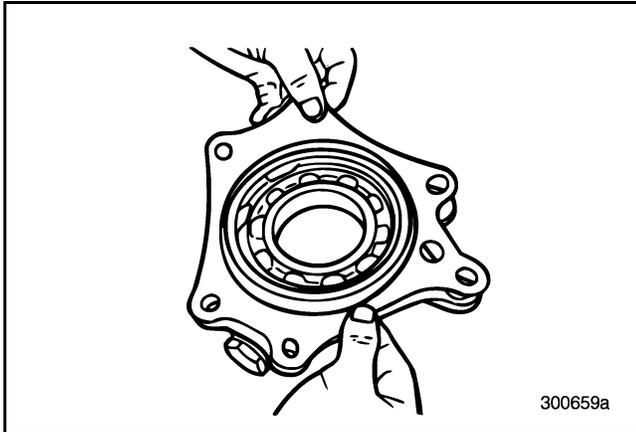
Figure 345 — Installing Gasket onto Cover
