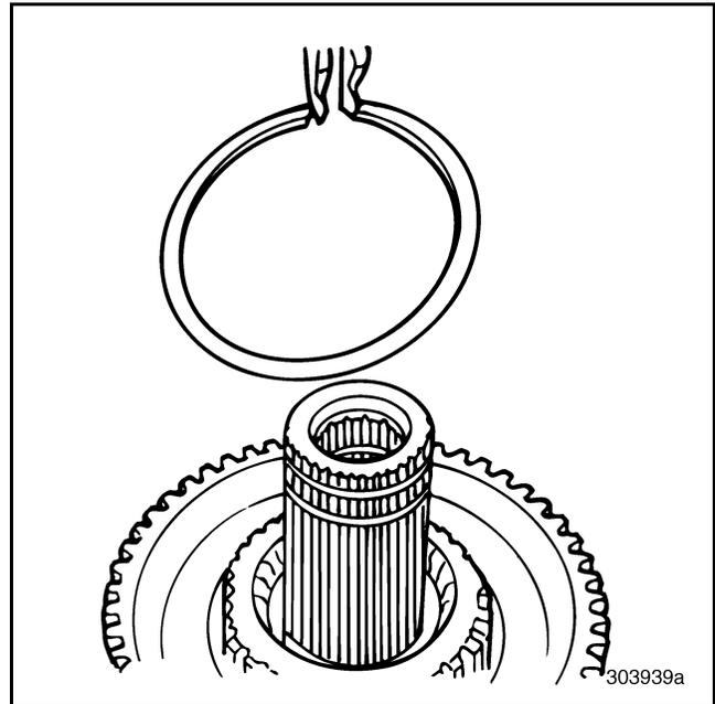
Figure 254 — Removing Gear-to-Hub Snap Ring (T313L/T318L Shown)
