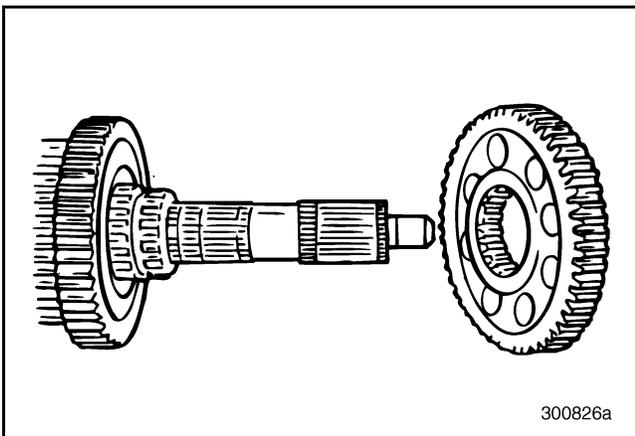
**Figure 206 — Removing Reverse Gear from Mainshaft (T313L/T318L Shown)**
