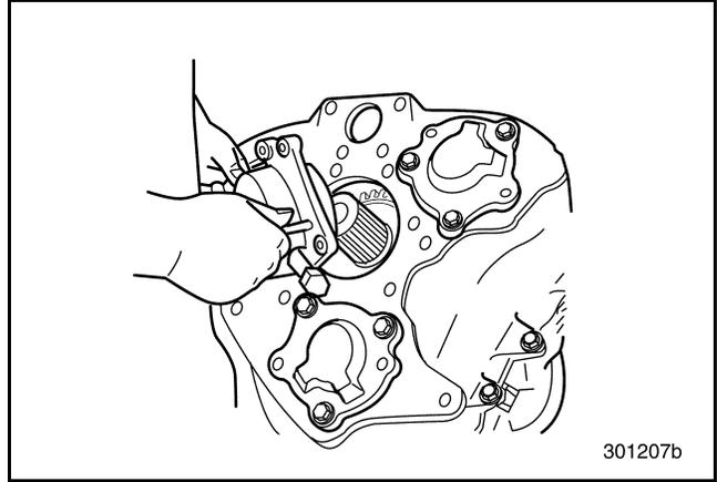
**Figure 84 — Rear Mainshaft Bearing Cover Removed**
