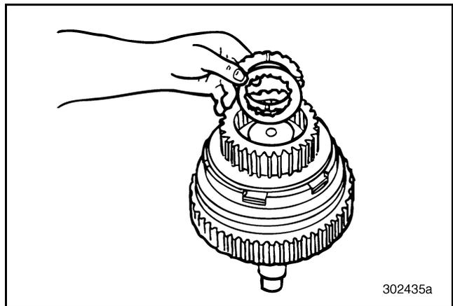
Figure 240 — Removing Thrust Washers (T313L21/T318L21 Shown)
