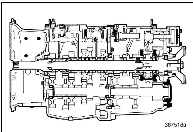
Figure 294 — Rear Countershaft Bearing Cover Component Locator (T313L/T318L Shown)
