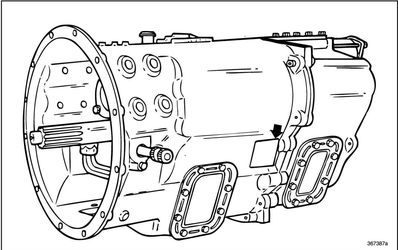
Figure 1 — Location of Identification Stamping on Left Side of Main Case
