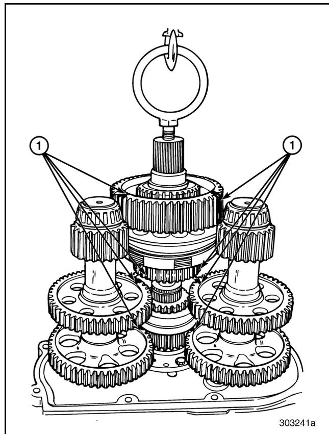
**Figure 552 — Installing Rear Mainshaft and Synchronizer Assembly (T313LR/T318LR Shown)**
