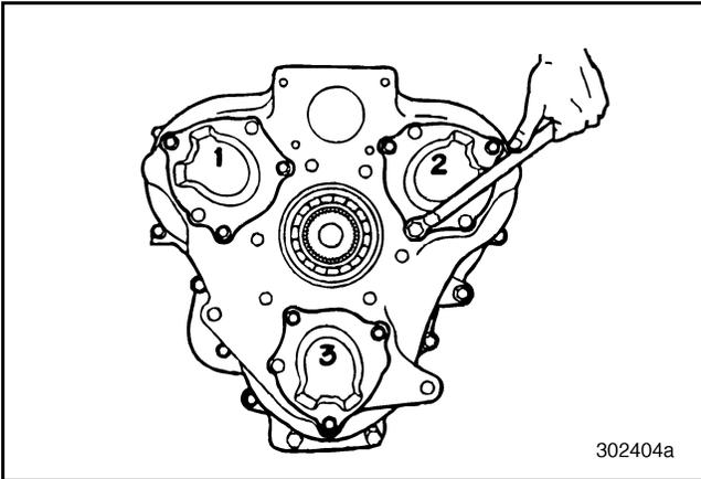
Figure 87 — Removing Rear Countershaft Bearing Cover Capscrews
