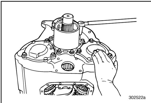
**Figure 562 — Tightening Output Housing Capscrews (T313L21/T318L21 Shown)**
