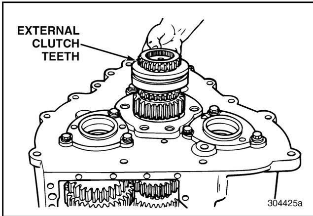
Figure 549 — Installing the Sliding Clutch
