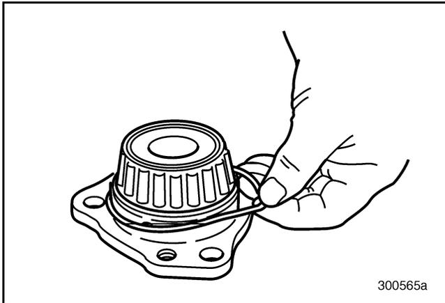
Figure 338 — Installing O-Ring onto Front Cover
