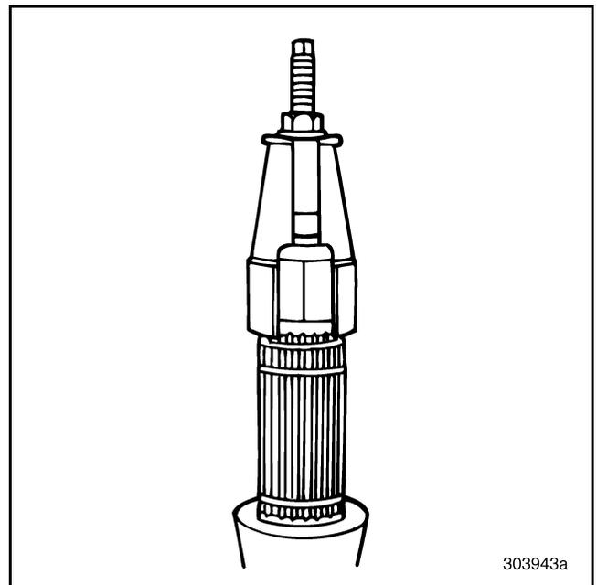
**Figure 259 — Removing Spigot Bearing from Rear Mainshaft (T313L/T318L Shown)**
