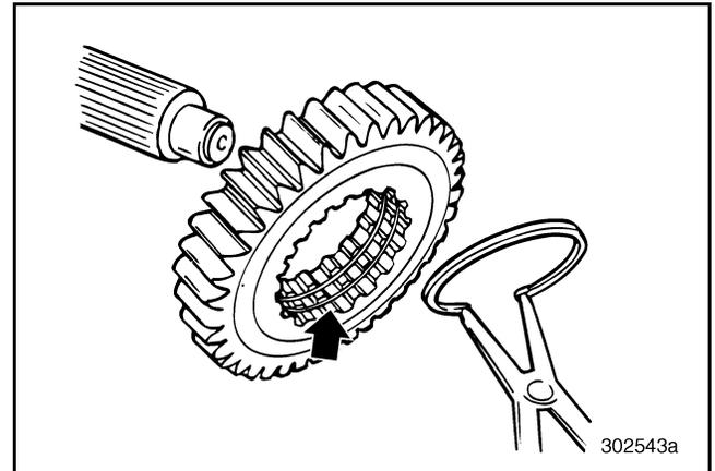
Figure 408 — Installing Snap Ring into Second Speed Gear
