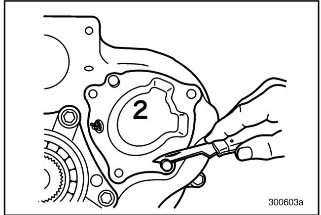
Figure 88 — Removing Jackscrew Plugs
