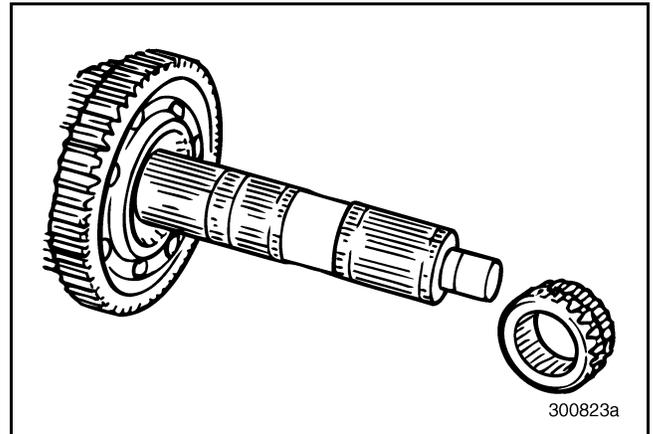
**Figure 207 — Removing Lo/Reverse Sliding Clutch from Mainshaft (T313L/T318L Shown)**
