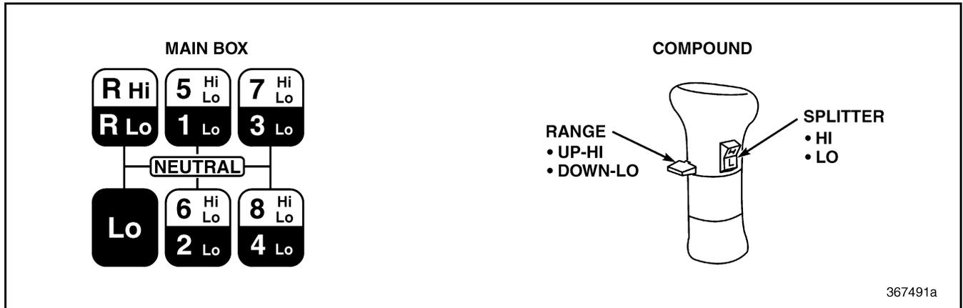
Figure 12 — T313(L)(LR)(21)(L21)(LR21) Shift Pattern
