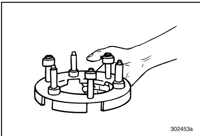
**Figure 360 — Installing Synchronizer Pins**
