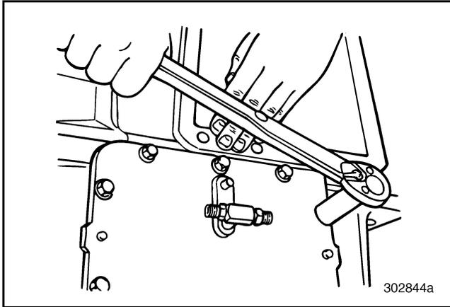
Figure 574 — Tightening Rear Case Shift Cover Capscrews
