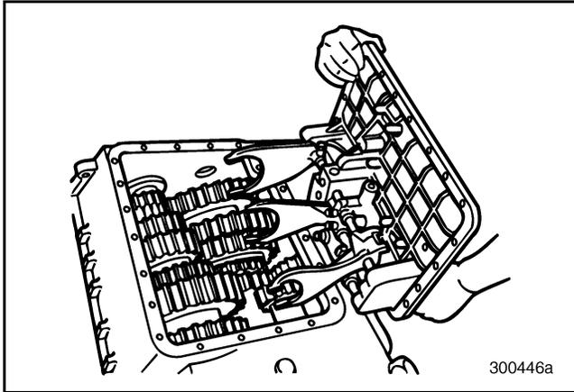
Figure 66 — Removing Main Case Shift Cover
