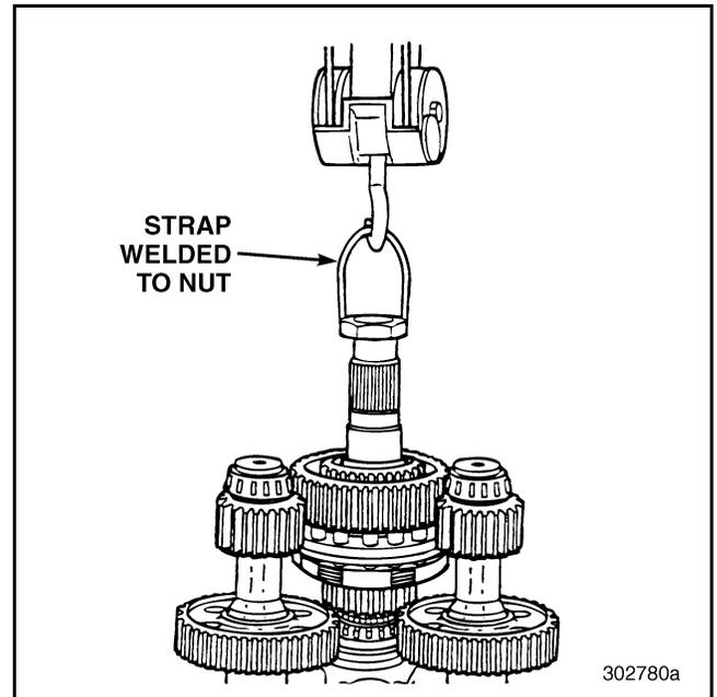
**Figure 95 — Removing Mainshaft and Synchronizer Assembly (T313L21/T318L21 Shown)**
