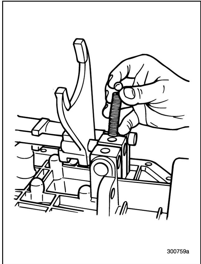
Figure 495 — Installing Poppet Ball and Spring
