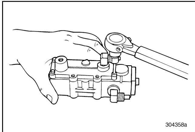
Figure 440 — Installing Top Cover
