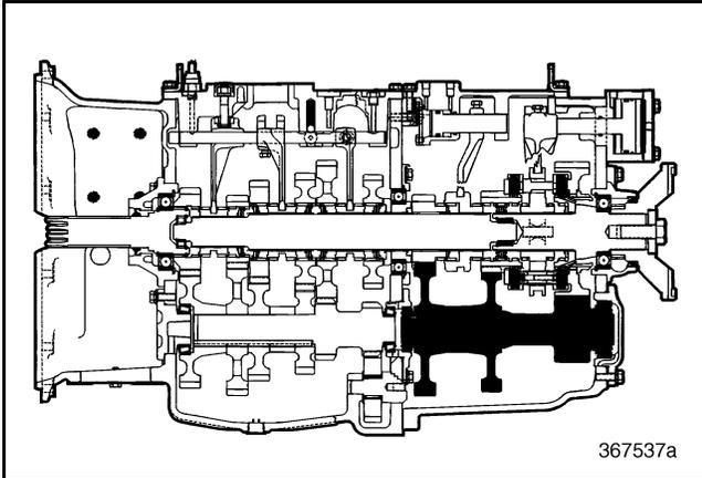
Figure 289 — Rear Countershaft Locator
