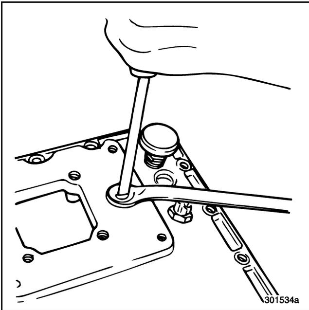
Figure 577 — Adjusting Eccentric Pin
