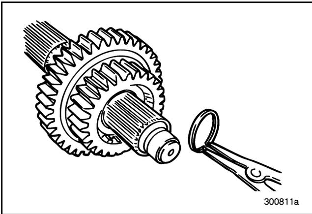
Figure 413 — Installing Fourth Speed Gear Snap Ring
