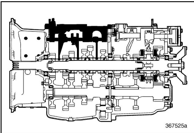
Figure 126 — Main Case Shift Cover Component Locator
