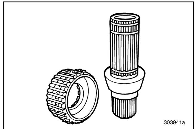
Figure 371 — Installing Lo-Range Gear Hub (T313L/T318L Shown)
