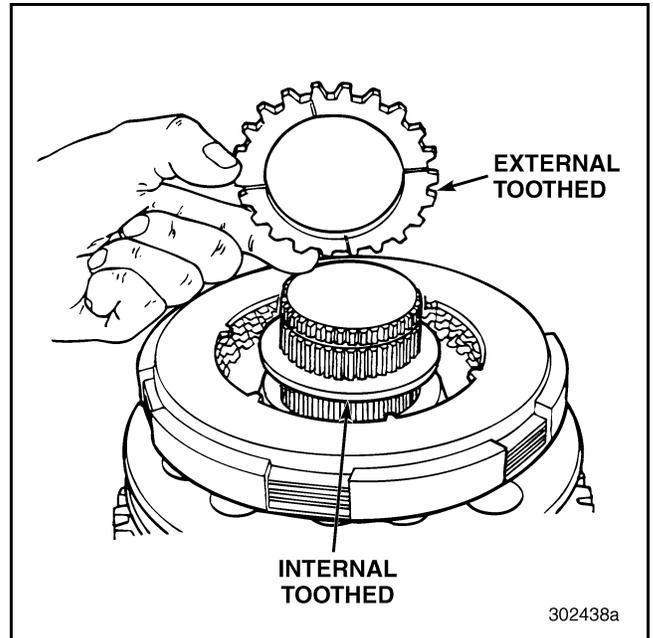
Figure 243 — Removing External-Toothed Thrust Washer (T313L21/T318L21 Shown)
