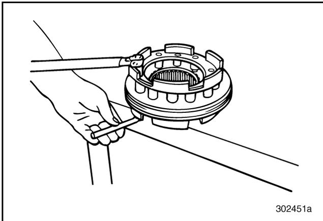
Figure 366 — Tightening 12-Point Screws
