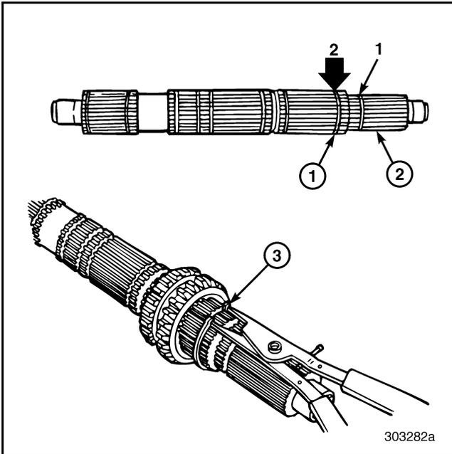
**Figure 222 — Removing Second Speed Snap Ring (T313L/T318L Shown)**
