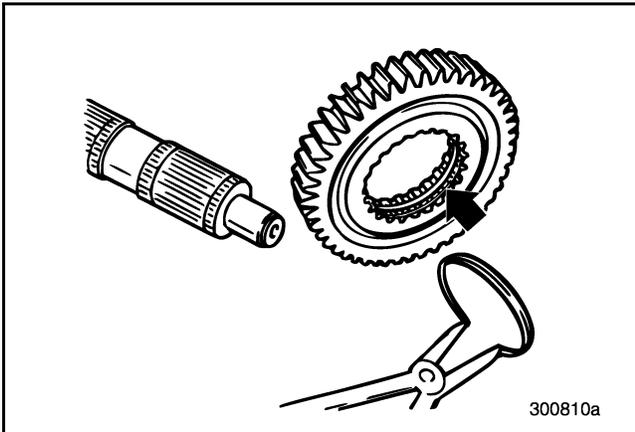
**Figure 213 — Removing First Speed Gear Snap Ring (T313L/T318L Shown)**
