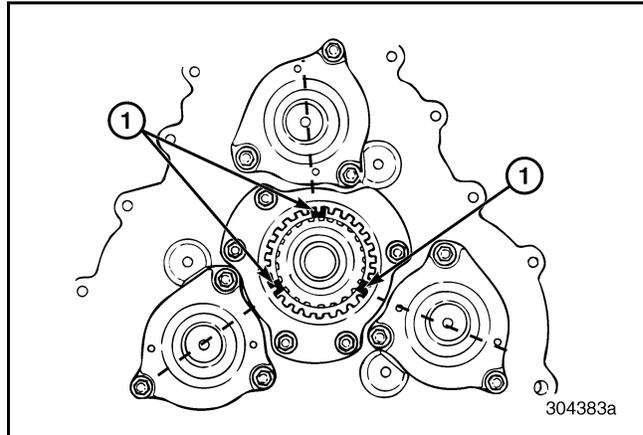
**Figure 547 — Installing and Aligning Lo-Split Gear**
