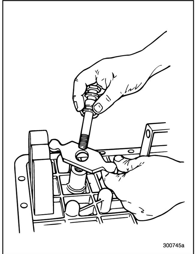
Figure 157 — Removing Third/Fourth Rocker Pin and Rocker Arm
