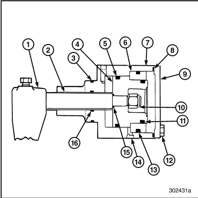
**Figure 604 — Cutaway View of Three-Position Range Shift Cylinder**
