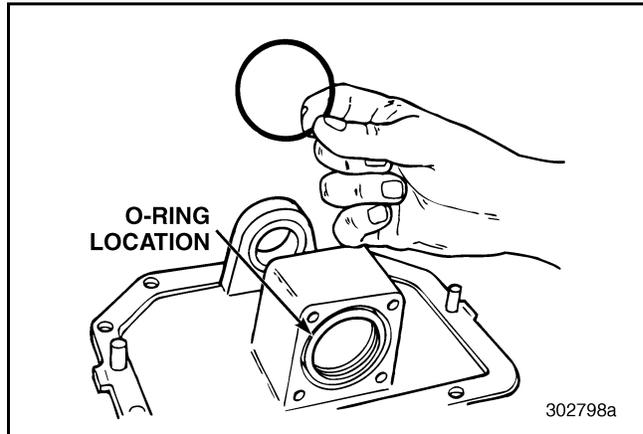
Figure 475 — Installing O-Ring onto Front of Housing
