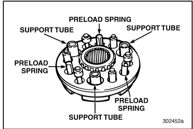
**Figure 364 — Install Support Tubes into Assembly**
