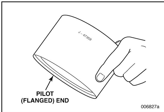
**Figure 453 — Piston Assembled in Seal Sizer/Piston Installer (Tool No. J 47359)**
