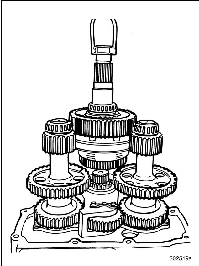
Figure 553 — Installing Output Shaft and Synchronizer Assembly (T313LR21/T318LR21 Shown)
