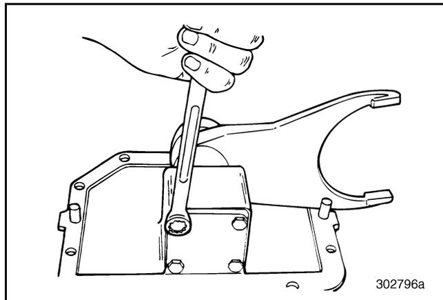
Figure 162 — Removing Cover Capscrews
