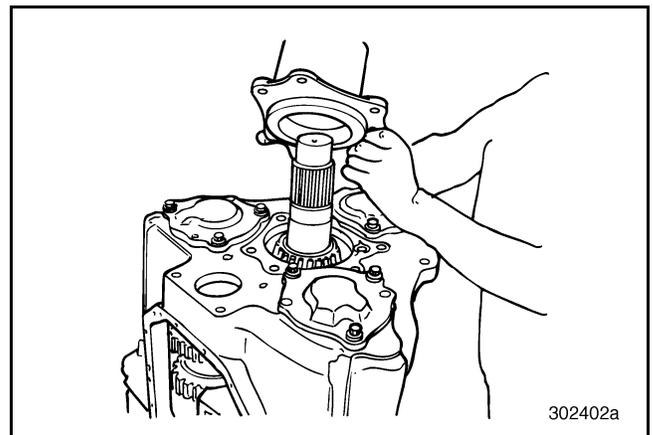
**Figure 81 — Removing Output Housing, Bearing Cone and Spacer (T313L21/T318L21 Shown)**
