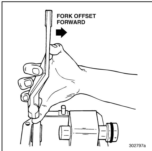
Figure 476 — Installing Piston and Shift Fork
