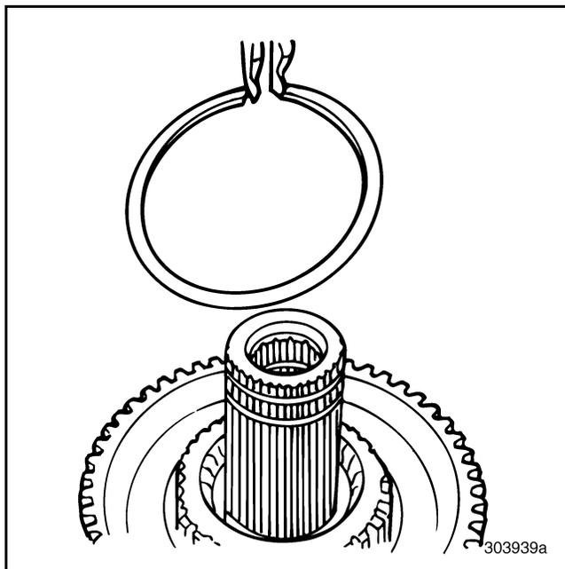
Figure 373 — Installing Lo-Range Gear-to-Hub Snap Ring (T313L/T318L Shown)
