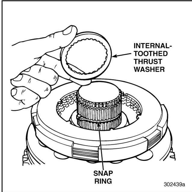
Figure 244 — Removing Internal-Toothed Thrust Washer and Snap Ring (T313L21/T318L21 Shown)
