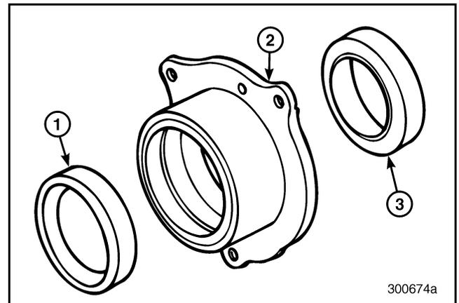
Figure 321 — Exploded View of Front Countershaft Rear Bearing Cover
