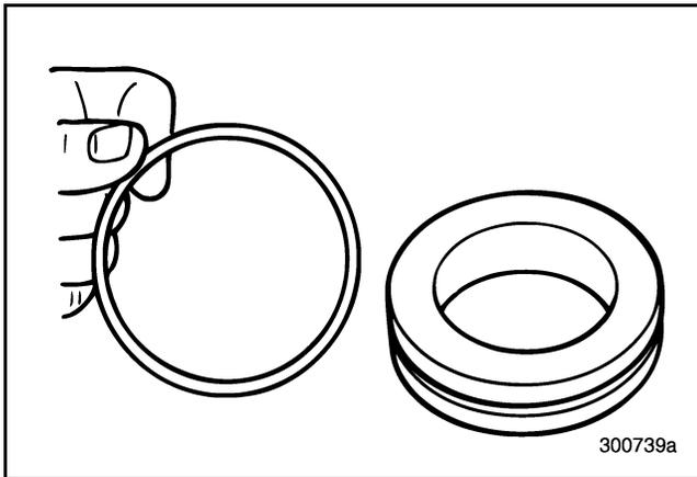
Figure 177 — Removing O-Ring from Sleeve
