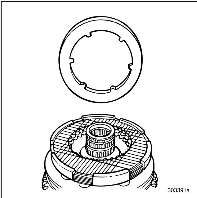
Figure 381 — Installing Spacer (T313L/T318L Shown)
