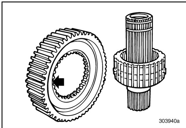
Figure 372 — Installing Lo-Range Gear
