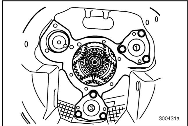
**Figure 534 — Gear Timing Marks Aligned**
