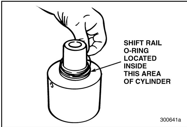
Figure 171 — Removing Shift Cylinder Outside O-Ring
