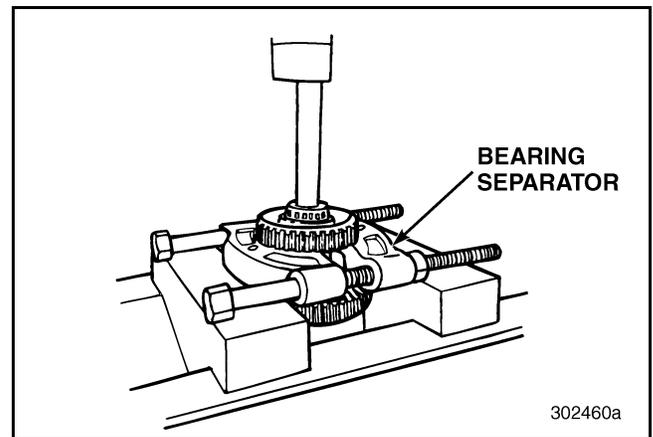
Figure 292 — Pressing off Lo-Split Gear and Bearing Cone
