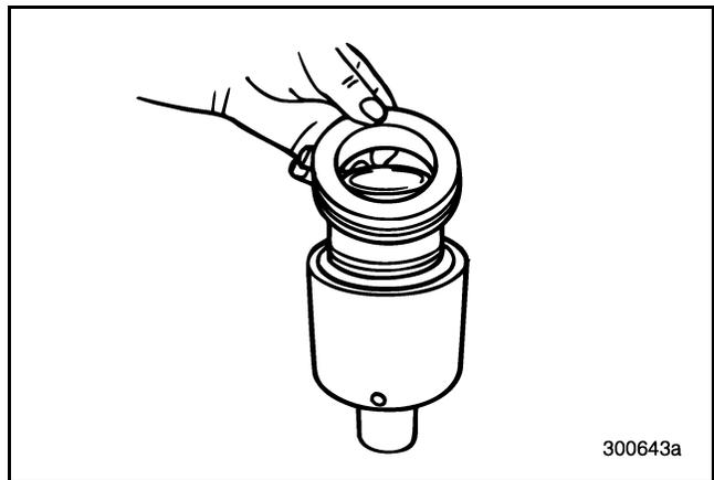
Figure 170 — Removing Sleeve from Piston
