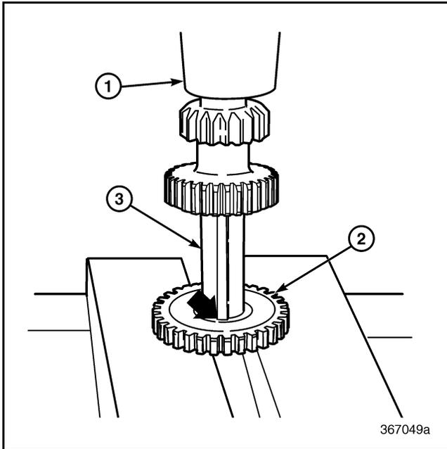
**Figure 328 — Installing First (Fifth) Gear on Countershaft**
