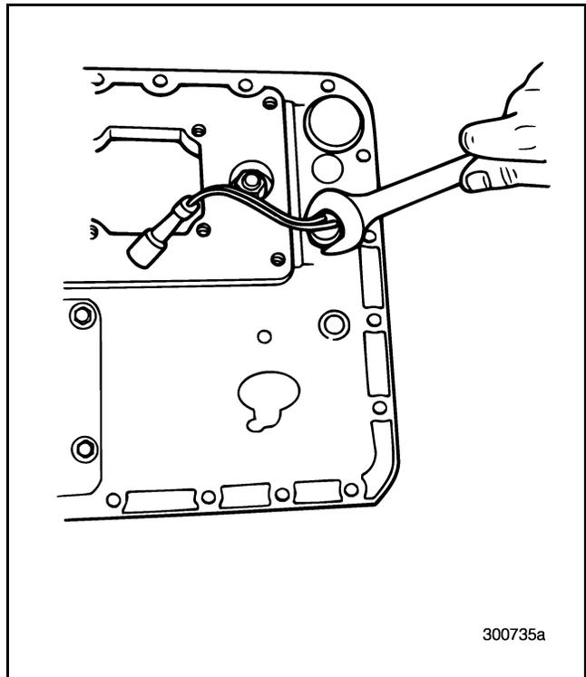
Figure 486 — Installing Reverse Light Switch
