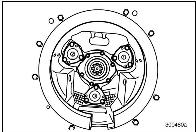
**Figure 85 — Mark Front Countershaft Front Bearing Covers for Placement**
