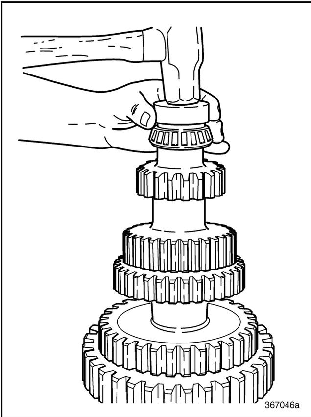
Figure 334 — Installing Rear Bearing Cone onto Shaft
