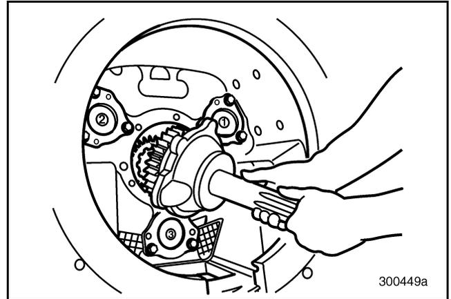
**Figure 112 — Removing Main Drive Pinion Assembly**
