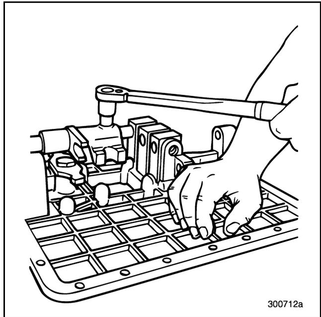
Figure 490 — Tightening Setscrew
