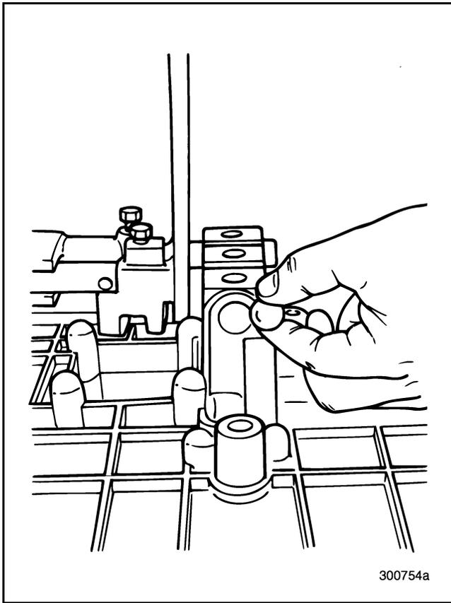
Figure 494 — Installing Interlock Ball Between Rails
