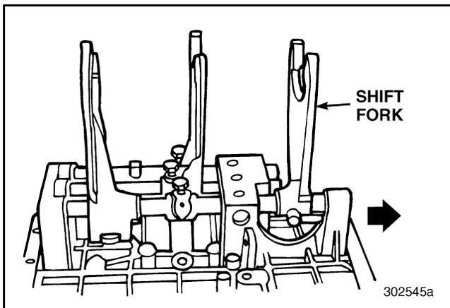
Figure 506 — Shift Rail in Position
