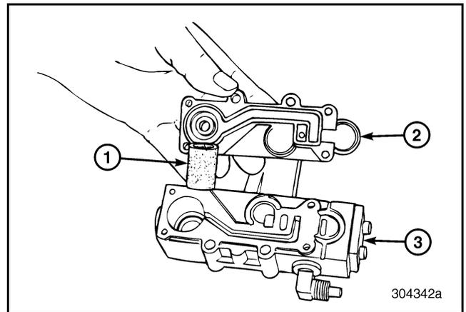
Figure 188 — Removing Sintered Bronze Filter
