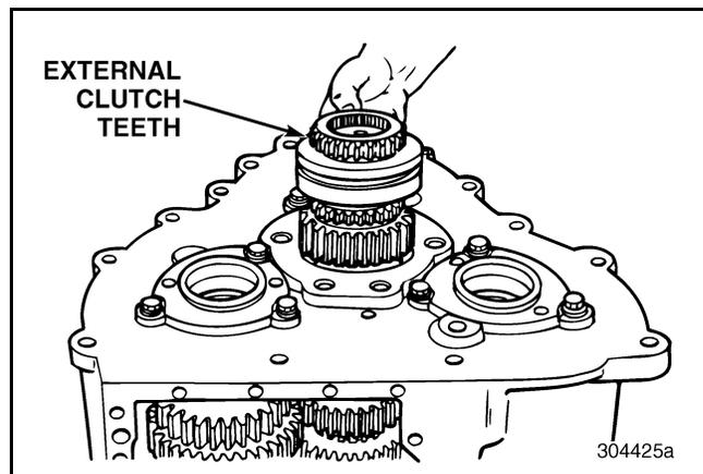
**Figure 98 — Removing Splitter Sliding Clutch**
