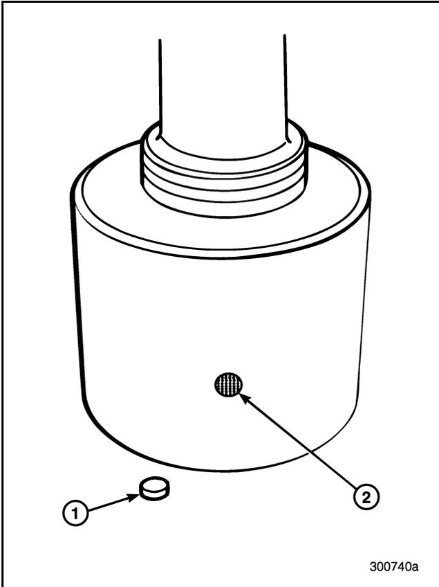
Figure 461 — Shift Cylinder Breather Vent
