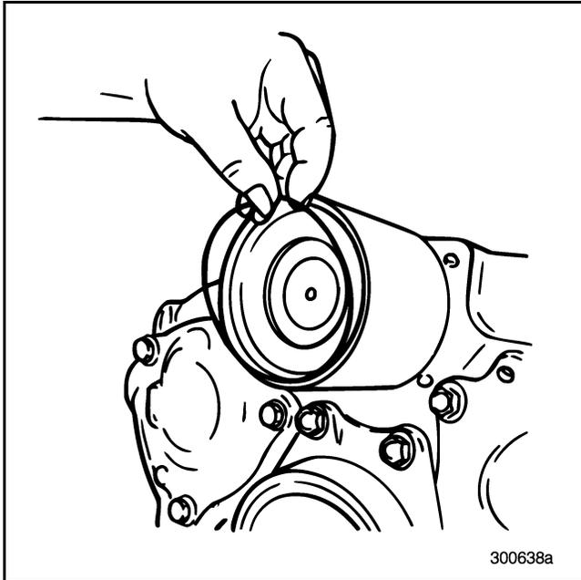
Figure 74 — Removing Range Shift Cylinder O-Ring
