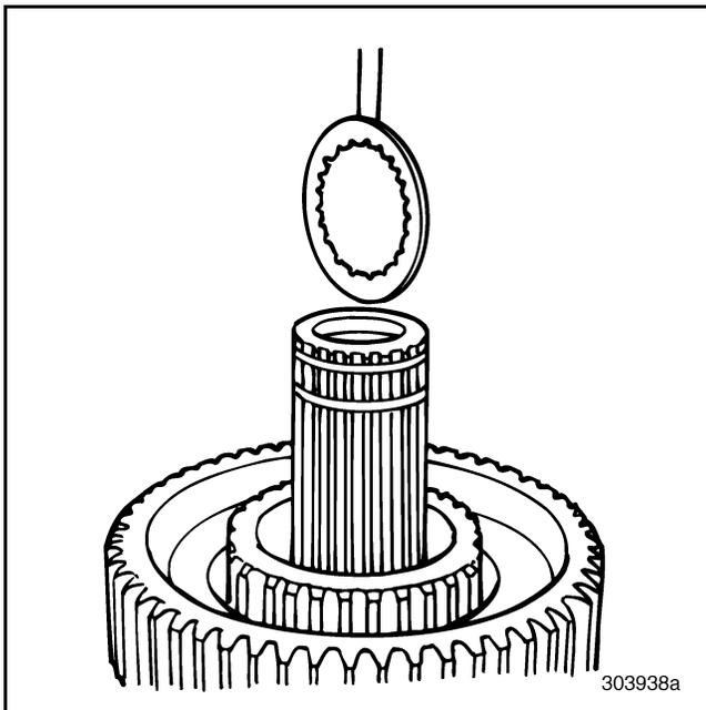
Figure 253 — Removing Hub Thrust Washer (T313L/T318L Shown)
