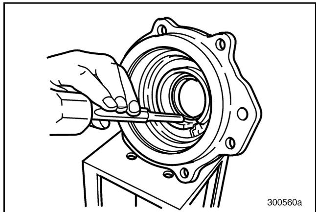
Figure 200 — Removing Bearing Cover Oil Seal
