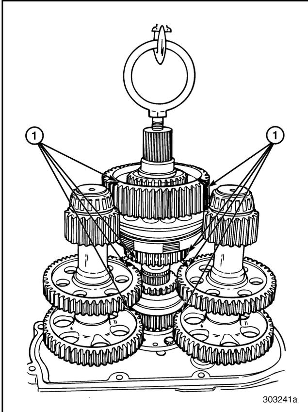
**Figure 96 — Removing Mainshaft and Synchronizer Assembly (T313L/T318L Shown)**
