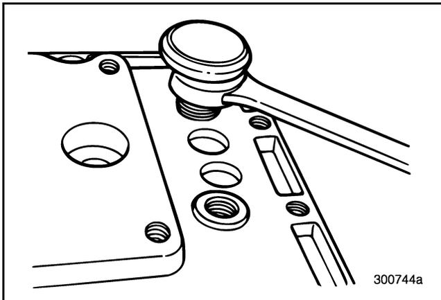
Figure 480 — Installing Breather Vent
