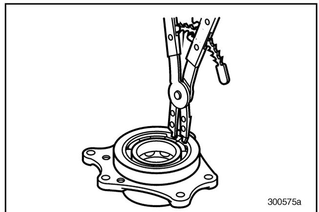
Figure 344 — Installing Snap Ring
