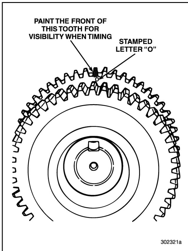
Figure 512 — Gear Tooth Marked for Timing
