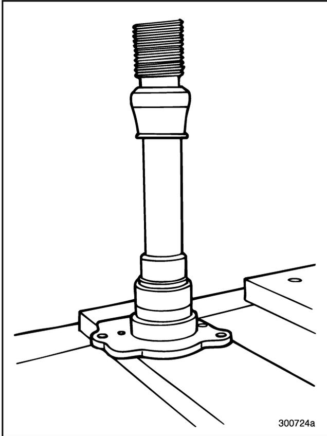
Figure 322 — Pressing Front Bearing Cup into Cover
