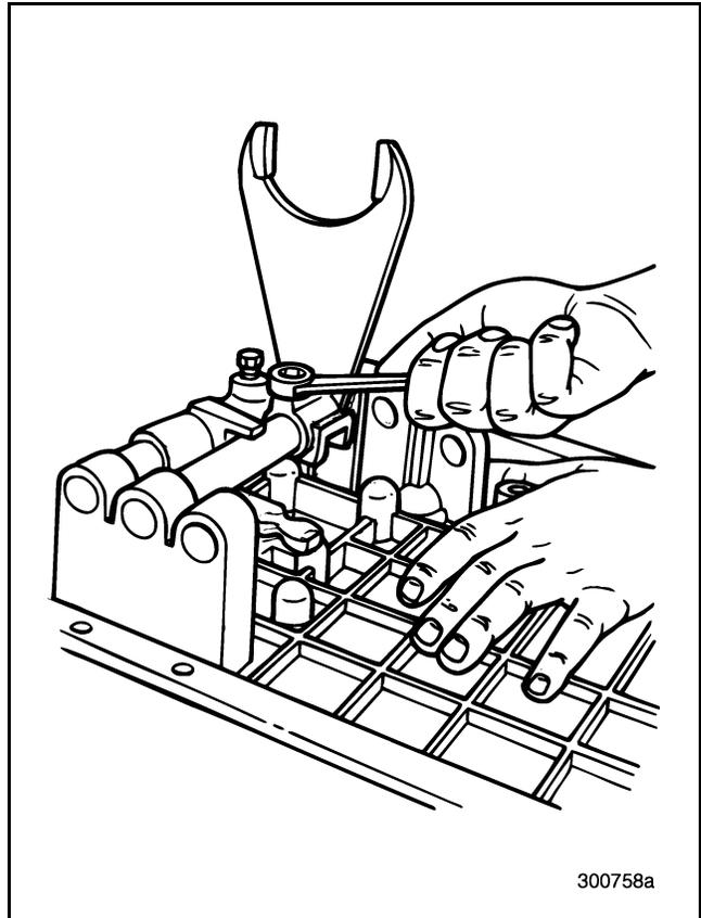
Figure 141 — Removing Setscrew from First/Second Shift Fork
