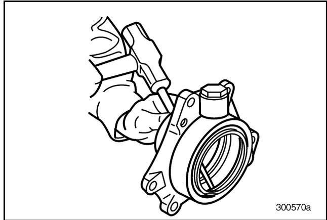
Figure 269 — Using Hammer and Blunt Punch to Remove Oil Seal
