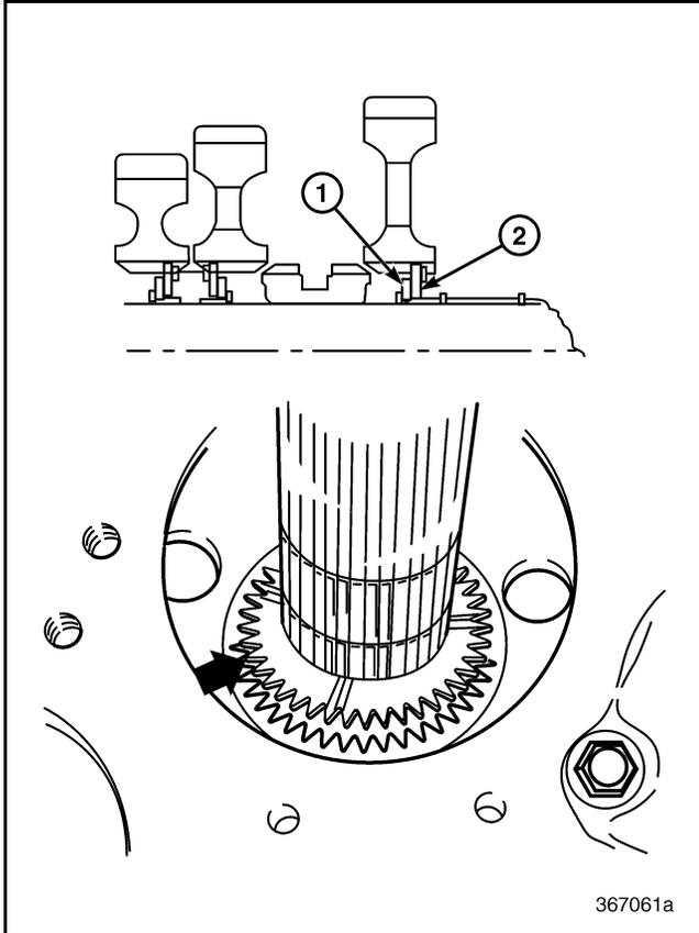
**Figure 107 — Removing External- and Internal-Toothed Thrust Washers**
