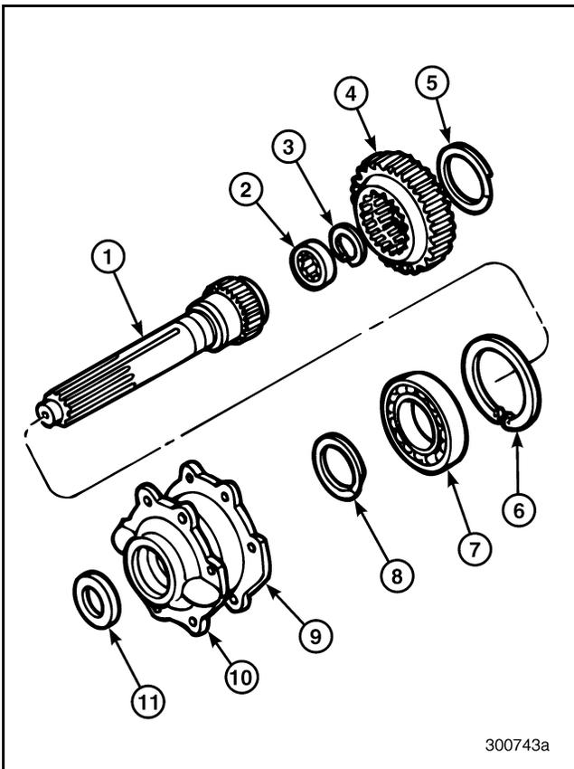
**Figure 596 — Exploded View of Main Drive Pinion**
