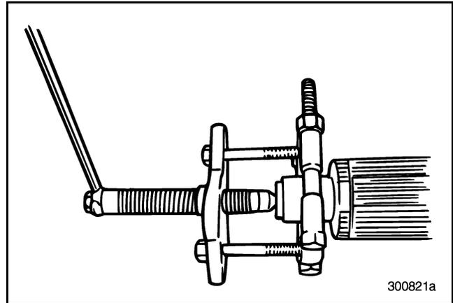
Figure 227 — Removing Rear Spigot Bearing Inner Race (T313L/T318L Shown)
