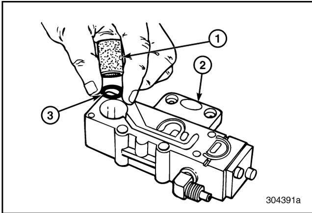
Figure 438 — Installing O-Ring and Filter
