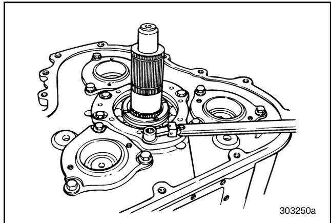
Figure 539 — Installing Front Mainshaft Rear Bearing Cover (T313L/T318L Shown)
