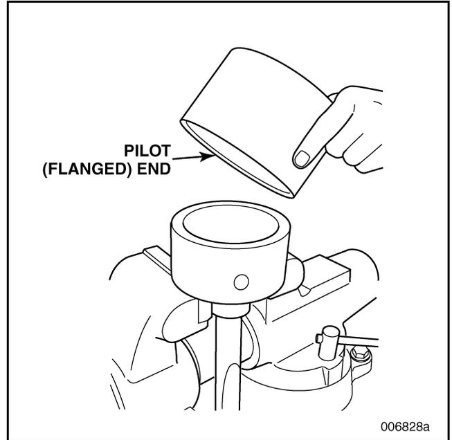
**Figure 456 — Placing Seal Sizer/Piston Installer (Tool No. J 47359) on Cylinder Housing**
