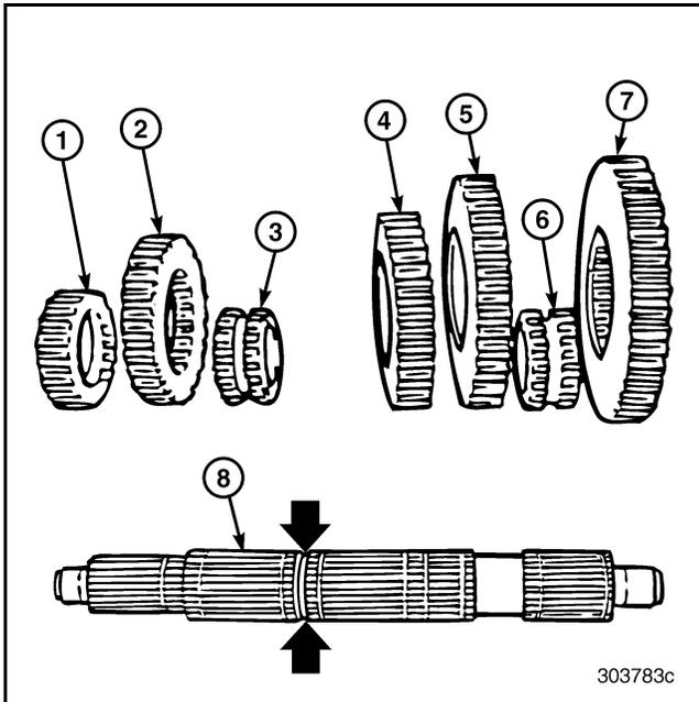
Figure 398 — View of Mainshaft and Gears (T313L/T318L Shown)
