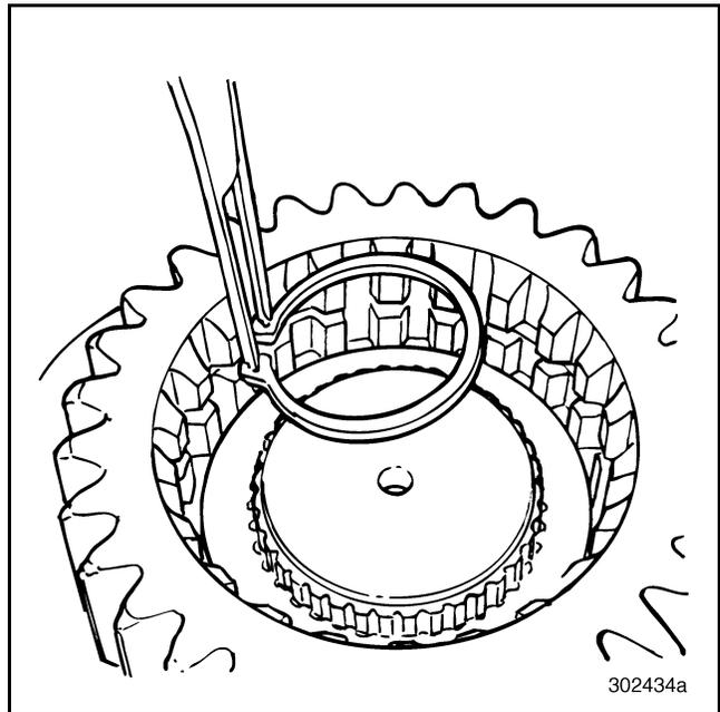
**Figure 394 — Installing Snap Ring onto Front of Shaft (T313L21/T318L21 Shown)**
