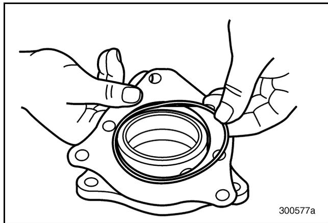
Figure 296 — Removing Cover Shims and O-Ring
