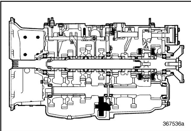
Figure 298 — Reverse Idler Gear Component Locator (T313L/T318L Shown)
