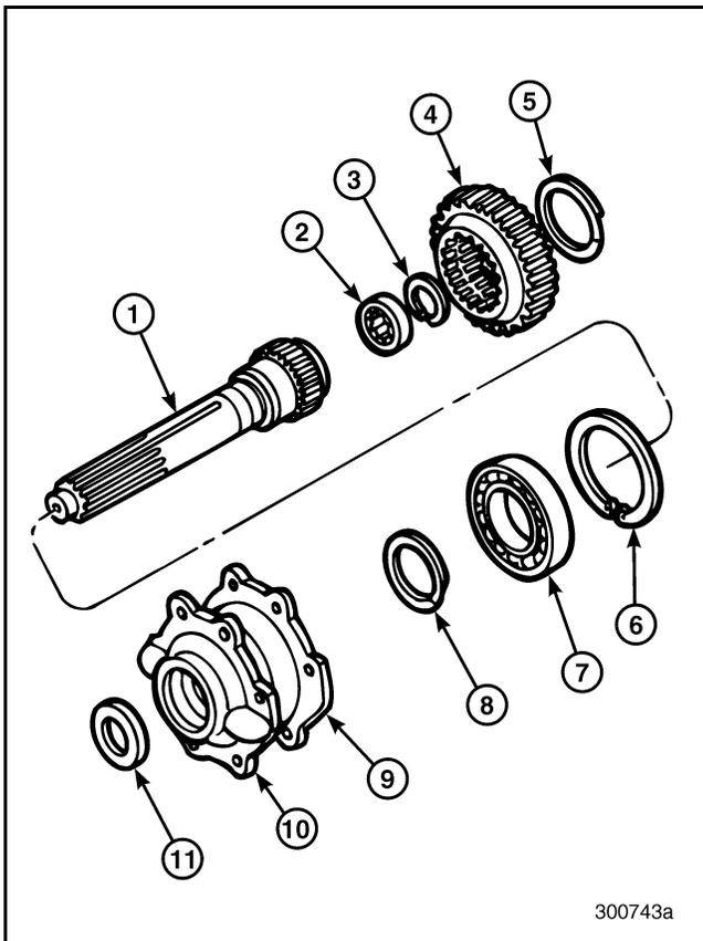
Figure 190 — Exploded View of Main Drive Pinion
