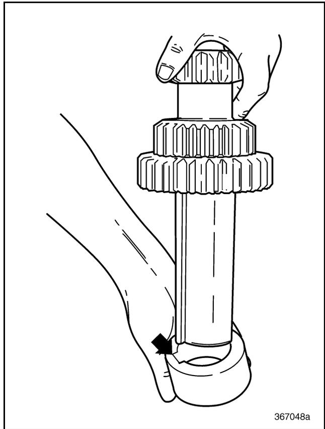
**Figure 329 — Installing First and Second Gear Spacer**
