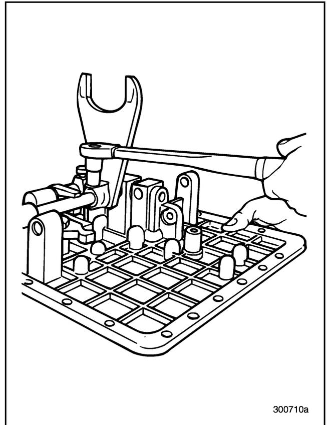
Figure 497 — Tightening Setscrew
