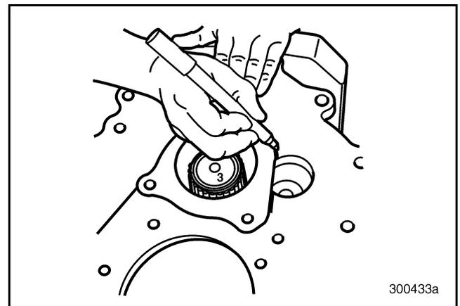
**Figure 516 — Marking Idler Shaft Opening**
