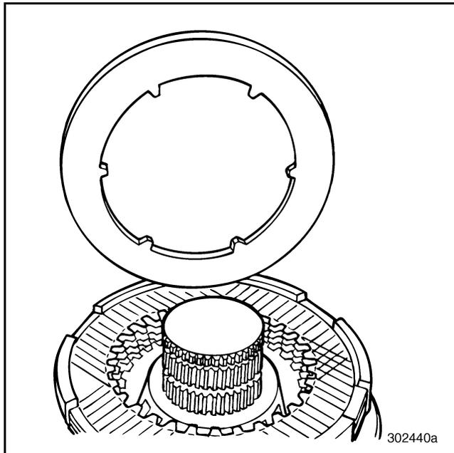
Figure 245 — Removing Spacer from Disc Pack (T313L21/T318L21 Shown)
