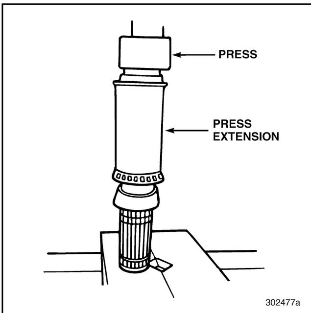
Figure 367 — Pressing Bearing onto Output Shaft
