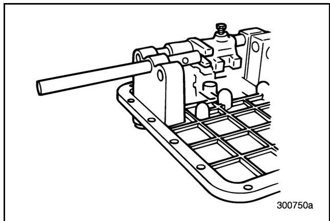
Figure 491 — Installing First/Second Shift Rail
