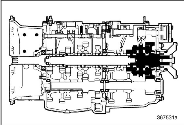
Figure 228 — Rear Mainshaft and Synchronizer Component Locator (T313L/T318L Shown)
