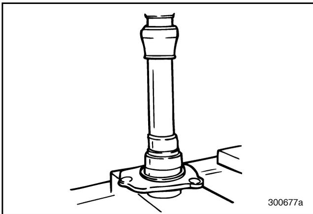
Figure 323 — Pressing Rear Bearing Cup into Cover
