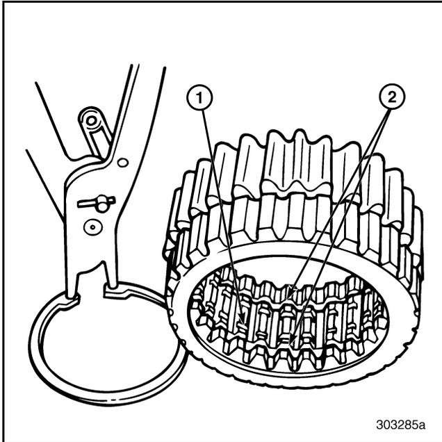
**Figure 383 — Installing Gear Snap Ring
