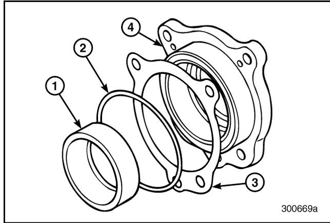
Figure 295 — Exploded View of Rear Countershaft Bearing Cover
