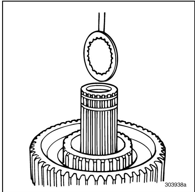
Figure 374 — Installing Internal-Toothed Thrust Washer (T313L/T318L Shown)
