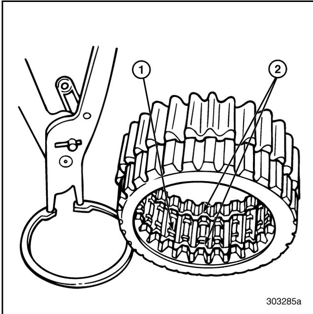
Figure 237 — Removing Remaining Gear Snap Ring (T313L/T318L Shown)
