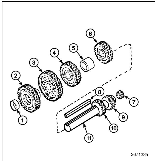
Figure 325 — Exploded View of Front Countershaft
