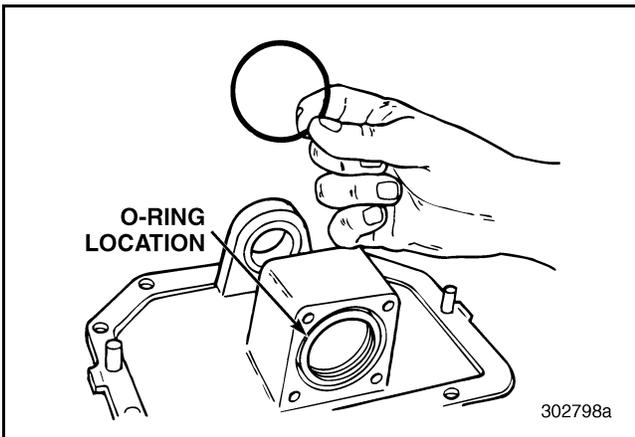
Figure 164 — Removing Piston Cover O-Ring
