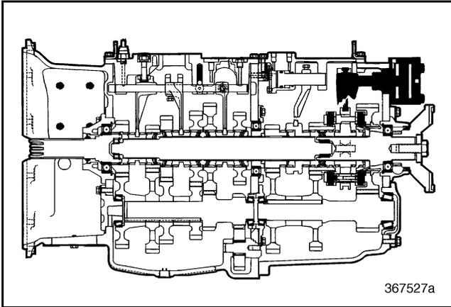
Figure 179 — Range Shift Cylinder Component Locator (T313L/T318L Shown)
