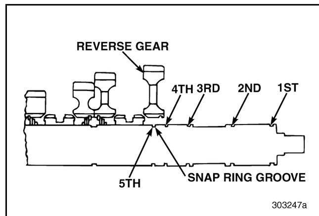
Figure 529 — Installing Reverse Gear Mainshaft Snap Ring (T313L/T318L Shown)
