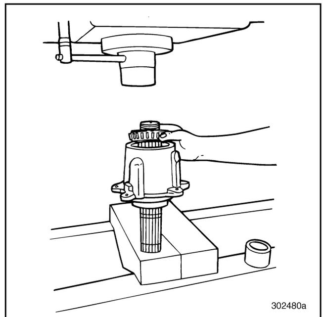
Figure 352 — Positioning Bearing Cone
