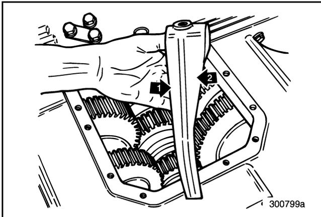
**Figure 569 — Installing Range Shift Fork**
