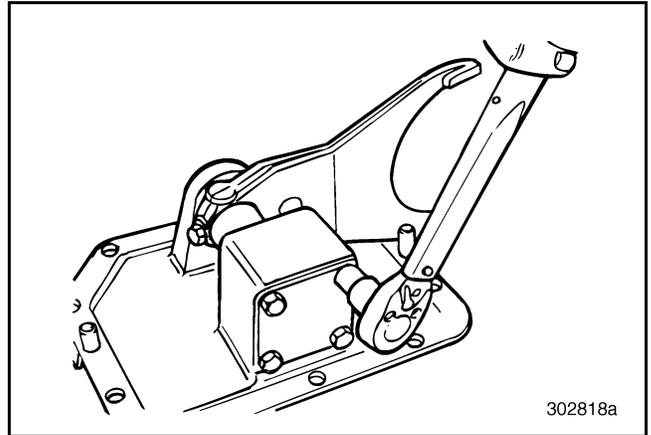
Figure 478 — Installing Piston Cover and Capscrews
