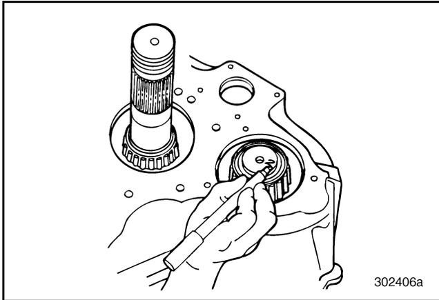
Figure 90 — Marking Rear Countershafts (T313L21/T318L21 Shown)
