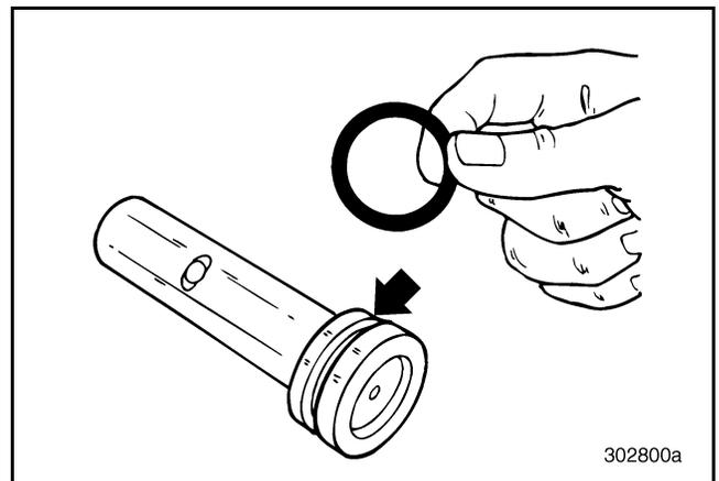
Figure 166 — Removing Piston O-Ring
