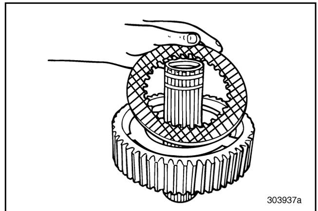
**Figure 251 — Removing Friction Disc (T313L/T318L Shown)**
