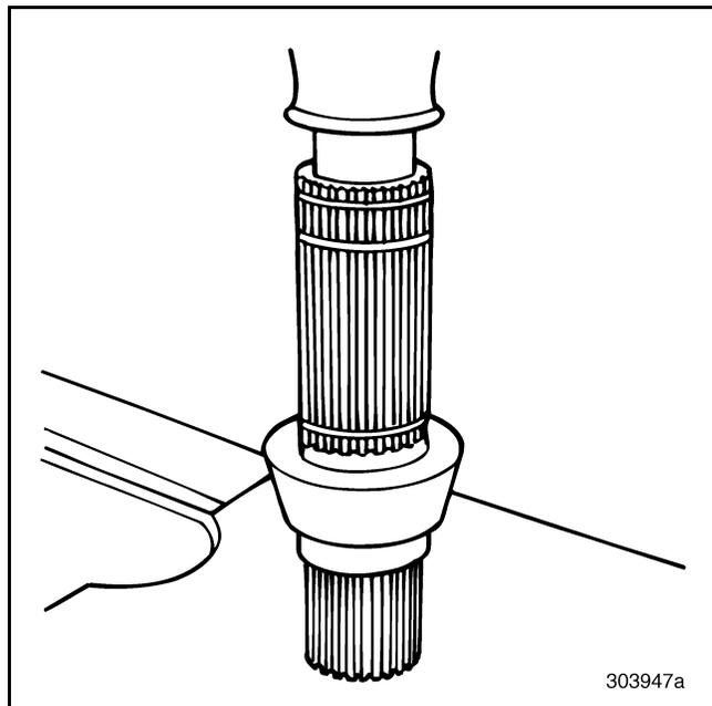
Figure 368 — Installing Spigot Bearing
