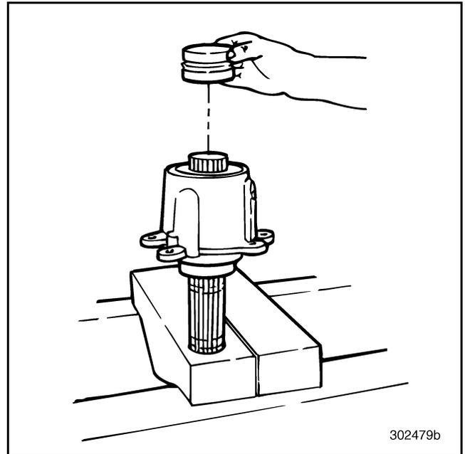
Figure 351 — Installing Spacer
