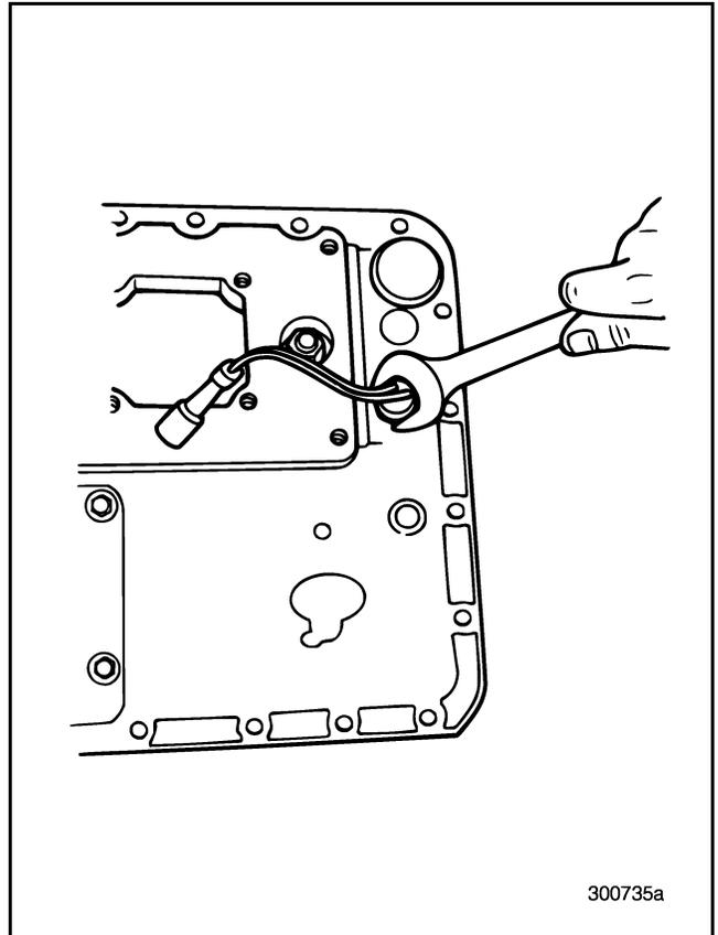
Figure 153 — Removing Reverse Light Switch
