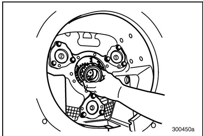
Figure 540 — Installing Sliding Clutch
