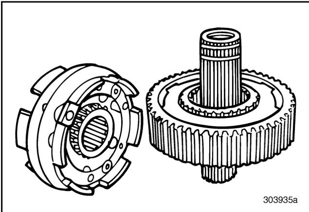
**Figure 249 — Synchronizer Assembly Removed (T313L/T318L Shown)**
