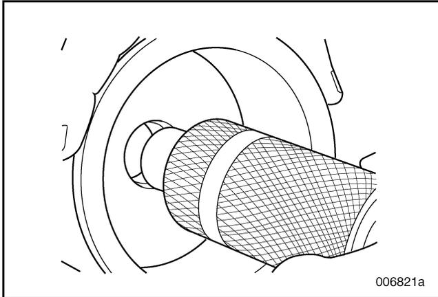
Figure 445 — Positioning Tool in Shift Rail Bore
