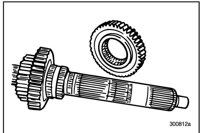
Figure 416 — Installing First Speed Gear onto Mainshaft (T313L/T318L Shown)
