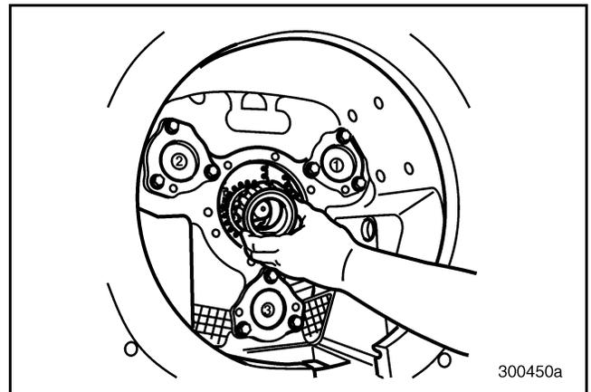
**Figure 113 — Removing Sliding Clutch**
