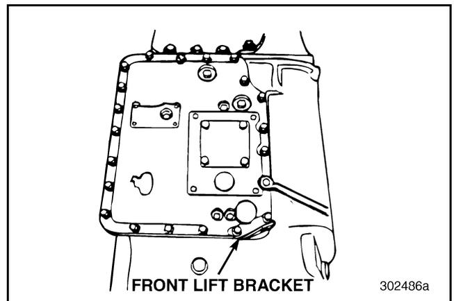
**Figure 65 — Removing Main Case Shift Cover Capscrews**
