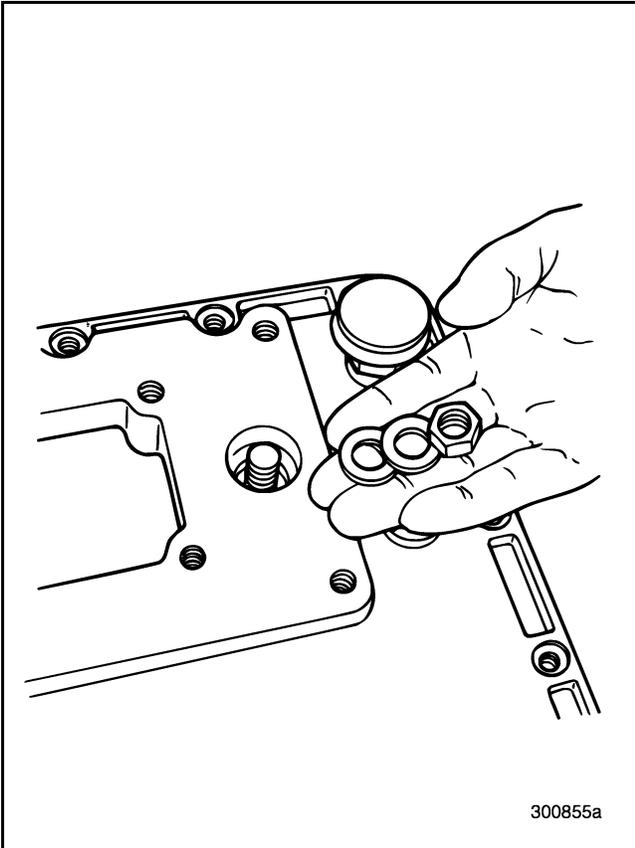
Figure 156 — Recovering the Lock Washer, Flat Washer and Nut
