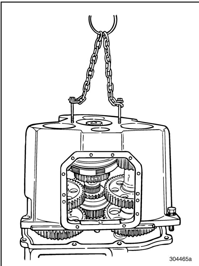
**Figure 94 — Removing Rear Case (T313L/T318L Shown)**
