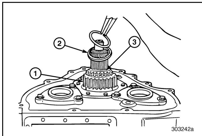
**Figure 548 — Thrust Washer and Snap Ring Location (T313L/T318L Shown)**
