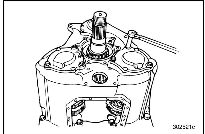
Figure 559 — Tightening Rear Countershaft Bearing Cover Capscrews (T313L21/T318L21 Shown)
