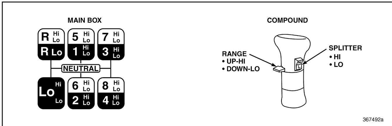
Figure 13 — T318(L)(LR)(21)(L21)(LR21) Shift Pattern
