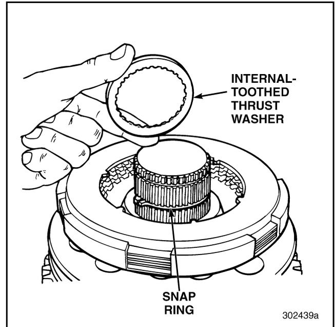
**Figure 389 — Installing Internal-Toothed Thrust Washer (T313L21/T318L21 Shown)**
