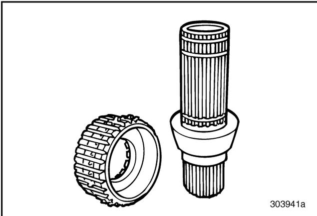
**Figure 256 — Removing Lo-Range Gear Hub from Rear Mainshaft (T313L/T318L Shown)**
