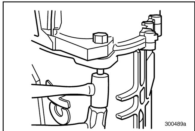
Figure 93 — Removing Dowel Bolts
