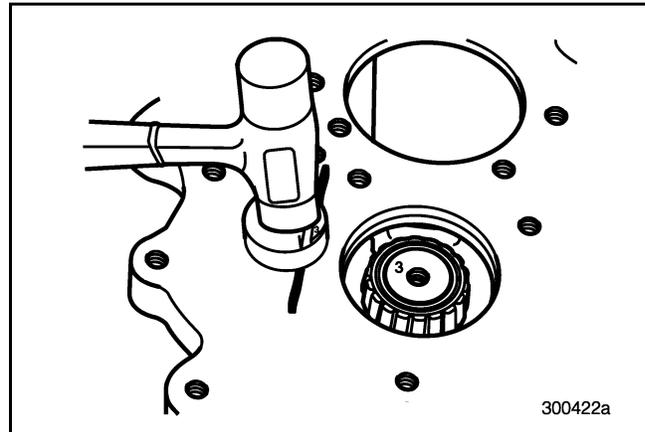
Figure 524 — Tapping Reverse Idler Shaft into Place
