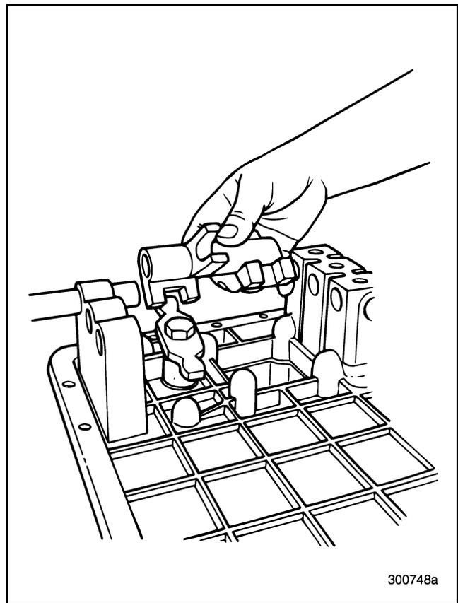
**Figure 150 — Removing Third/Fourth Shifter**
