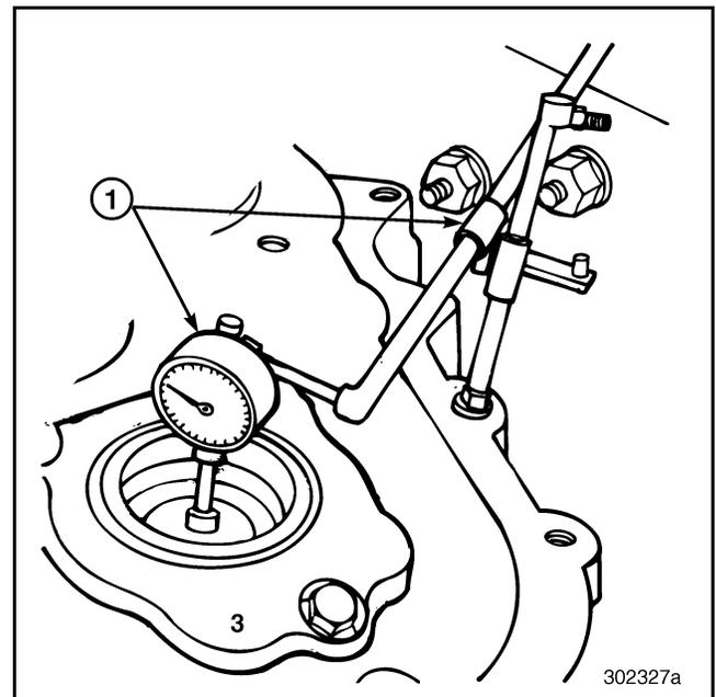
Figure 527 — Measuring Countershaft End Play
