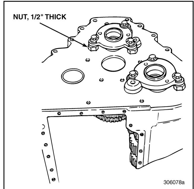
**Figure 521 — Bearing Covers Temporarily Installed with Spacers**
