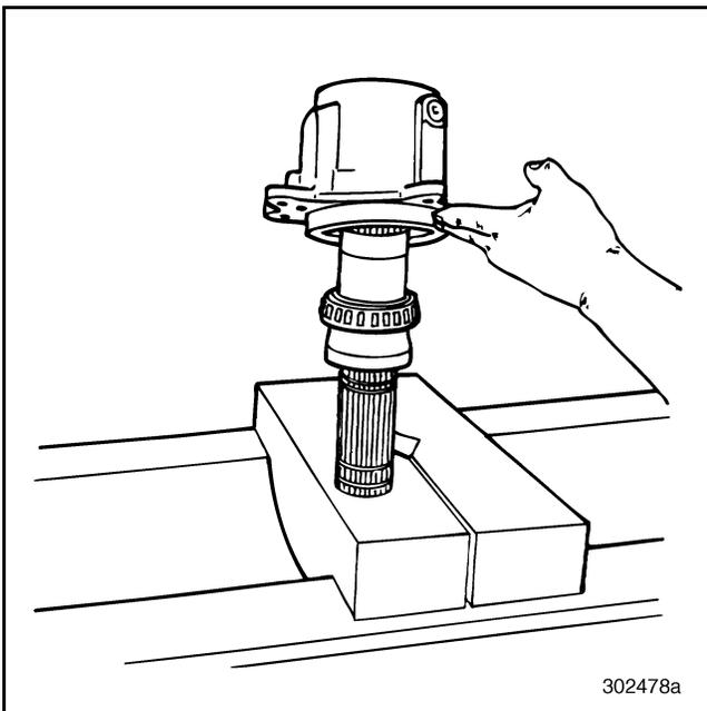
Figure 350 — Positioning Output Housing Over Shaft
