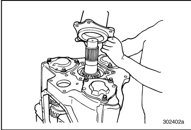
**Figure 561 — Installing Output Housing (T313L21/T318L21 Shown)**
