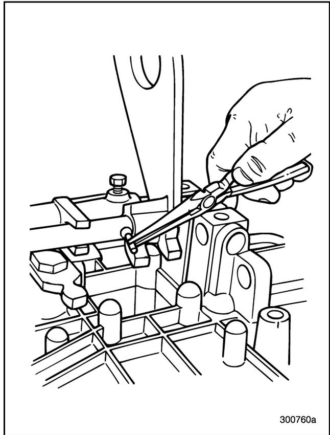
Figure 145 — Removing Interlock Pin
