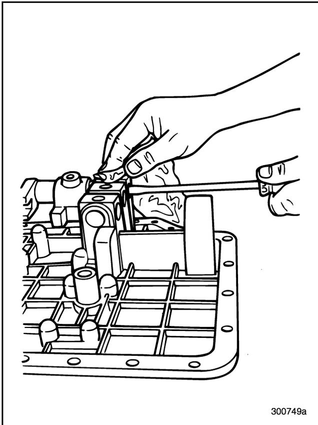
**Figure 149 — Pushing Third/Fourth Shift Rail Forward**
