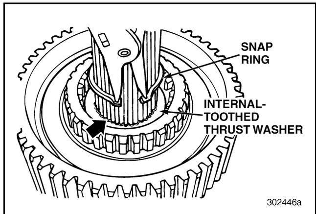
Figure 375 — Installing Lo-Range Gear Hub Shaft Snap Ring
