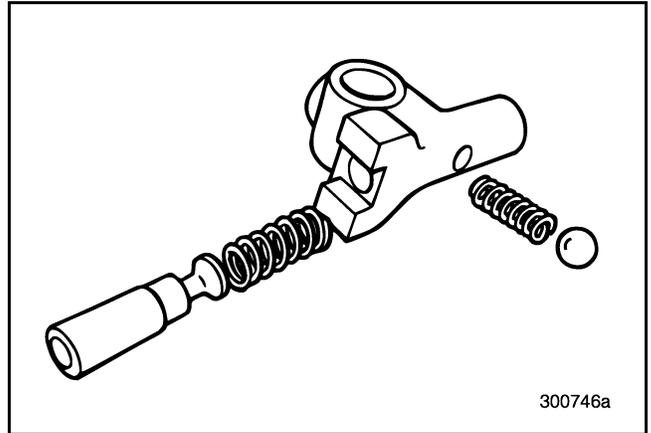
Figure 152 — Lo/Reverse Shifter Disassembled
