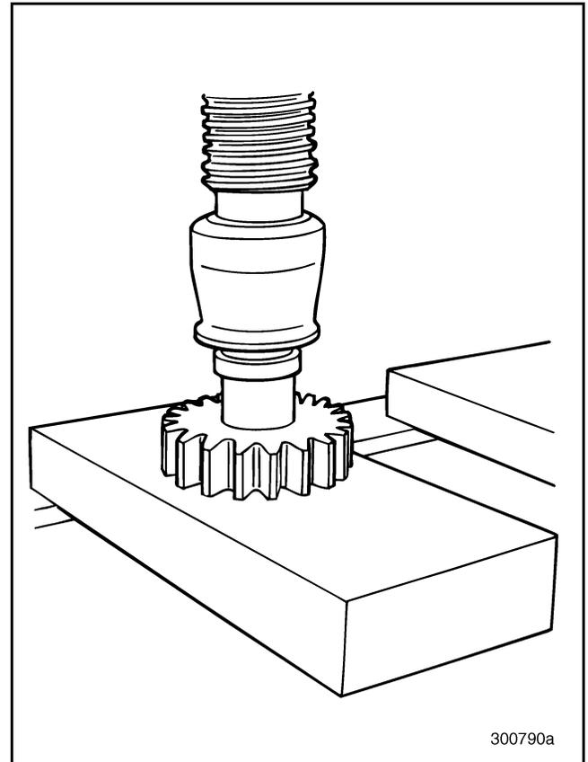
Figure 307 — Pressing Bearing into Gear
