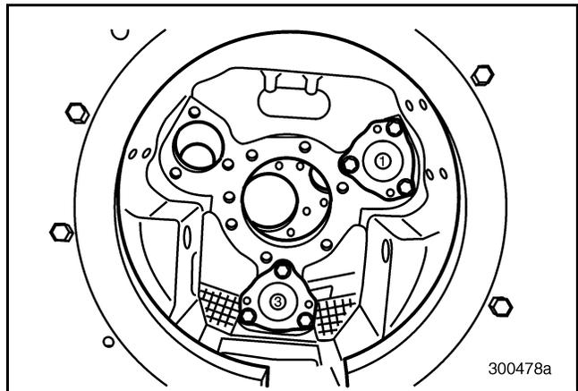
Figure 125 — Remaining No. 1 and No. 3 Front Countershaft Bearing Covers
