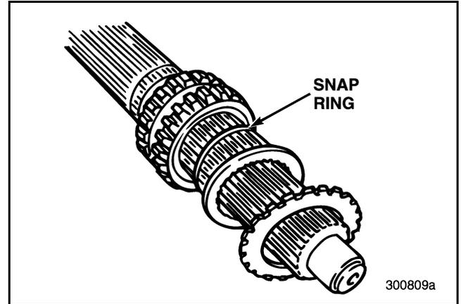
Figure 407 — Installing Internal-Toothed and External-Toothed Thrust Washers
