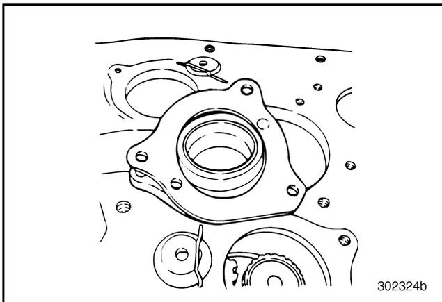
Figure 528 — Installing Shim Pack
