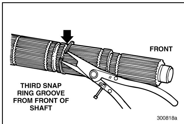
Figure 404 — Installing First Speed Gear Snap Ring
