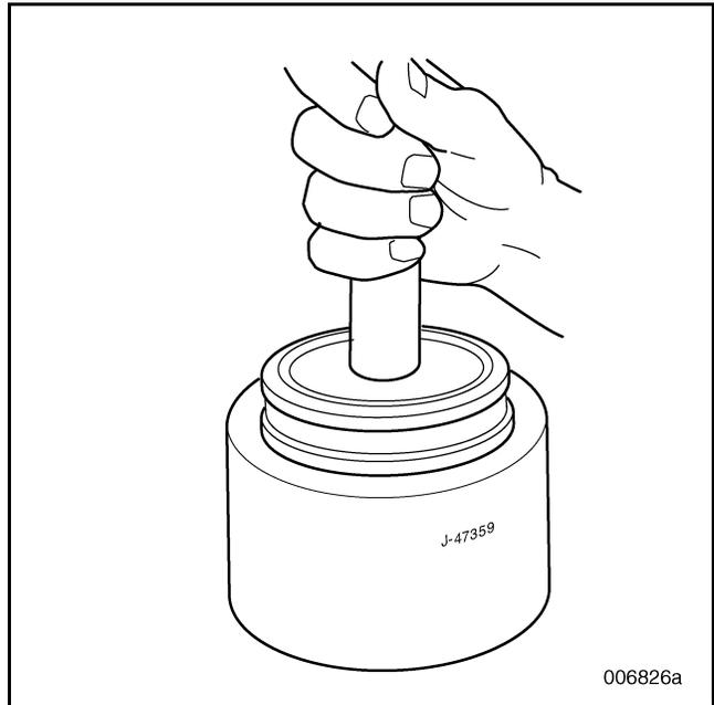
**Figure 454 — Inserting Range Shift Piston into Seal Sizer/Piston Installer (Tool No. J 47359)**
