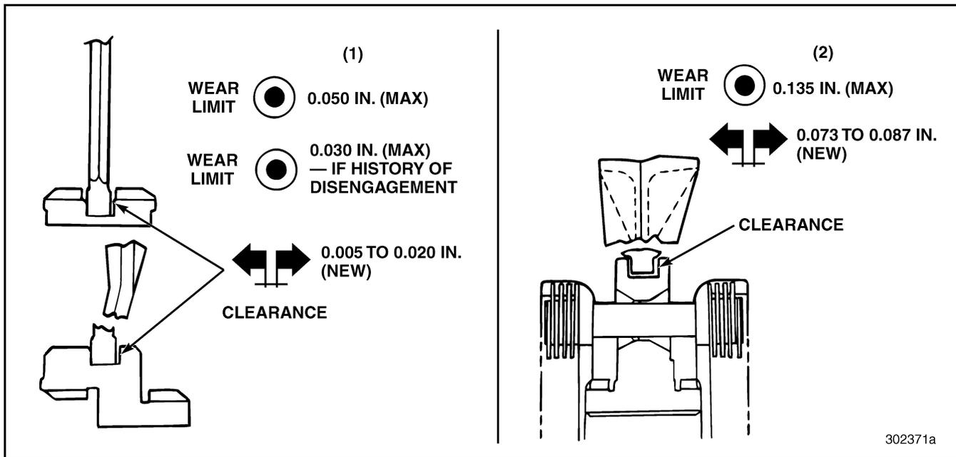
Figure 587 — Sliding Clutch Clearances
