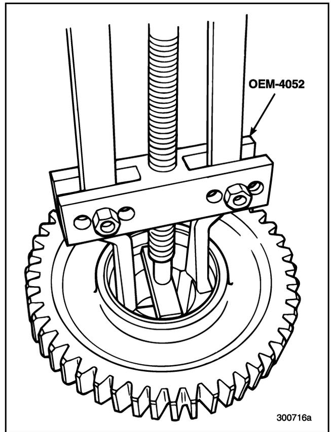
Figure 284 — Removing Bearing Cup from Main Drive Gear
