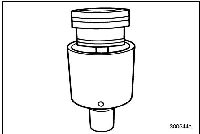
Figure 169 — Piston Assembly Partially Removed
