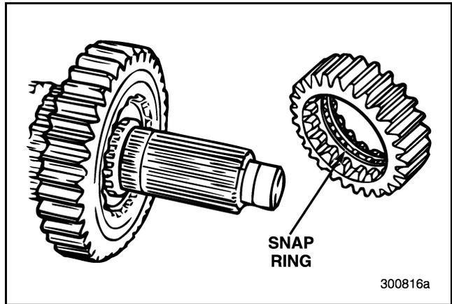
Figure 411 — Installing Fourth Speed Gear
