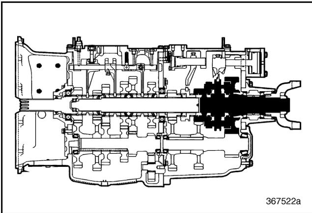
Figure 229 — Rear Mainshaft (Output Shaft) and Synchronizer Component Locator (T313L21/T318L21 Shown)
