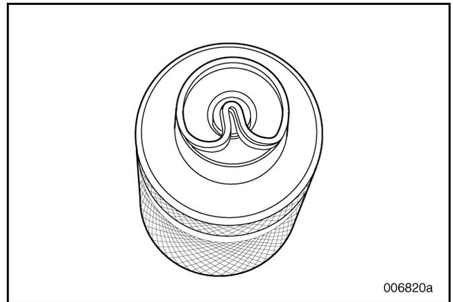
Figure 444 — Inserting Teflon® Seal in Nose of Insertion Tool (Tool No. J 47357)
