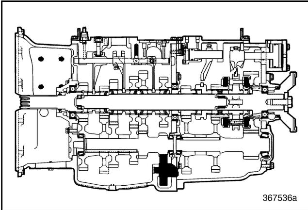
Figure 305 — Reverse Idler Gear Component Locator (T313L/T318L Shown)
