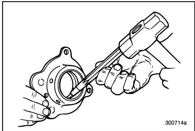
Figure 288 — Removing Rear Bearing Cup
