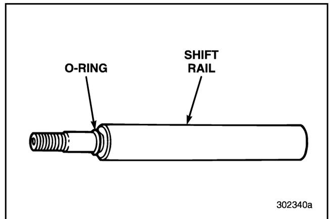
Figure 463 — Installing Shift Rail O-Ring
