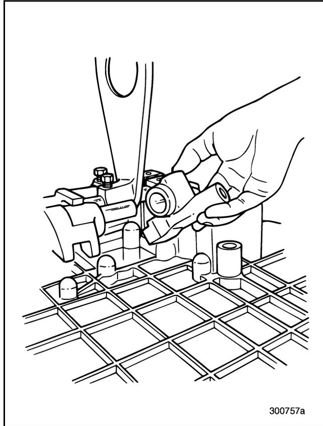
Figure 500 — Installing Lo/Reverse Shifter
