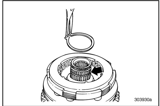
Figure 382 — Installing Shaft Snap Ring (T313L/T318L Shown)
