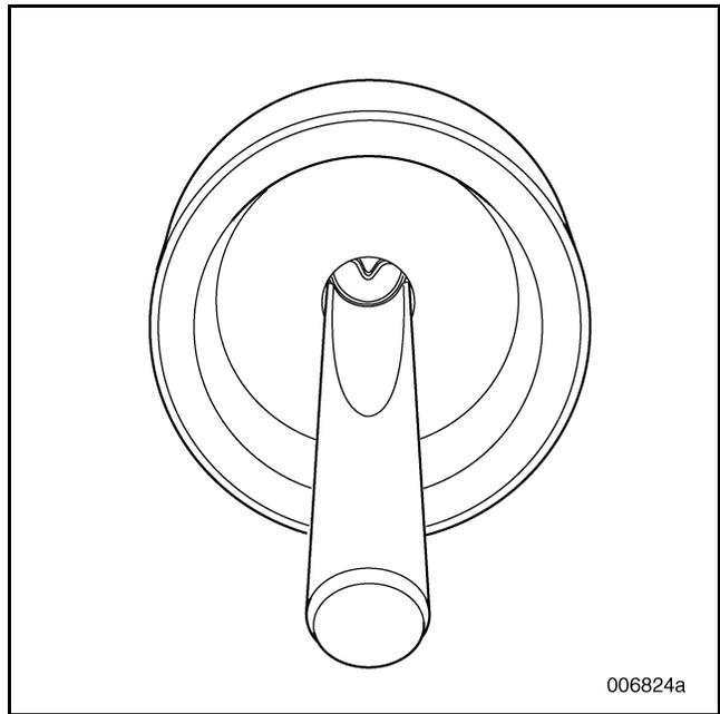
Figure 448 — Inserting Teflon® Seal Installer/Sizer (Tool No. J 47358)
