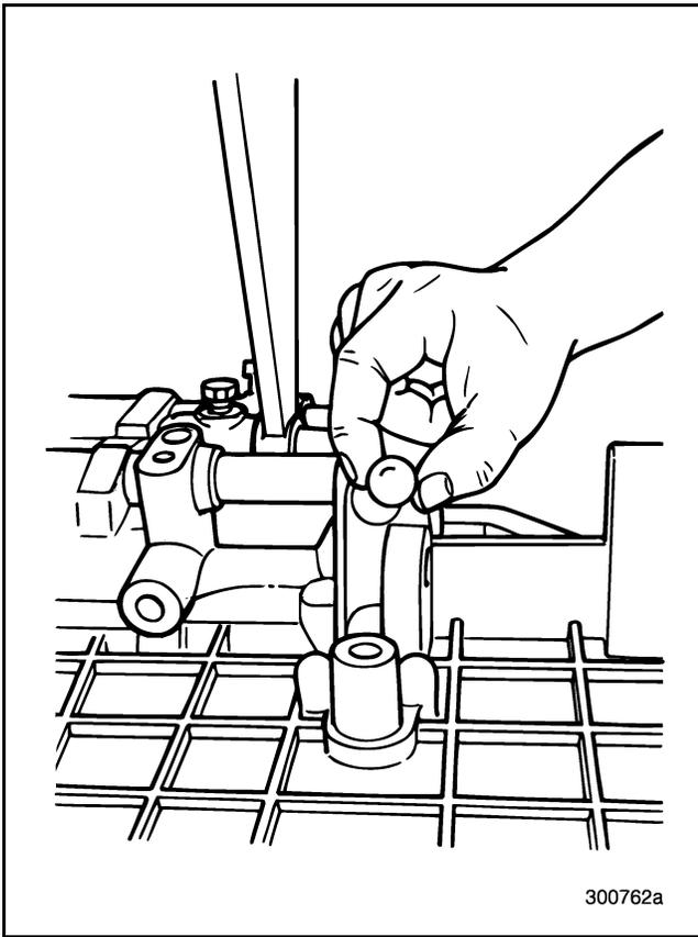
Figure 138 — Removing Interlock Ball
