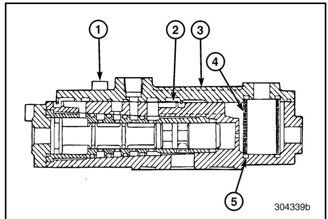
Figure 437 — Cutaway View of Range Shift Valve Assembly
