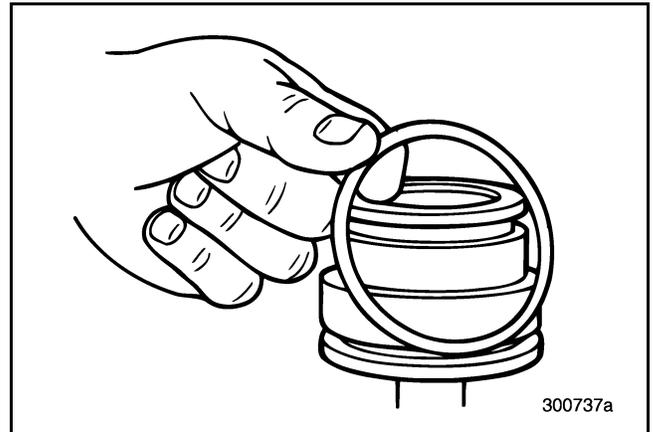
Figure 174 — Removing O-Ring from Front of Piston
