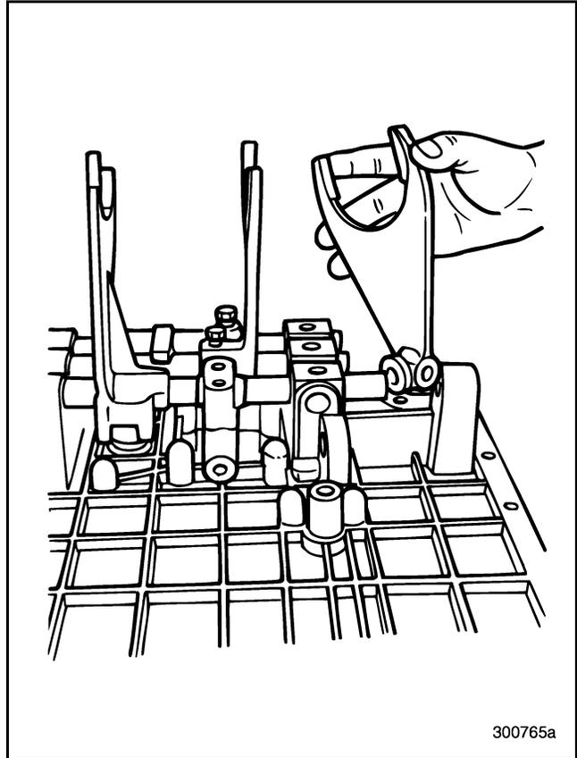
Figure 504 — Installing Lo/Reverse Shift Fork
