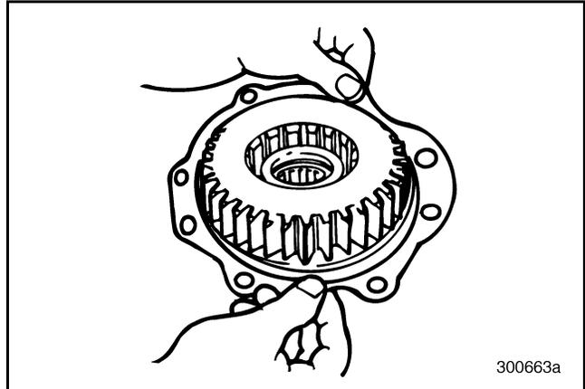
Figure 191 — Removing Gasket from Main Drive Pinion Bearing Cover
