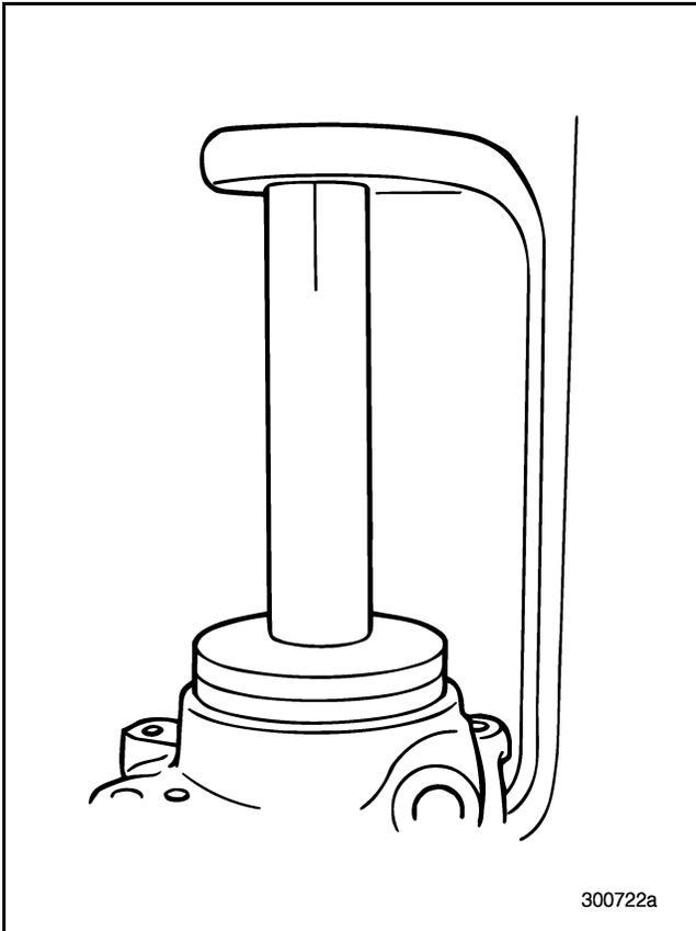
Figure 341 — Pressing Oil Seal into Rear Mainshaft Bearing Cover
