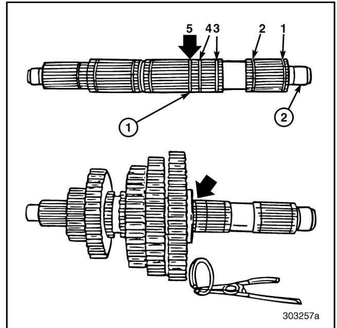
Figure 423 — Installing Reverse Speed Gear Snap Ring onto Mainshaft (T313L/T318L Shown)
