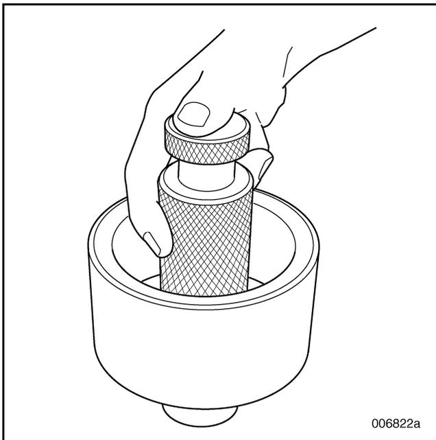
Figure 446 — Installing Teflon® Seal
