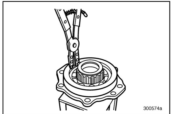
Figure 196 — Removing Main Drive Pinion Cover Bearing Snap Ring
