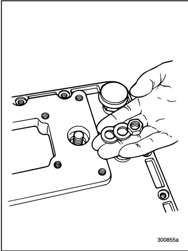
Figure 483 — Installing Washers and Nut
