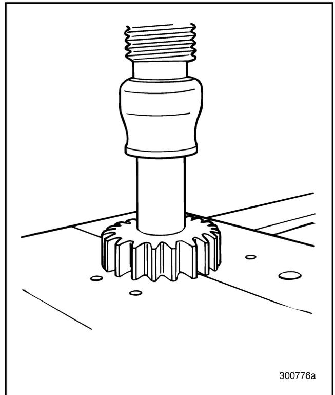
Figure 300 — Pressing out Reverse Idler Gear Bearing
