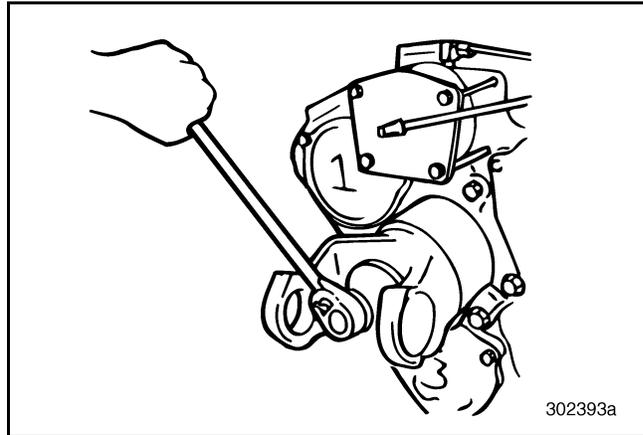
Figure 68 — Removing Drive Yoke Nut (T313L21/T318L21 Shown)
