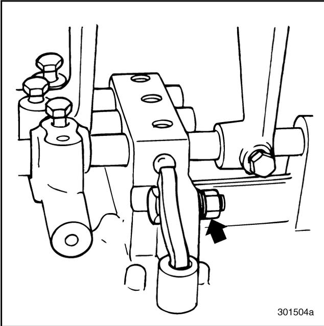
Figure 129 — Remove Nut and Washers
