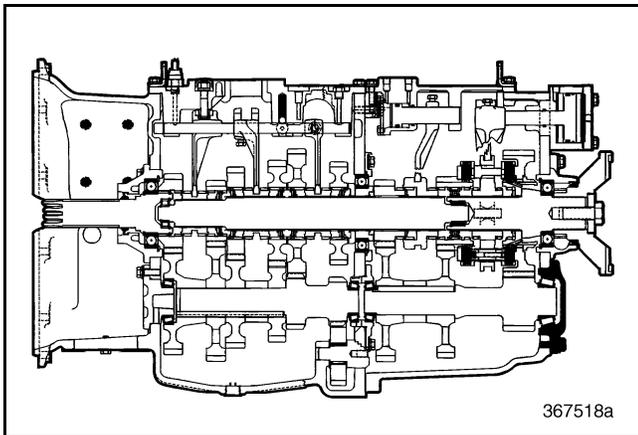
Figure 309 — Rear Countershaft Bearing Cover Component Locator (T313L/T318L Shown)
