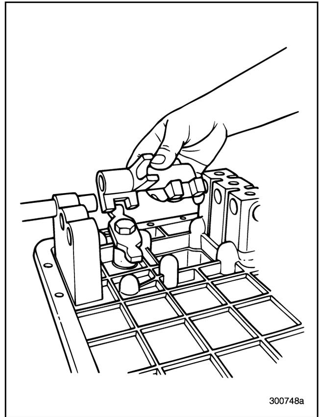
Figure 488 — Installing Shift Rail and Shifter
