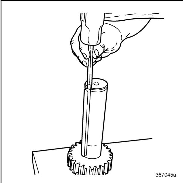
Figure 283 — Removing Key
