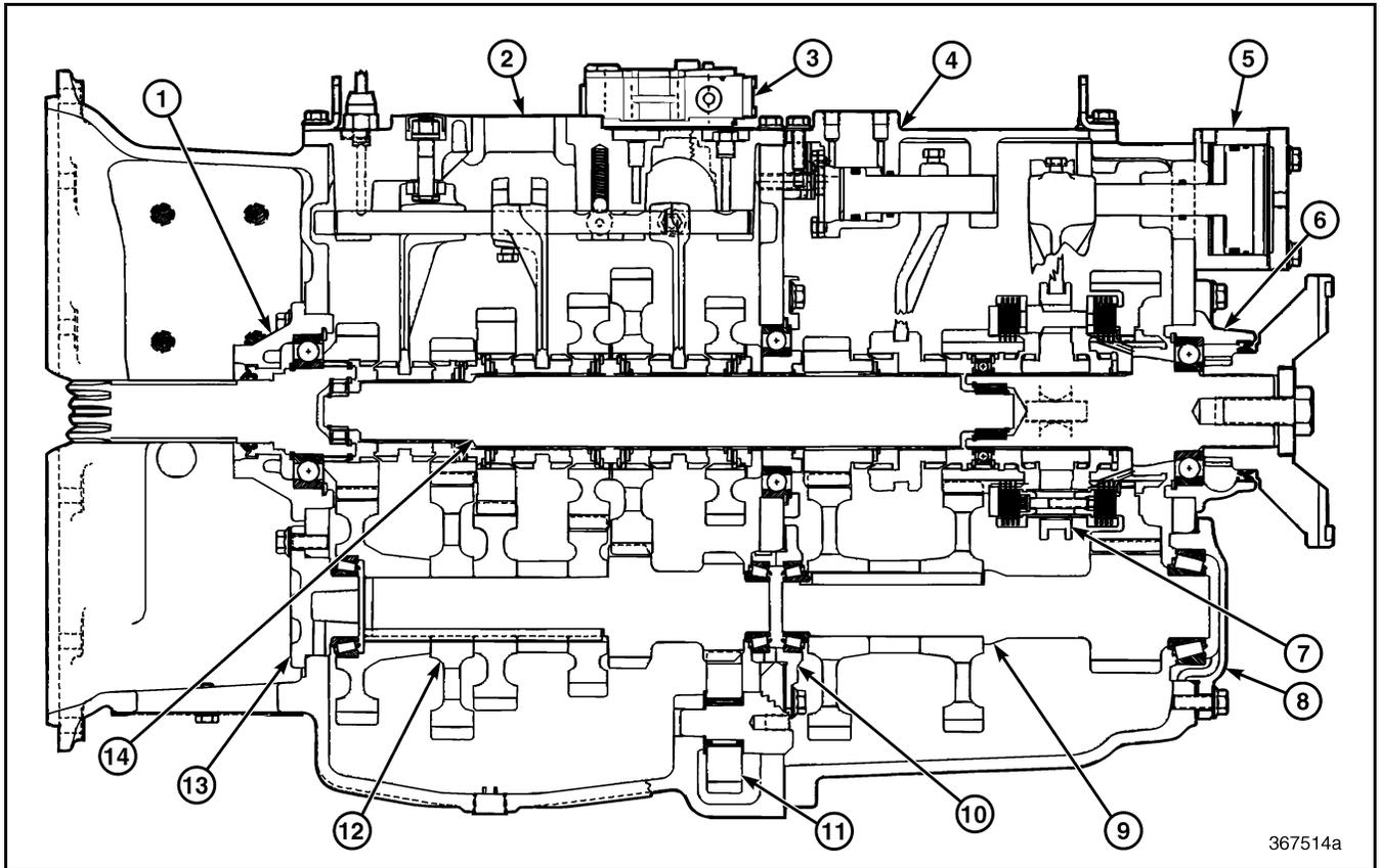
Figure 51 — Major Component Locations for T313L/T318L Transmission
