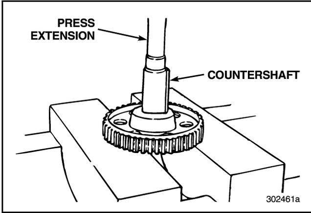
Figure 293 — Pressing off Hi-Range/Hi-Split Gear
