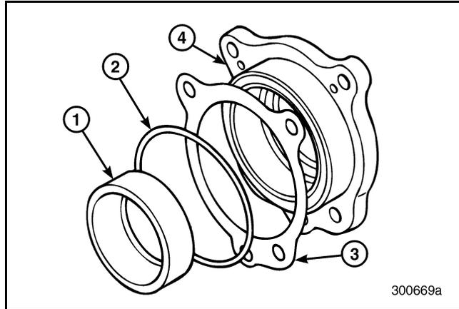
Figure 310 — Exploded View of Rear Countershaft Bearing Cover
