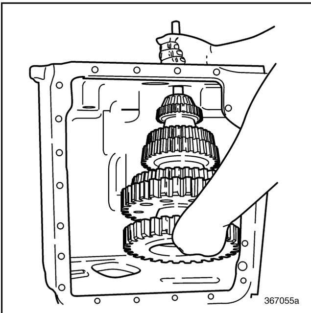
**Figure 515 — Installing Lower No. 3 Countershaft into Main Case**
