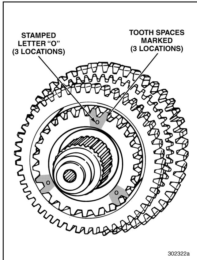
Figure 513 — Gear Tooth Spaces Marked for Timing
