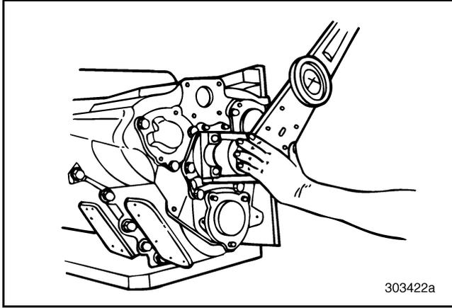
**Figure 568 — Tightening Clamp Plate Capscrew (T313LR/T318LR Shown)**
