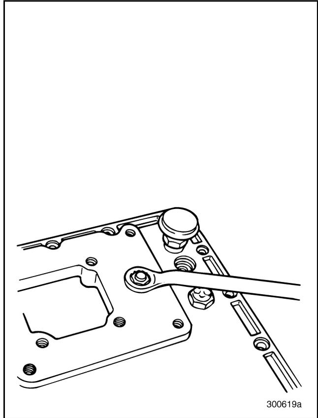
Figure 155 — Loosening Third/Fourth Rocker Pin Nut
