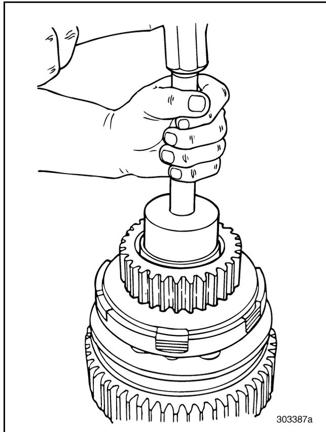
**Figure 386 — Installing Ball Bearing
