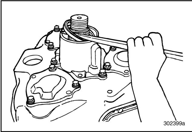
**Figure 78 — Removing Output Housing Oil Seal for T313L21/T318L21 Series**
