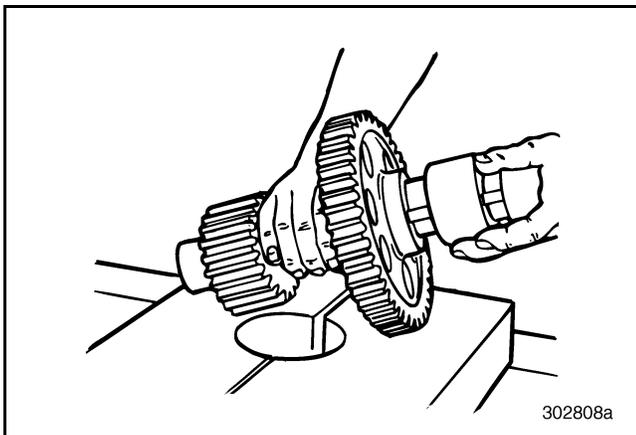
Figure 316 — Installing Spacer
