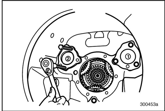
Figure 116 — Removing No. 2 Front Countershaft Front Bearing Cover
