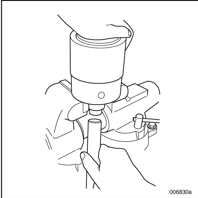
Figure 458 — Installing Piston into Range Shift Cylinder Housing
