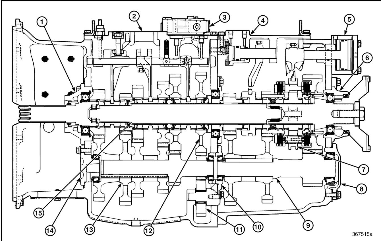
**Figure 52 — Major Component Locations for T313LR/T318LR Transmission**
