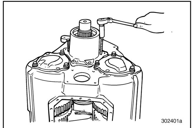
**Figure 80 — Separating Output Housing from Case (T313L21/T318L21 Shown)**
