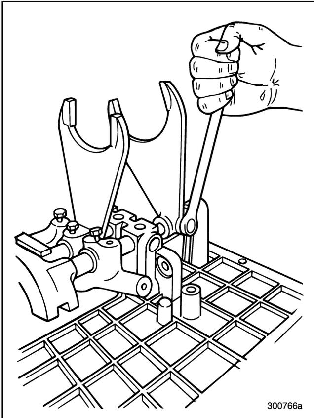
Figure 132 — Removing Setscrew from Lo/Reverse Shift Fork
