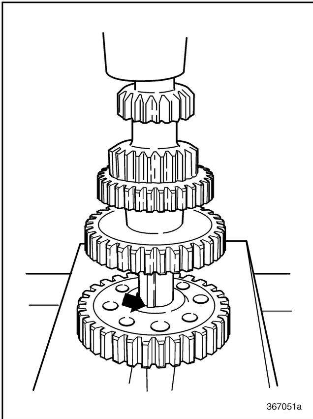
Figure 332 — Installing Fourth (Eighth) Speed Gear
