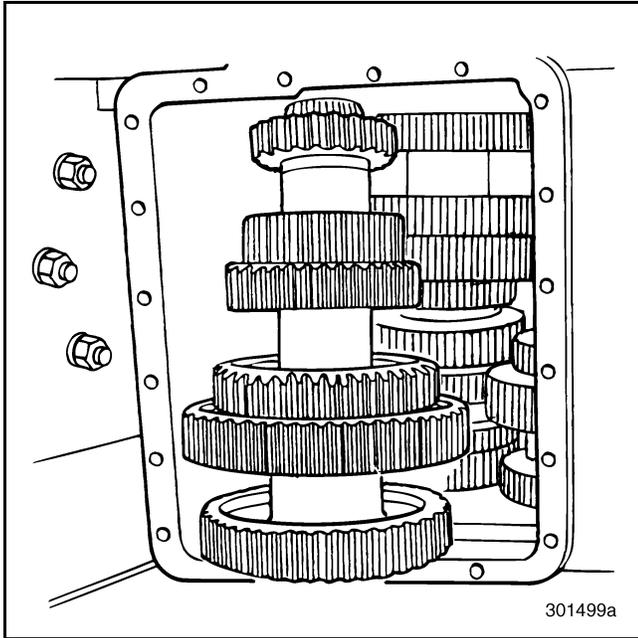
Figure 114 — Removing No. 2 Countershaft from Transmission Case
