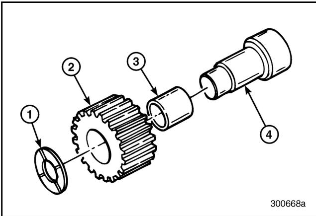
Figure 306 — Exploded View of Reverse Idler Gear Assembly
