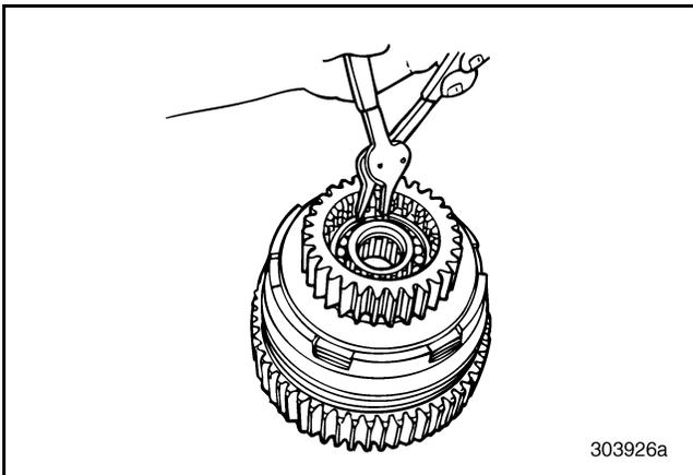
**Figure 388 — Installing Gear Snap Ring (T313L/T318L Shown)**
