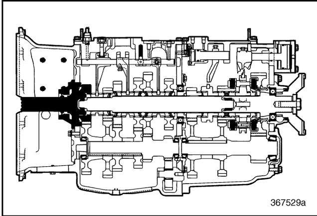
Figure 189 — Main Drive Pinion Component Locator (T313L/T318L Shown)
