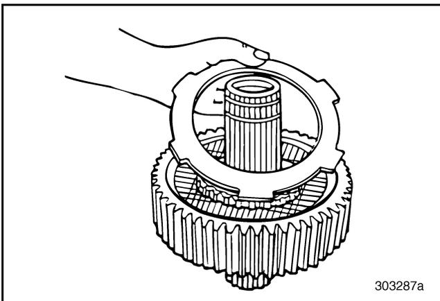
Figure 377 — Installing Reaction Disc
