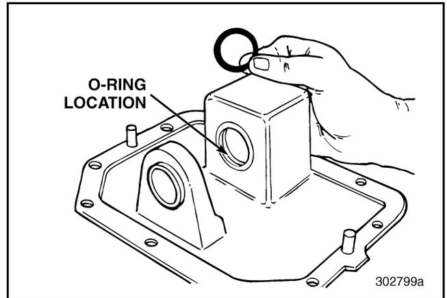
Figure 165 — Removing O-Ring from Rear of Housing
