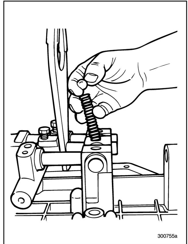
Figure 502 — Installing Poppet Ball and Spring
