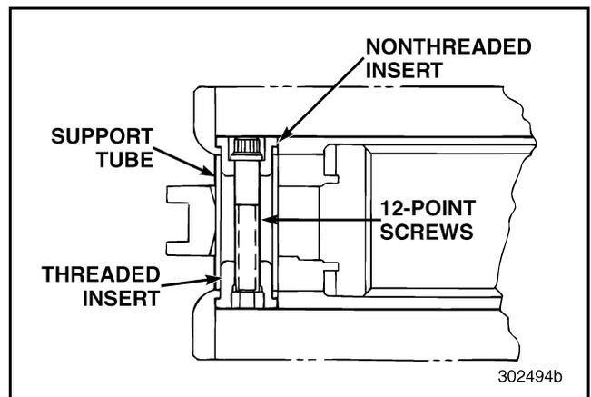
**Figure 365 — Installing 12-Point Screws and Inserts**
