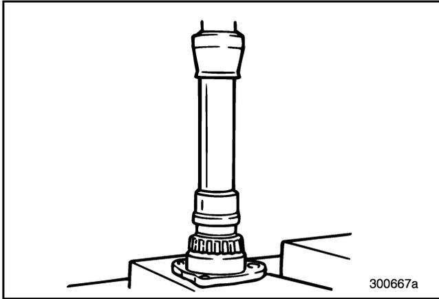
Figure 337 — Pressing Bearing Cone onto Cover
