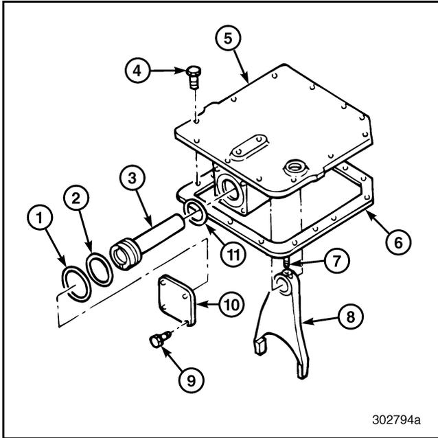
**Figure 606 — Exploded View of Rear Case Shift Cover**
