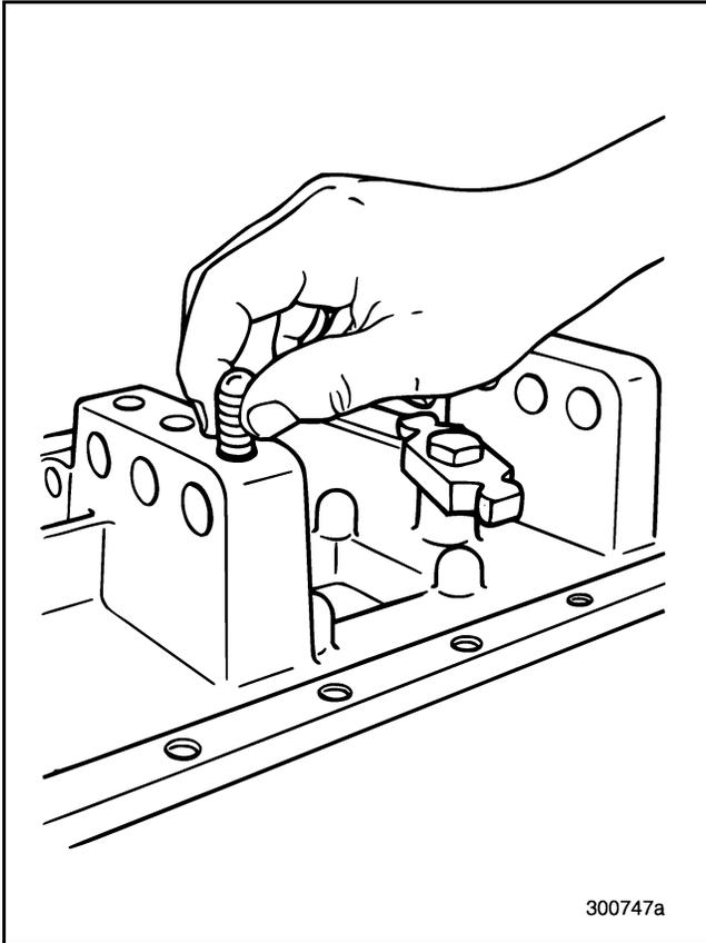
Figure 487 — Installing Poppet Ball and Spring
