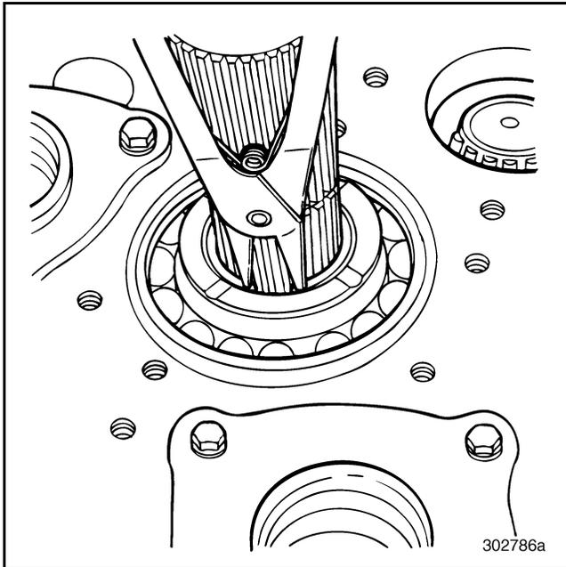
Figure 538 — Installing Snap Ring
