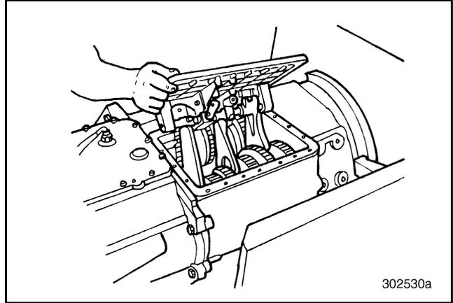
Figure 575 — Installing Main Case Shift Cover Assembly
