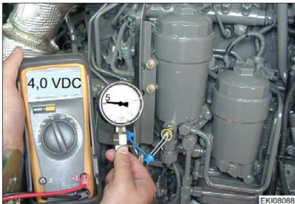
Connect pressure gauge on measuring point
