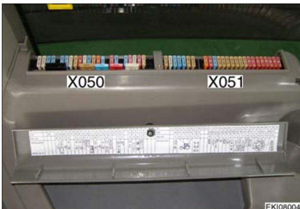
X050 = Fuse holder 1 compl X051 = Fuse holder 2 compl At right rear in cab
