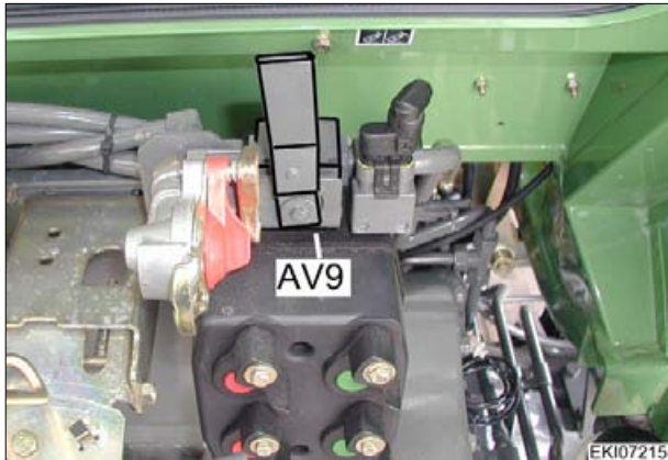
AV9 = Stopcock EPC lock "rigid drawbar" At rear of tractor
