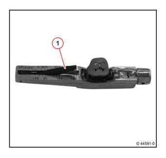
• Mount V-belt tension measuring device on V-belt.
