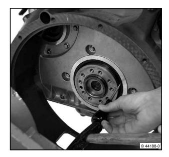
• Turn in a self-tapping screw with washer.
