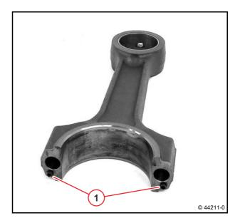
• Insert bearing shell in the con rod.
