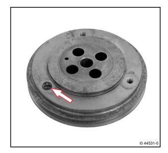
• Fix the tooth lock washer with the largest hole (1) to the V-belt pulley with clamping bushing (2).
