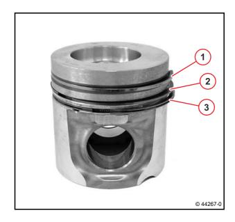
• Install piston rings with universal piston ring pliers.
