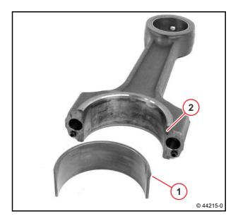
• Insert bearing shell in the respective big end bearing cap.
