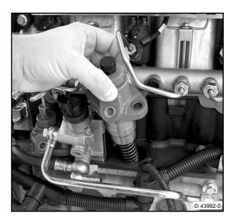
• Oil the screws (1) lightly and tighten alternately until the high-pressure pump is flush with the crankcase.
