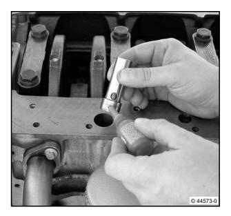
• Insert new pressure holding valve in the crankcase.
