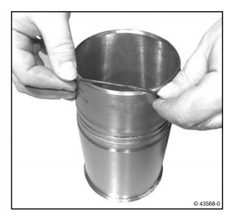
• Coat the crankcase and the cylinder liner in area (X) with lubricating oil.
