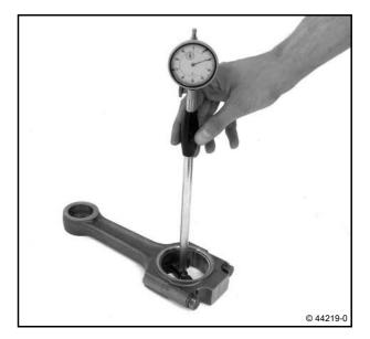
• Checking the diameter of the lifting journals.
