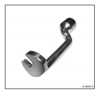
103220 Special pliers for removing the roller tappet
