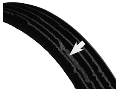
UNEVEN RIB WEAR
