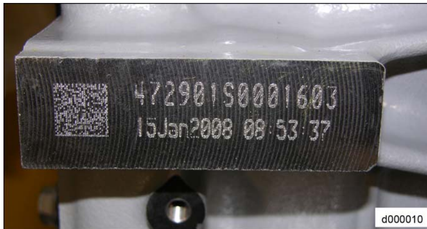
Figure 3-6 The Engine Serial Numbers Stamp and Model Number, DD Platform
