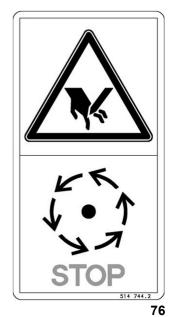
Touch machine parts only after they have come to a complete standstill.
