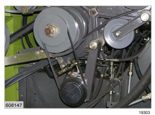
When the desired temperature is reached, a thermostat switch in conjunction with an electro-magnetic clutch disengages the compressor.
