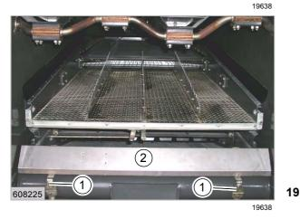
Removing the lower sieves
