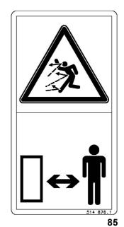
Danger - flying objects; keep safe distance from the machine as long as the engine is running.
