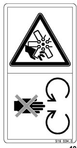
19 Do not open or remove safety shields while engine is
