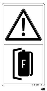
Do not operate machine unless an approved fire extinguisher is installed.
