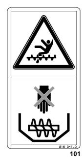
Never reach or climb into grain tank while engine is running.
