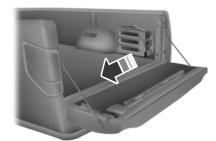
1. Pull the locking pin toward the center of the vehicle.
