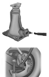
5. Insert the hooked end of the jack handle into the jack and use the handle to slide the jack under the vehicle.
