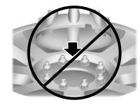
If the ornament retention towers are aligned between the studs or lug nuts, the ornament is improperly installed. This improper installation may appear and sound correct, but will not keep the ornament on the vehicle. Ornaments improperly installed in this manner will fall off or become loose with minimal force or impact.
