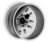
Inspect the wheel pilot hole and mounting surface prior to installation. Remove any visible corrosion or loose particles.
