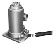
11. Slide the notched end of the jack handle over the release valve and use the handle to slide the jack under the vehicle. Make sure the valve is closed by turning it clockwise.
