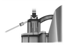
10. Reconnect the mass air flow sensor electrical connector to the outlet tube. Make sure the locking tab on the connector is in the "locked" position (connector shown from below for clarity).
