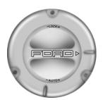
For proper operation, make sure that each hub is fully engaged and that both hub locks are set to the same position (both set to LOCK or both set to AUTO). To engage LOCK, turn the hub locks completely clockwise; to engage AUTO, turn the hub locks completely counterclockwise.
