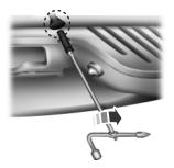
3. Fully insert the jack handle (with one extension) through the bumper hole and into the guide tube. The key and lock will engage with a slight push and counterclockwise turn. Some resistance will be felt when turning the jack handle assembly.
