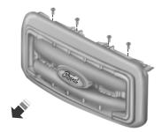
2. Using masking tape or a marker, make an alignment mark between one of the grille brackets and the vehicle radiator support to ensure correct grille alignment during the installation procedure. Do not scratch the black coating from the radiator support.
