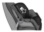
5. To put the retractor in the automatic locking mode, grasp the shoulder portion of the belt and pull downward until all of the belt is pulled out.
