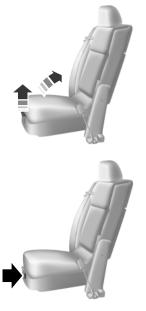
To gain access to the under-seat storage compartment (if equipped) in your seat cushion, lift the latch to open the lid. The lid cannot be opened when the armrest is down.
