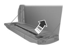
3. Raise the handle upright until you feel it latch and see the latch lever in the lock position. The yellow lever only needs to be used when releasing the grab handle.
