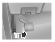
1. Inside the vehicle, pull the hood release handle located under the bottom left corner of the instrument panel.
