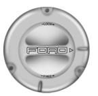
The 4WD system is engaged or disengaged by rotating the control for both front wheel hub locks from the FREE or LOCK position, then manually engaging or disengaging the transfer case with the floor-mounted shifter. For increased fuel economy in 2WD, rotate both hub locks to the FREE position.
