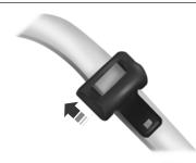
1. To lengthen the lap belt, pull some webbing out of the shoulder belt retractor.
