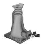
7. Turn the jack handle clockwise until the wheel is completely off the ground and high enough to install the spare tire.
