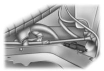
1. Before removal of the tailgate, locate and disconnect the tailgate in-line connector under the pickup box on the passenger side of the vehicle near the spare tire.
