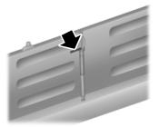
5. Make sure the latch rod is inserted into the tailgate hole and the locking pins on both sides are engaged into their holes in the pick-up box.
