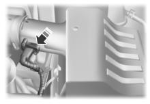
1. Locate the mass air flow sensor electrical connector on the air outlet tube. This connector will need to be unplugged.
