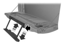
4. Rotate the center molding to unlatch the tailgate step and pull it toward you to extend it.
