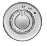
**2H (2WD)** - For general on-road driving. Sends power to the rear wheels only and should be used for street and highway driving. Provides optimal smoothness and fuel economy at high speeds.
