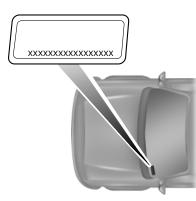
The vehicle identification number is located on the driver side instrument panel.
