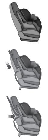
1. Position the child safety seat in a seat with a combination lap and shoulder belt.
