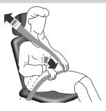
Pregnant women should always wear their safety belts. The lap belt portion of a combination lap and shoulder belt should be positioned low across the hips below the belly and worn as tight as comfort will allow. The shoulder belt should be positioned to cross the middle of the shoulder and the center of the chest.
