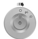
• Rotate the headlamp control clockwise to the first position to turn on the parking lamps.
