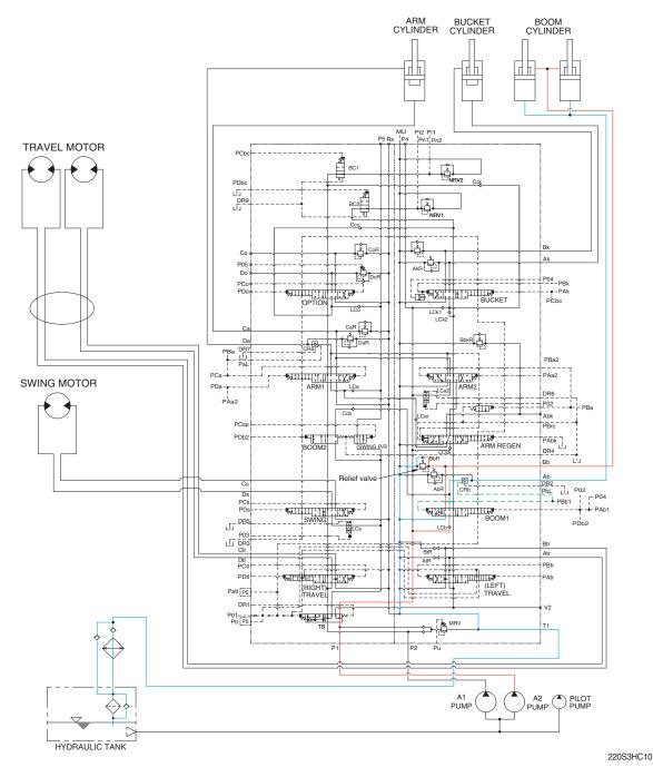
When the right control lever is pushed forward, the boom 1 spool in the main control valve is moved to the down position by the pilot oil pressure from the remote control valve.
