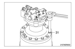
(4) Tighten 3 M16 eye bolts to the ring gear(11) and then lift the ring gear(11) out of the casing(1).
