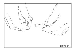
(15) Remove O-ring(13) and seal(12) from plug(11).
