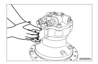
(5) Remove the relief valve(051) from valve casing(303).
