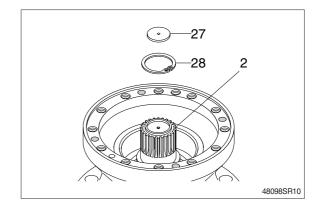
(12) Remove drive shaft (2) with roller bearing(5) and oil seal (4) assembled.Remove knock pin (26) from the casing (1).
