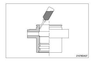
② Coat dust wiper(9) with grease and fit dust wiper(9) to the bottom of the hole of dust seal.
