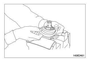
(15) Fit boot(25) and lock nut(20), and handle subassembly is assembled completely.
