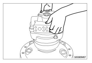
(8) Remove the brake spring(712) from brake piston(702).
