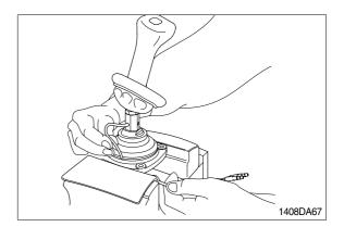
(18) Determine handle direction, tighten lock nut(20) to specified torque to fix handle.
