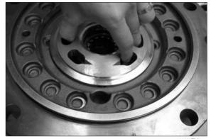
(17) Assemble O-ring (26) (WG51) to rear flange (1) sub-assembly.
