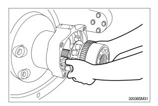
(11) Place the casing(301) under the front cover(304) and reassemble 3 sheets of separate plate(743) and then 2 sheets of friction plate(742) to the casing(301).
