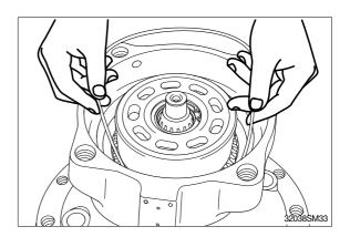
(13) Reassemble brake piston(702) to the casing(301).
