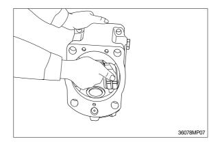
(13) Tapping lightly shaft ends of drive shafts(111, 113) with plastic hammer, take out drive shafts from swash plate supports.
