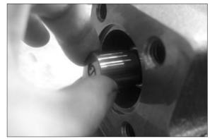
(9) Assemble washer (7) into rear flange (1).
