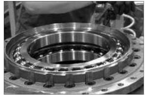
(16) Assemble hub (102) and ring gear (114) assy to spindle (101).
