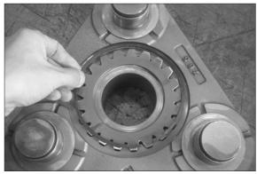
(4) Assemble planetary gear 1 (141) and side plate (144).
