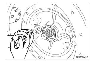
(13) Remove drive shaft(101) from casing (301).
