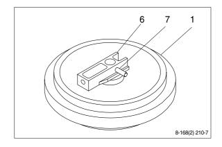
(8) Lay bracket(6) on its side. Supply engine oil to the specified level, and tighten plug.
