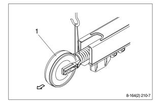
(3) Remove the bolts(2), washers(3) and separate ilder from recoil spring.
