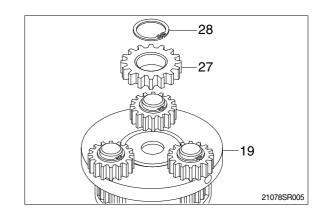
(6) Tighten two M10 eye bolts to carrier1(19) and lift up and remove carrier1(19) as subassembly.
