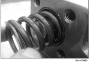
(12) Assemble counter balance spool (2), washer (7), main spring (6), seat (8) in the order named.
