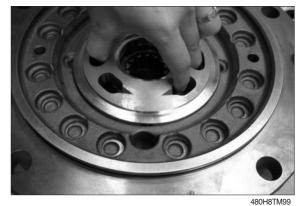
(21) Assemble cylinder spring (214, 9EA) to cylinder block (204).
