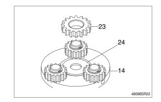
(9) Assemble carrier 1 (14) assembly onto the carrier2 assembly.
