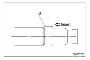
5 Fit piston assembly to rod assembly.
