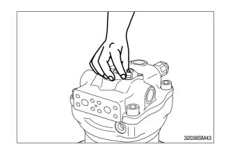
(21) Connect the valve casing(303) with the casing(301).
