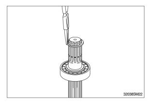
(3) Insert the drive shaft(101) into the casing (301) with the end of output shaft upward and tap the outer race of roller bearing with the hammer.
