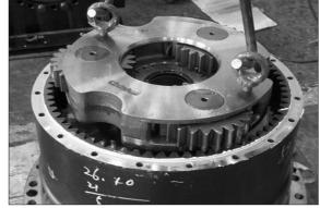
(22) Assemble carrier 1 sub assembly to ring gear (114).Assemble thrust ring 90 (151).
