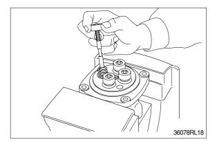
(5) Assemble O-ring(13) onto plug(11).
