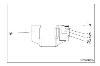
(5) Assemble carrier2(9) assembly correctly to the drive shaft(2).
