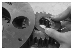
(14) Remove thrust ring (151) from sun gear(150), than remove clip (152) and remove carrier 2 (130) from sun gear 3 (150).
