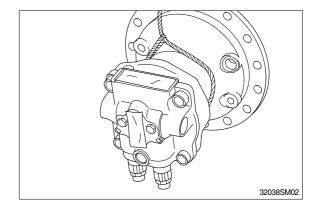
(3) Fix the drive shaft(101) on the workbench with the end of output shaft down. Put matching marks on casing (301) and valve casing(303) for easy reassembly.
