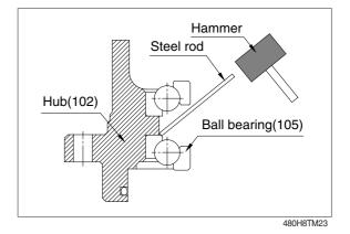
(24) As show right figure, remove remained angular bearing (105) from hub (102).
