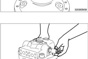
(20) Tighten the plug(468) to valve casing(303) with O-ring(487) and tighten the plug(464) to casing(301) with O-ring(485).
