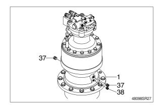
(16) Turn the swing motor assembly upside down and assemble cover plate (31) by tightening the hexagon bolts (32).
