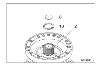
(12) Remove drive shaft(2) with roller bearing(7) and oil seal(6) assembled.Remove knock pin(12) from the casing(1).
