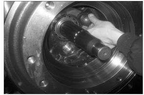
(29) Assemble two speed piston (261), shoe (262) assy.
