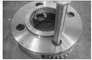
(18) Remove planetary gear 4 (121), needle bearing (122), floating bush (123), thrust washer (126) from carrier 3.
