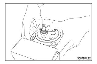
(9) When return spring is strong in force, assemble 4 sets at the same time, utilizing plate(15), and tighten joint(17) temporarily.
