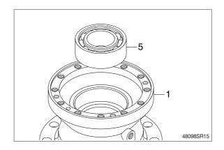
(2) Assemble the drive shaft (2) into the casing (1) and then install oil seal (4) and roller bearing (5).
