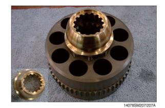
③ Disassemble spring (11) from cylinder block (10).
