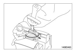
(4) Loosen lock nut(20) and adjusting nut(19) with spanners on them respectively, and take out handle section as one body.
