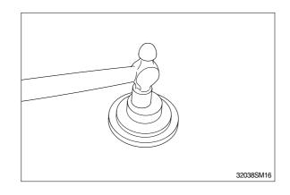
③ Remove the roller bearing(444) from the valve casing(303) by using slide hammer bearing puller.
