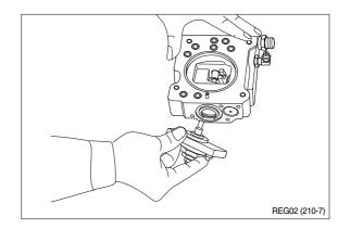
(5) After removing cover(C, 629) subassembly, take out outer spring(625), inner spring (626) and spring seat(C, 624) from compensating section.
