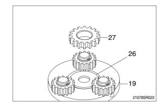
(9) Assemble carrier1(19) assembly onto the carrier2(9) assembly.
