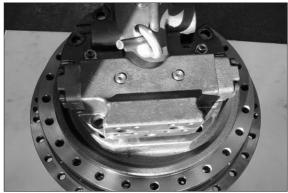
(6) Remove socket bolt (M10 $\times$ 135) then remove parking piston (212) and spring (213).
