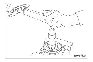
(12) Assemble swash plate(18) to joint(17).
