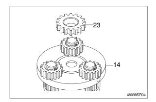
(6) Tighten two M10 eye bolts to carrier1 (14) and lift up and remove carrier1 (14) as subassembly.
