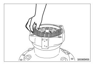
(15) When assembling the roller bearing(444), insert the roller bearing(444) into valve casing(303) by hammering.
