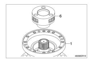
(6) Assemble sun gear2 (22) to the center of the carrier2 (6) assembly.
