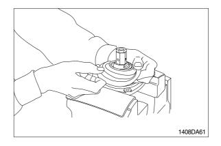
(6) Loosen adjusting nut(19) and plate(18)with spanners on them respectively, and remove them.
