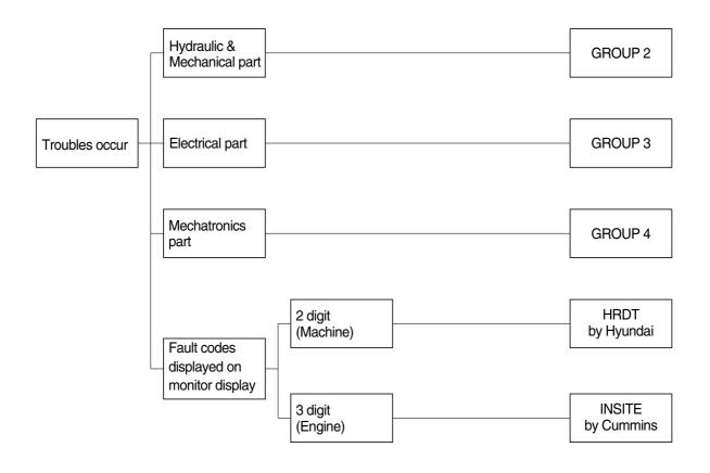
\* If fault codes (2 or 3 digits) are displayed on the monitor, please contact Hyundai or Cummins.
