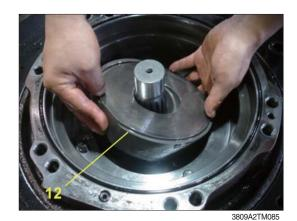
(9) Assemble swash piston kit assembly.
