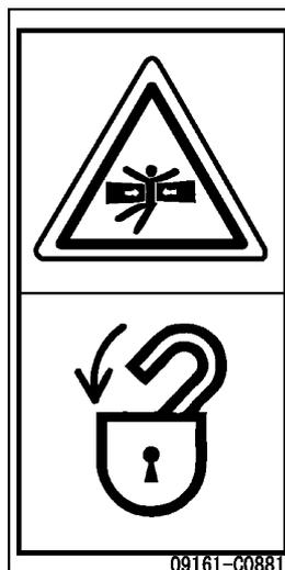
Sign indicates a crush hazard between the articulating parts of vehicle.
