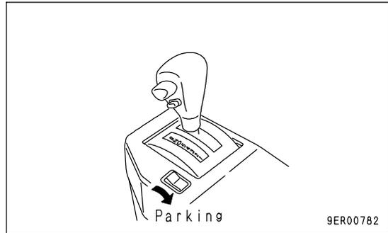
2. Check that gear shift lever (2) is at the N position.
