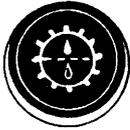
This lamp lights up when the torque converter or transmission filter elements are clogged.
