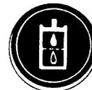
This lamp lights up to warn of a clogged element in the hydraulic oil filter.
