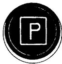
This pilot lamp lights up when the parking brake is applied by operation of the parking brake valve lever.
