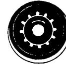
This pilot lamp lights up when the retarder brake is on.
