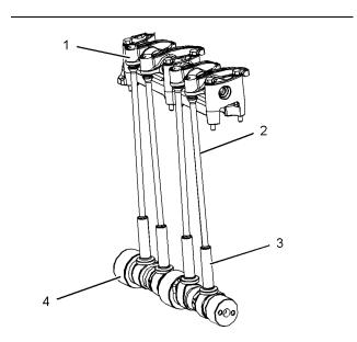
Illustration 14 Valve system components (1) Rocker arm
