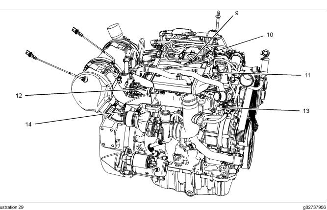
A typical example of sensors and electrical connector locations on the right side of the 854E-E34TA (model JR) and 854F-E34TA (model JV) engines
