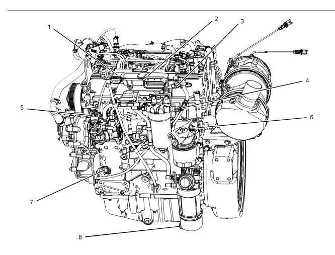
Sensors and electrical connector locations on the left side of the engine
