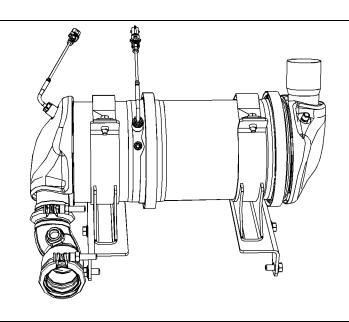
A typical example of a CEM with a wall flow Diesel Particulate Filter (DPF)
