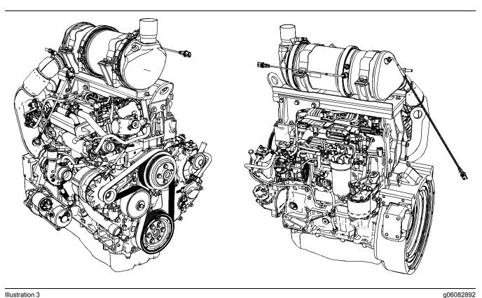
Typical example of an engine with top mounted aftertreatment
