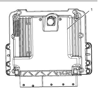
Illustration 33 Typical example The Electronic Control Module (ECM) (1) functions as a governor and a computer for the fuel system. The ECM receives signals from the sensors to control the timing and the engine speed.
