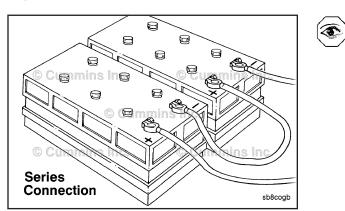
This illustration shows a typical series battery connection. This arrangement, positive (+) to negative (-), doubles the voltage.
