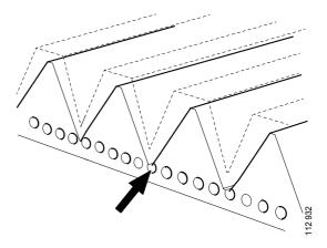
The belt is worn down to the cord. The drive belt must be renewed.
