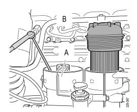
8. Move the suction tool to the pressure filter housing (B). Draw out remaining fuel and particles.
