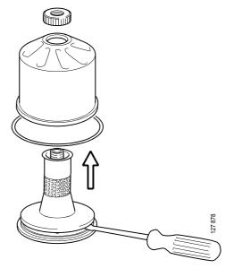
7. Remove the paper insert and scrape away any remaining dirt deposits inside the rotor cover. If the deposits are thicker than 28 mm, the centrifugal oil cleaner must be cleaned more often.
