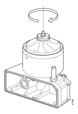
18. Renew the O-ring on the cover of the oil cleaner housing and fit the cover. Tighten the lock nut to 15 Nm.
