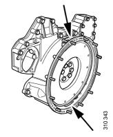
Openings for taking readings on the flywheel housing.
