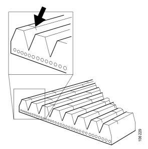
The drive belt must be renewed if it has cracks.
