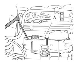
5. Make a mark on the pressure filter cover (B). Unscrew the cover 3 to 4 turns using a socket wrench with hexagon driver, e.g. 588 475. Draw out fuel which may drain into the water separating suction filter housing when the pressure filter is detached.
