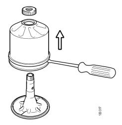
6. Remove the strainer from the rotor cover. If the strainer is stuck, insert a screwdriver between the rotor cover and strainer and carefully prise them apart.
