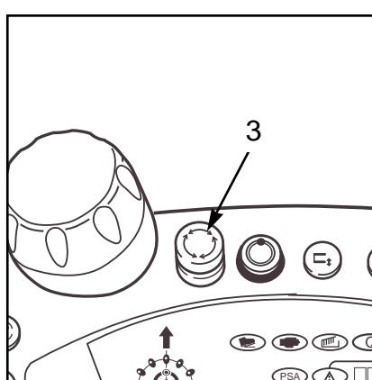
Unlock emergency shut-off switch (3) by turning it.
