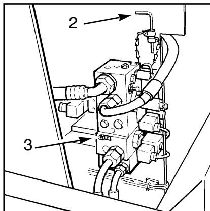
Emergency lowering of the driver's cab, leaving the cab in an emergency situation.
