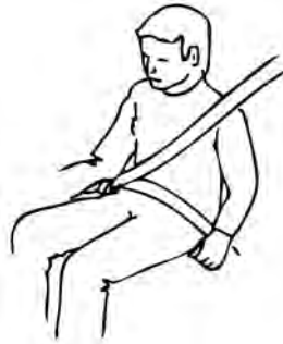
Incorrect (too high on hips)
