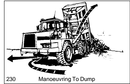
230 Manoeuvring To Dump
