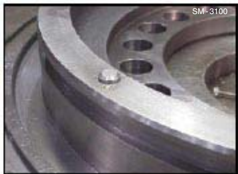
Fig. 13 - Pin at Proper Depth
