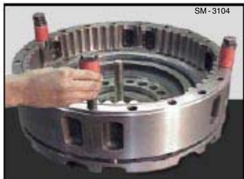
Fig. 17 - Installing Three Capscrews
