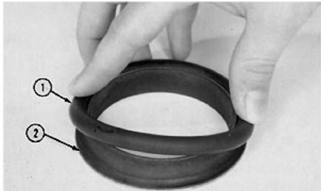
1—Rubber Seal 2—Metal Seal Ring
