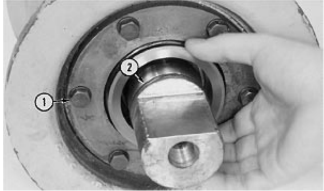
1—Cap Screw (12 used) 2—O-Rings
