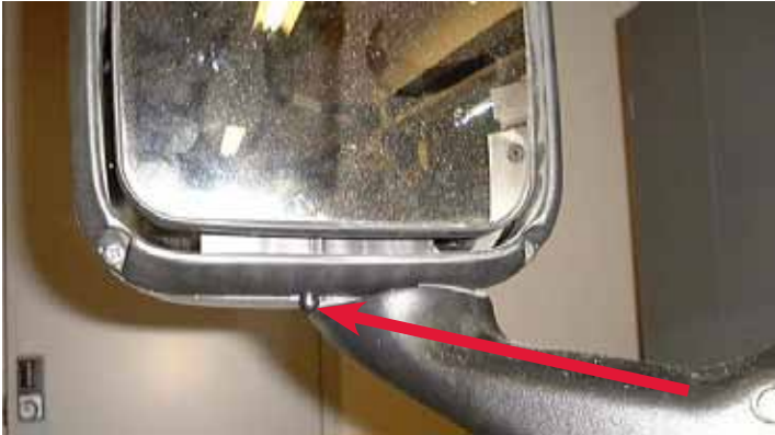
FIGURE 2-4: Aerodynamic Mirror OAT Sensor Location
