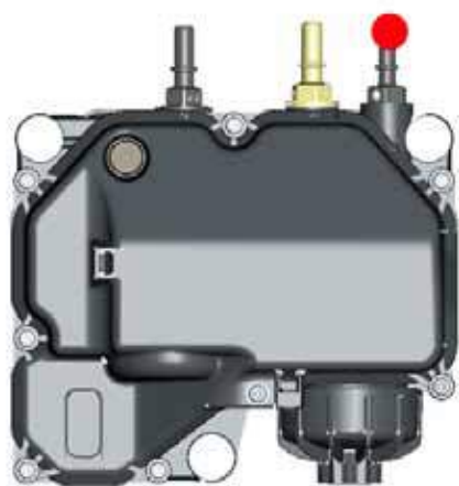
FIGURE 4-1: Measurement Location of DEF Supply Module (Pump)
