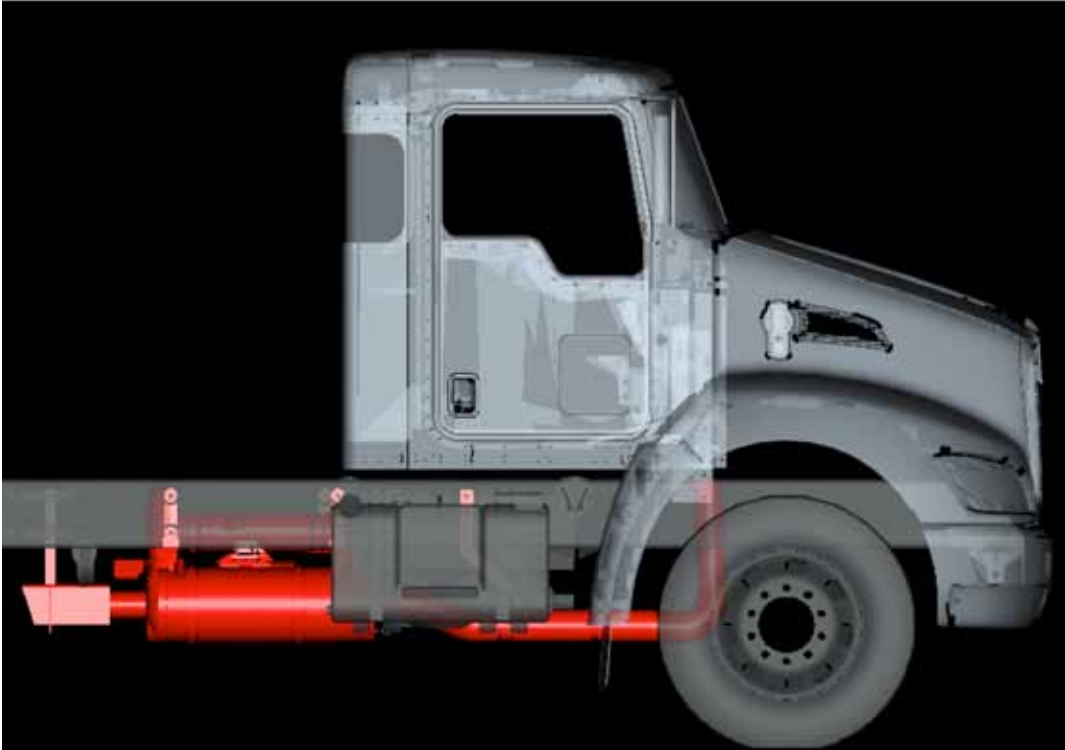
FIGURE 4-15: Right view of Horizontal DPF and SCR with Horizontal Tailpipe
