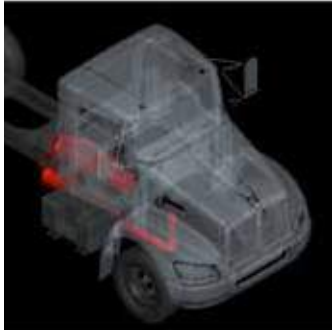
Horizontal DPF and SCR with Horizontal Tailpipe
