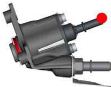
FIGURE 4-2: Measurement Location of DEF Dosing Module (Injector)
