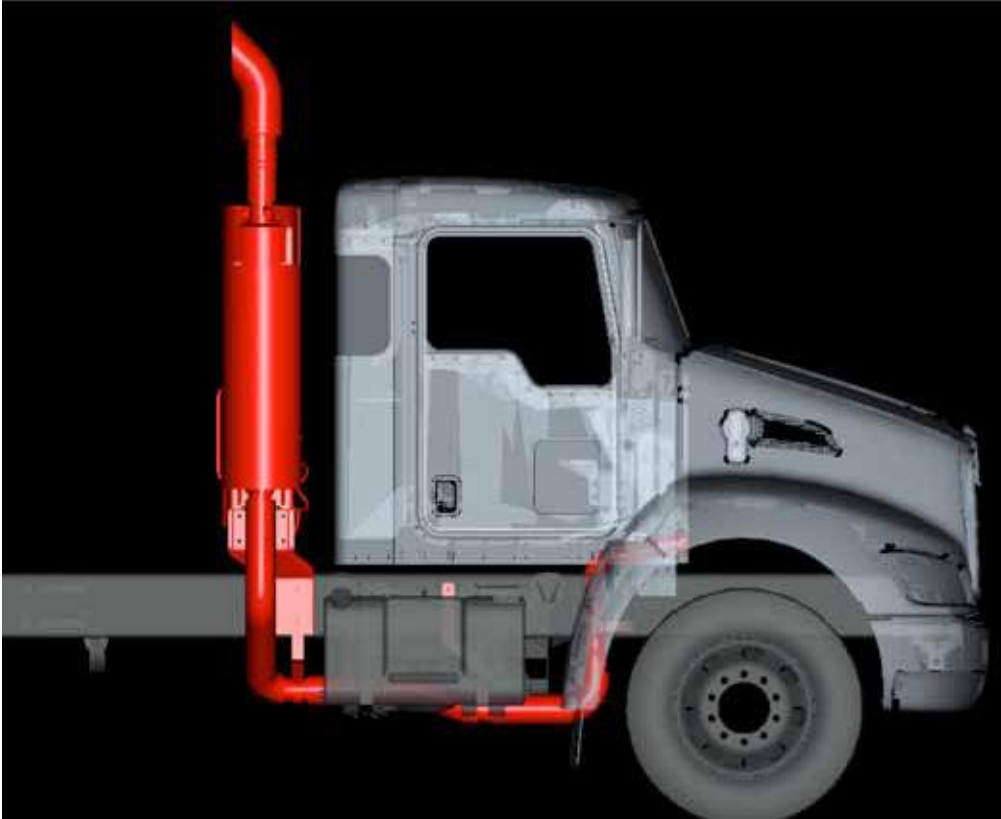
FIGURE 4-23: Right view of Vertical Independent DPF and SCR
