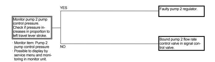
A-4 Right travel is inoperable during single travel operation. Single bucket operation speed becomes slow. Boom is not raised properly during arm level crowding. (All problems occur at the same time.)
