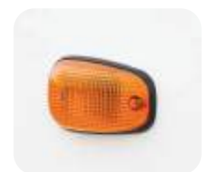
Side Marker Lamp Warns other drivers of truck getting closer
