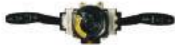
Combination Switch Turn Signal Lamp, Windshield Wiper, Exhaust Break, Hazard warning flasher
