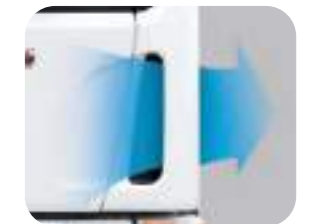
Large Corner Vane Reducing wind noise inside the cabin
