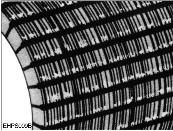
Marks on the Commutator Surface
