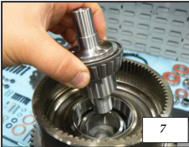
Thread 34-218 Stub Shaft with 101-76 Bearing Cone into the 34-216 Output Shaft . Photo 7. Torque to 100 ft lbs. Photo 8.
