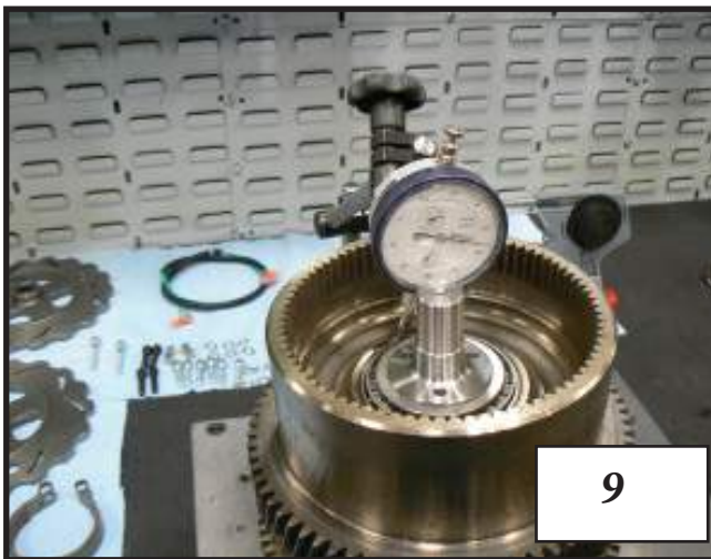
Check endplay with dial indicator (.0005 to .0025) Photo 9. If endplay is not enough, use required shim size.
