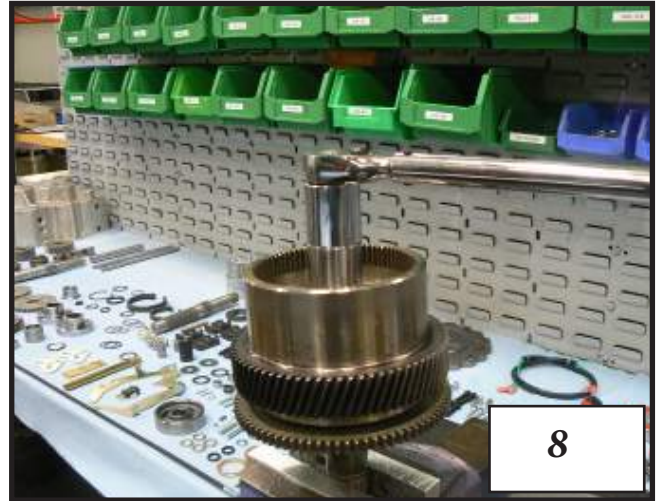
Thread 34-218 Stub Shaft with 101-76 Bearing Cone into the 34-216 Output Shaft . Photo 7. Torque to 100 ft lbs. Photo 8.
