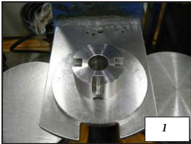
Position Output Shaft on special fixture on press. Photo 1 & 2.
