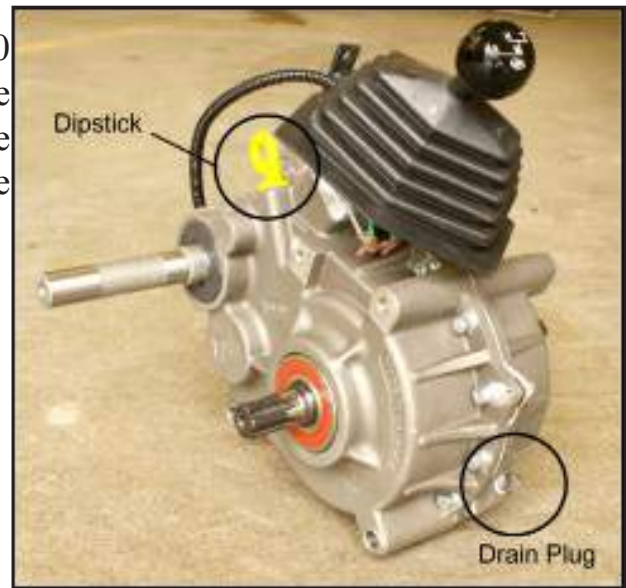
Figure 6-4a. 34-100 Transmission showing dipstick and drain plug locations
