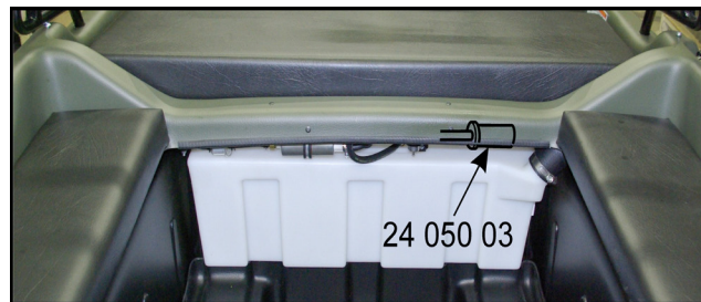
Figure 6-6. HDi and Avenger EFI fuel filter location.
