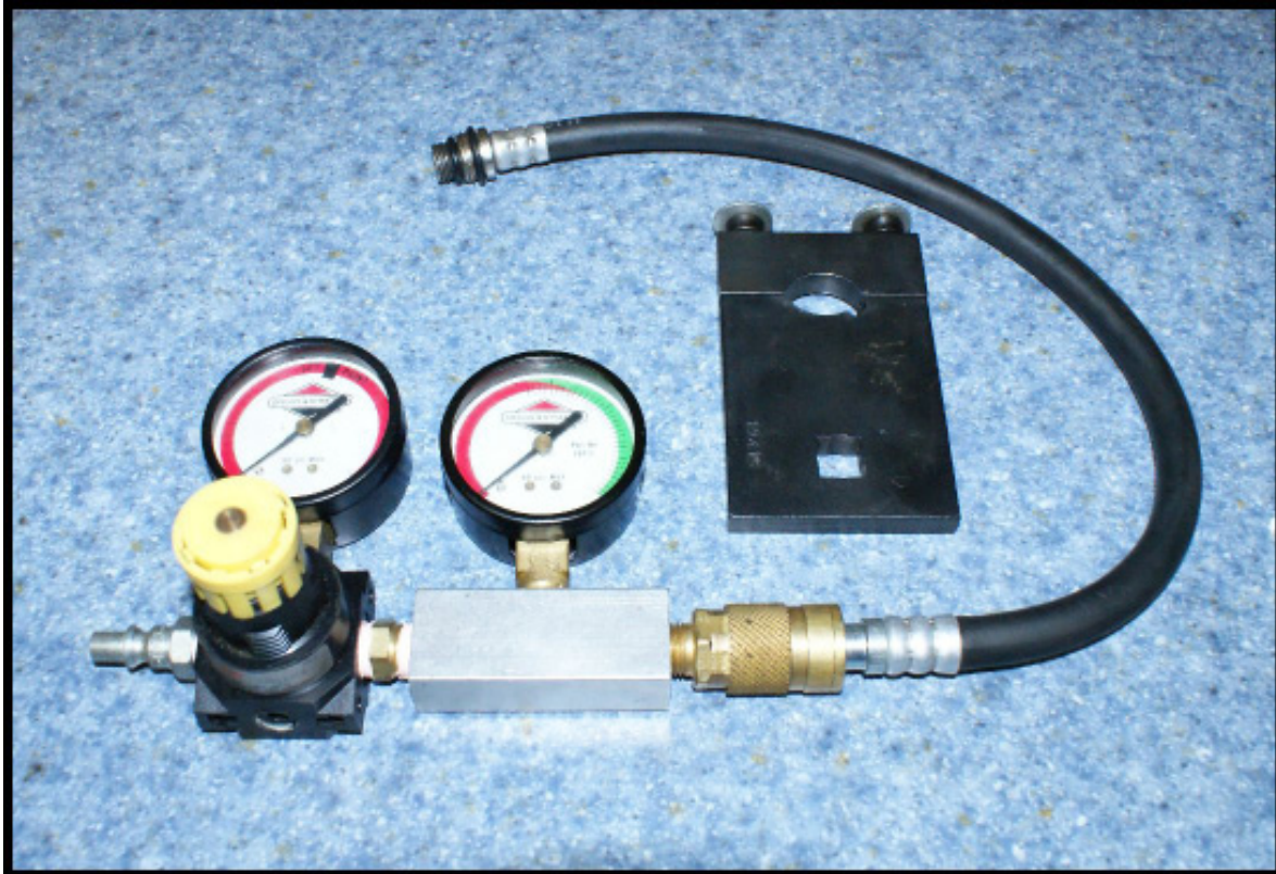
Leak down tester- Briggs & Stratton Part No. 19545 (can be used for all small engines)
