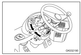
3. Pull parking brake lever (4) and set it to the LOCK position.
