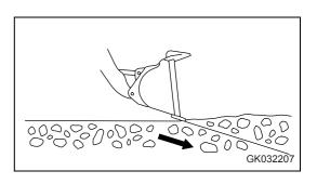
2. Drive the machine forward and operate the work equipment control lever forward to cut a thin layer of the surface each time when excavating the soil.
