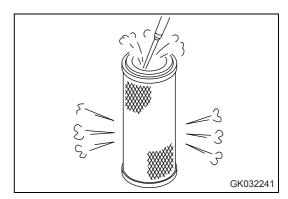
8. If small holes or thinner parts are found on the element when it is checked by shining a light through it after cleaning, replace the element.
