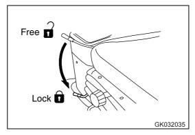
3. Stop the engine, check that the area around the operator's compartment is safe, then lock with the safety bar so that the front frame and rear frame do not articulate.
