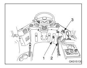
1. Depress accelerator pedal (1) lightly and run the engine with no load at midrange speed for about 5 minutes.
