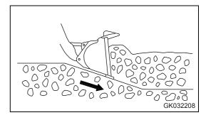
Operate the work equipment control lever slightly up and down to reduce the resistance when driving the machine forward.
