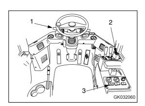
3. Place the directional selector switch actuation switch (3) at the ON position (a).
