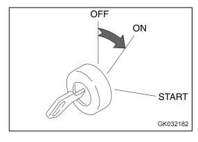
2. Check that all the monitors, gauges, and the central warning lamp light up for approx. 3 seconds and the alarm buzzer sounds for approx. 1 sec.
