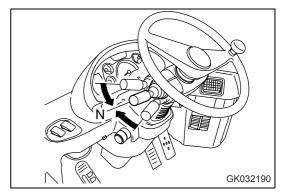
3. Pull parking brake lever (4) and set it to the LOCK position to apply the parking brake.
