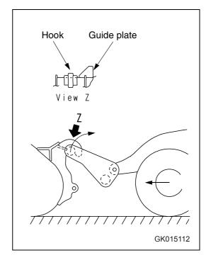
7. Operate the control lever for the coupler (2) backwards, to insent lock pins and lock the attachment in position.
