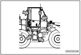
To ensure safety, always face the machine and maintain three-point contact (both feet and one hand, or both hands and one foot) with the handrails and steps to ensure that you support yourself.
