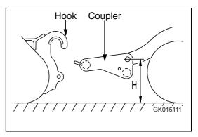
5. Drive the machine slowly forward until the guide plate enters the inside of the hook of the attachment.
