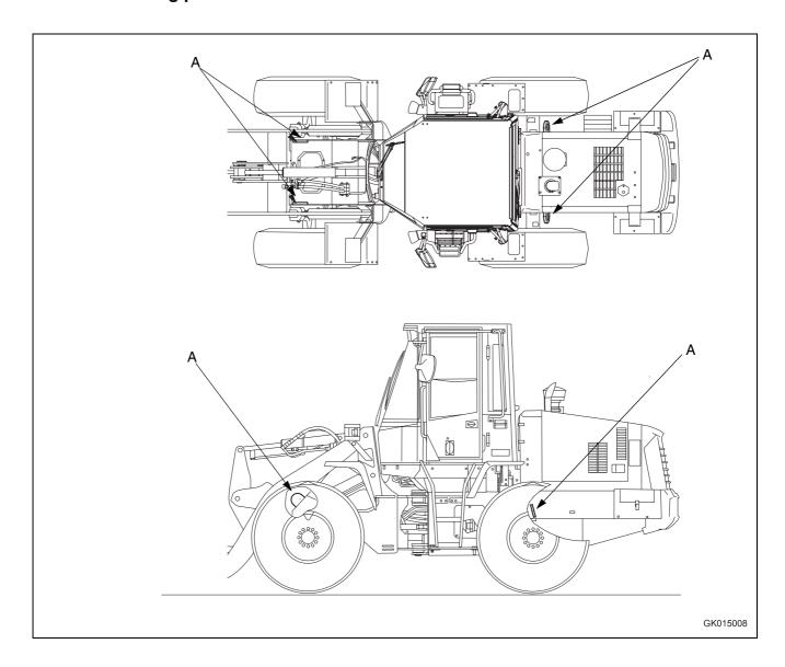
Lifting hooks (A) are located at 4 places on the machine as shown in the diagram on the right.
