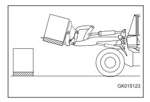
6. Lower the load until it is close to the ground surface (30 inches from the ground surface).
