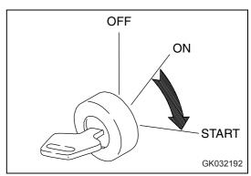
4. After the engine starts, release the key in starting switch (1). The key will automatically return to the ON position.
