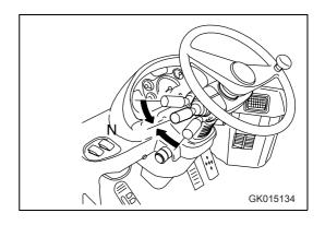
2. Place the directional selector switch (2) at the N position.
