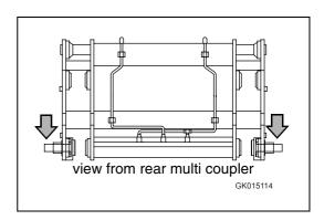
9. The protrusion (X) on left and right side should be 30mm.
