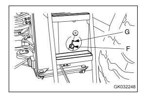
4. The oil level should be between the H and L marks on dipstick (G).
