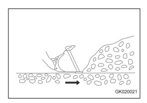
Thrust the bucket fully into the soil, then drive the machine forward and operate the work equipment control lever to raise the lift arm. In addition, operate the work equipment control lever occasionally to tilt the bucket so that the bucket can be fully loaded.
