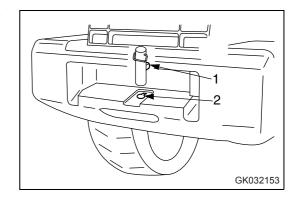
2. To prevent the towing pin from turning, fold the handle of the towing pin and set it in position.
