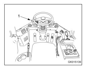
There is no need to stop the machine even when switching between FORWARD and REVERSE.
