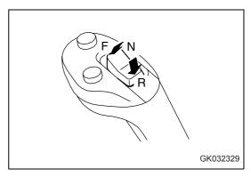
3. Place the directional selector switch actuation switch (3) at the ON position (a).
