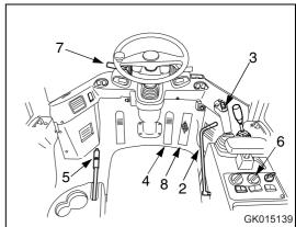
2. Check that the work equipment control lever (3) is at the HOLD position, then set safety lock lever (2) to the FREE position.
