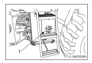
2. Remove the mud and dirt from around the breather (2), then remove breather (2).
