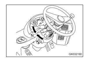
2. Place the directional selector switch (2) at the N position.
