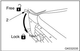
• Pull parking brake lever (3) to the LOCK position, then put blocks under the front and the rear of the tires.
