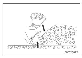
3. If it is difficult to thrust the bucket into the soil, operate the work equipment control lever to the left and right to move the cutting edge of the bucket up and down.
